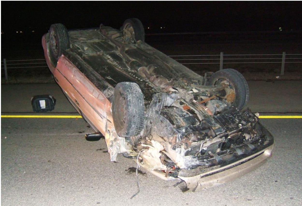
Figure 76. Example of Post Snag Rollover Crash
