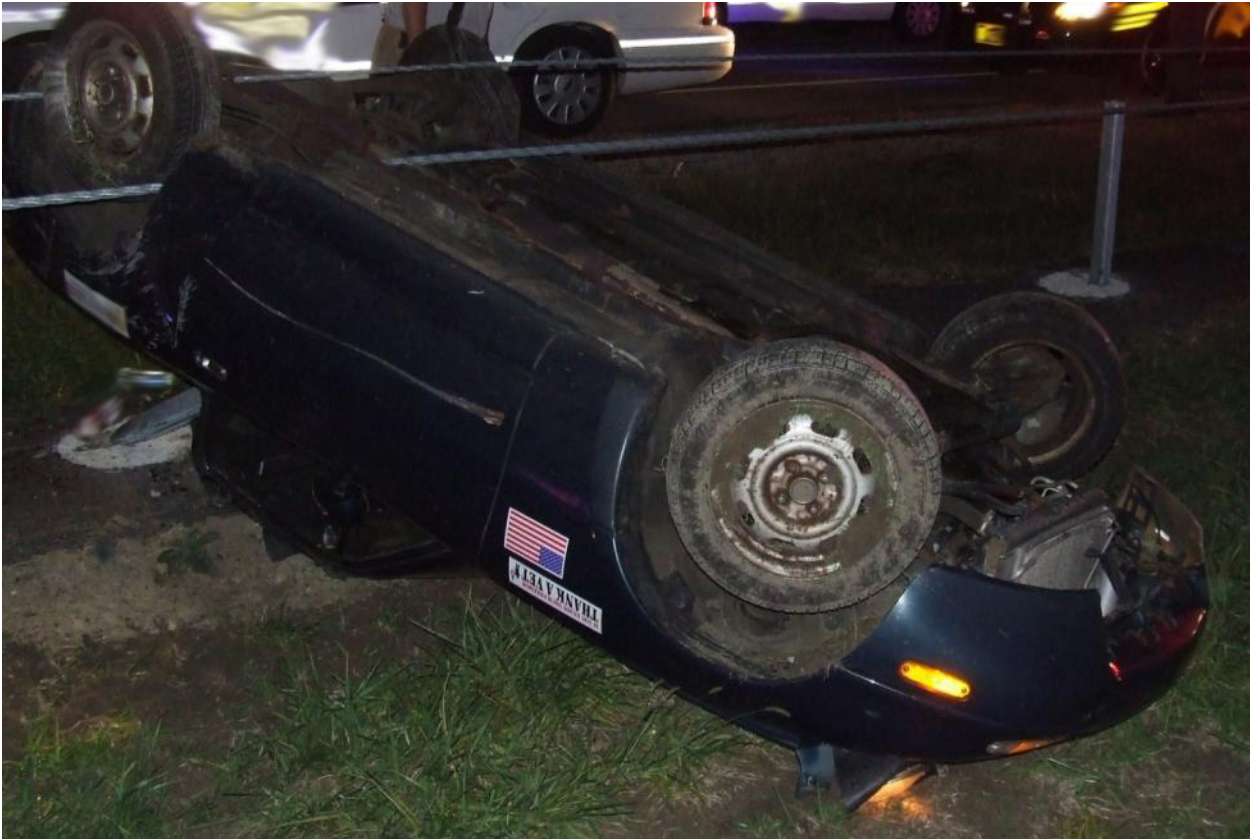
Figure 77. Example of Post Snag Rollover Crash
