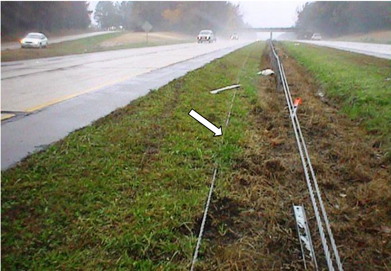
Figure 63. Middle Cable Release from Many Downstream Posts Resulting in Penetration
