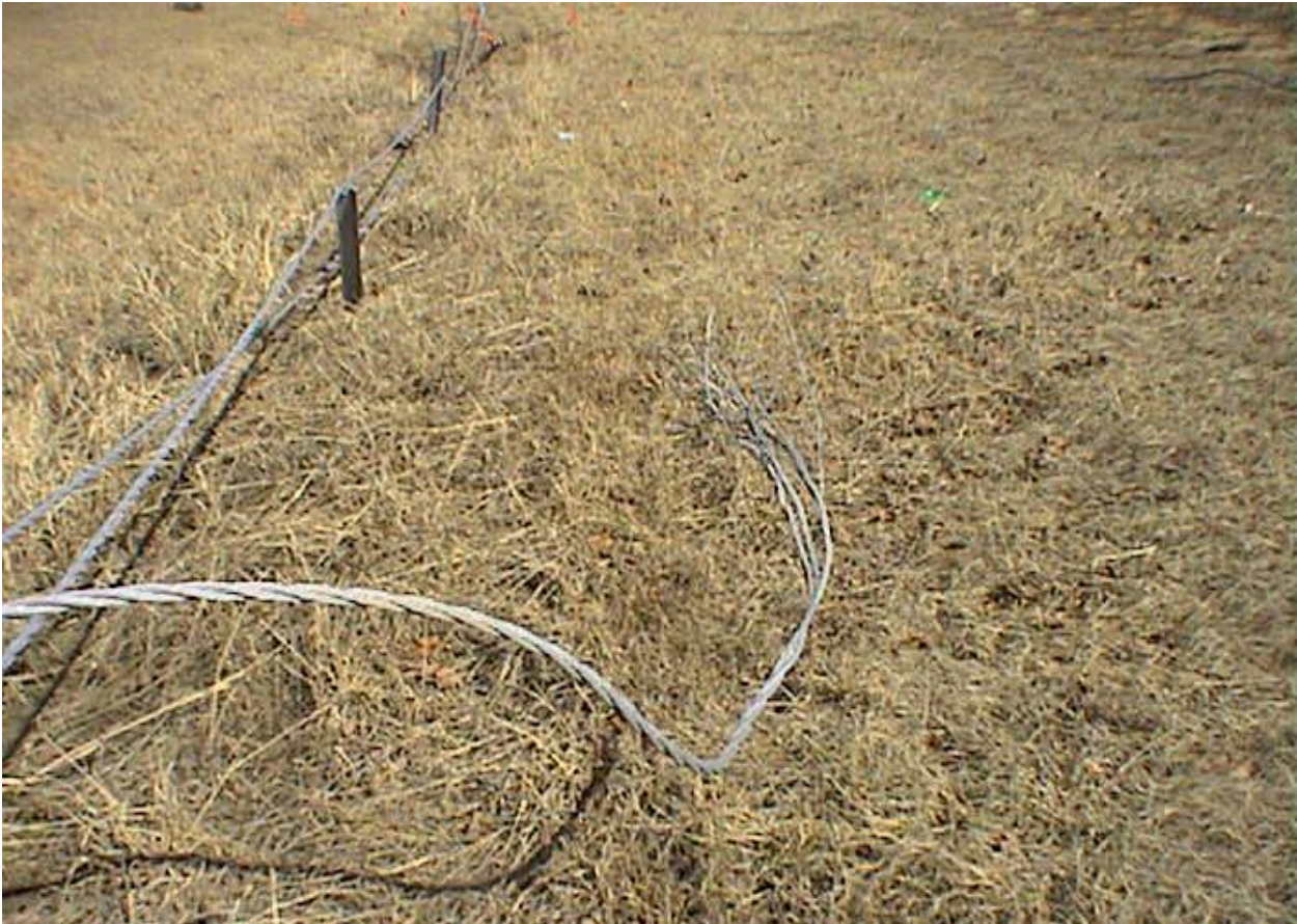
Figure 67. High-Tension Splice Tearout Penetration
