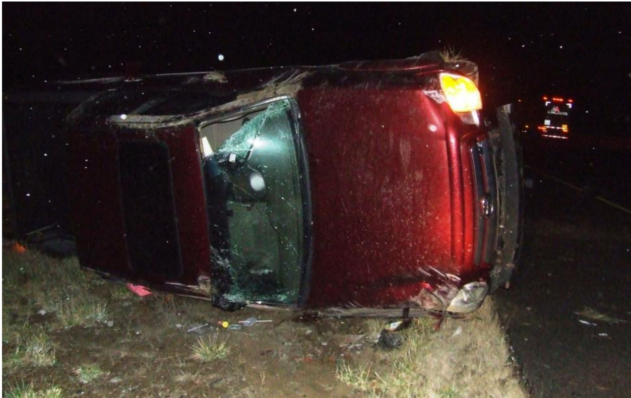
Figure 47. Crash Result Due to Strong Cable-to-Post Connection
