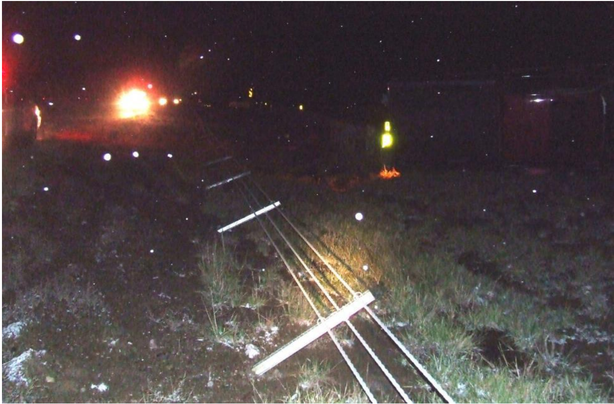
Figure 46. Penetration Crash Caused by Strong Cable-to-Post Attachment
