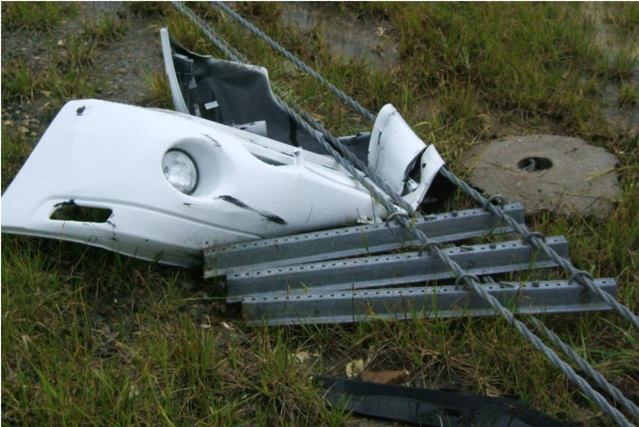
Figure 49. Override Penetration Crash Vehicle Final Position and Removed Bumper Cover
