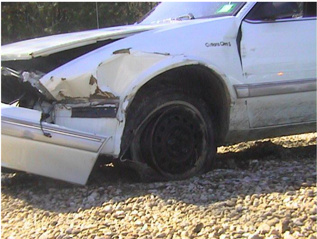
Figure 68. High-Tension Splice Tearout Penetration
