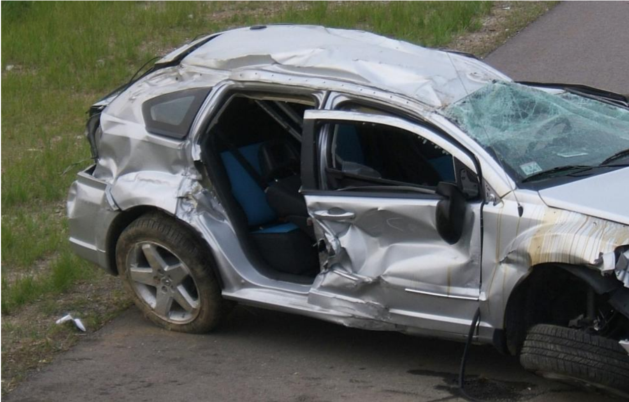
Figure 71. Example Rollover Crash Caused by Redirection on Back Slope (continued)
