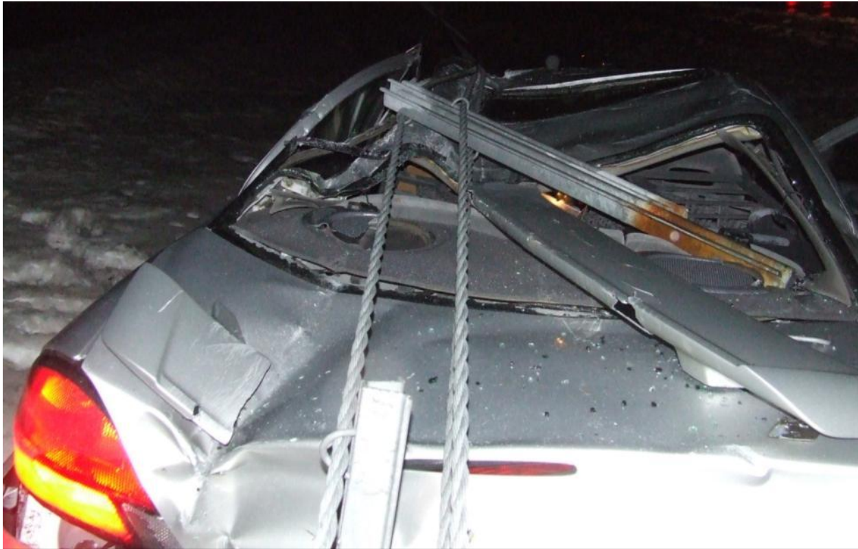
Figure 52. Potential Penetration Crash on Nucor NU-CABLE Barrier
