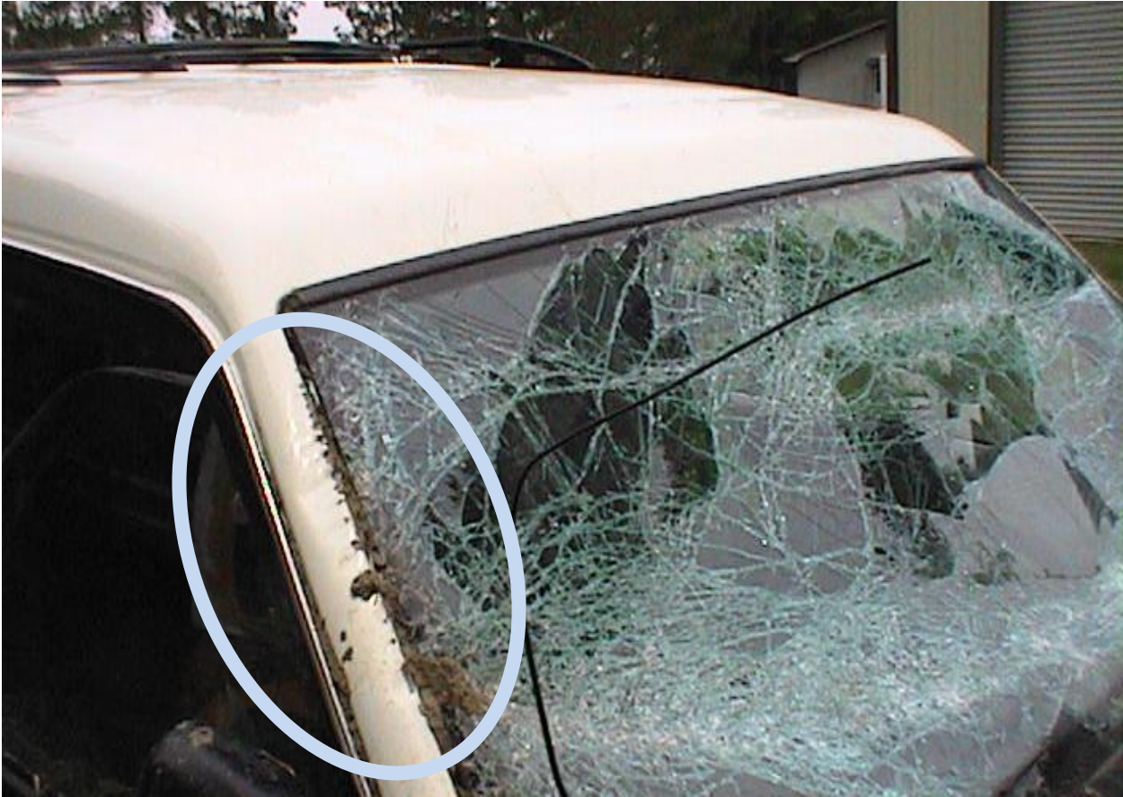
Figure 66. Brush Guard Prying Penetration with Cable Contact Striations on A-Pillar
