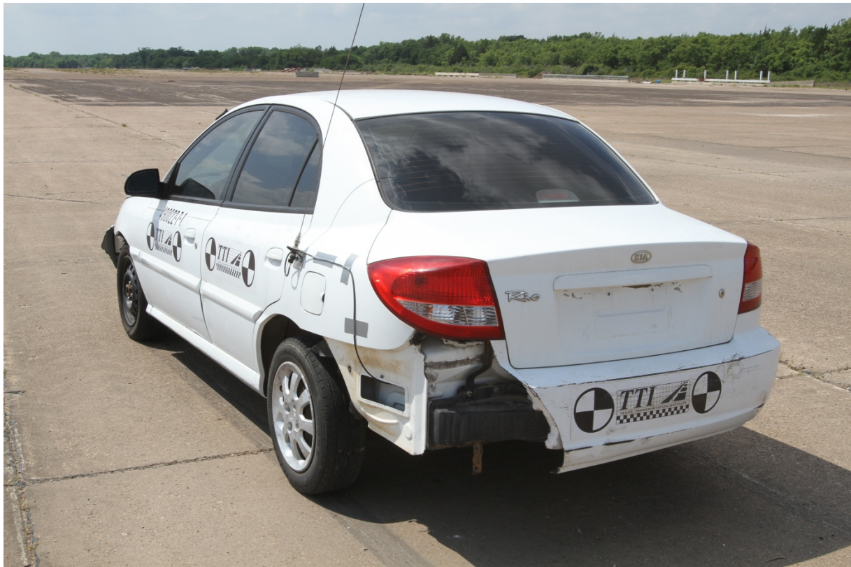
Figure 4.9. Vehicle after Test No. 490022-7-1.
