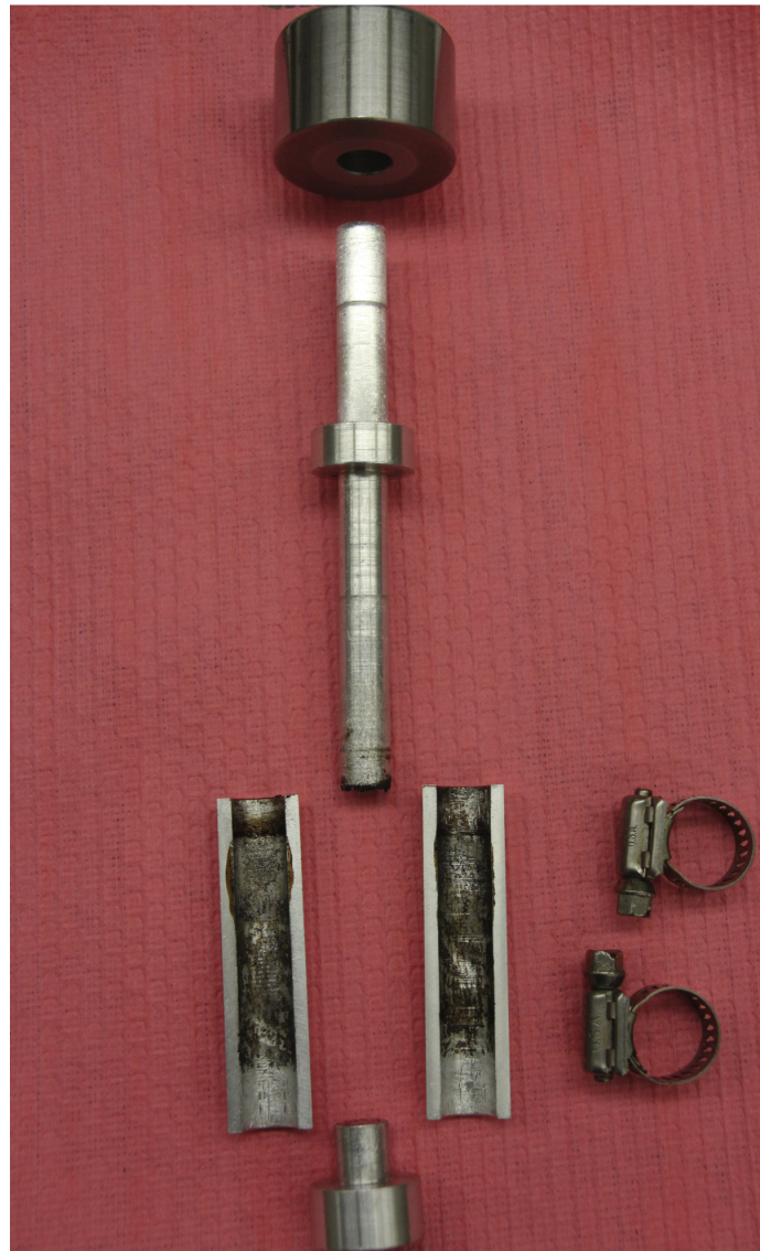
Figure 3.2. Assembly of the compaction mold
