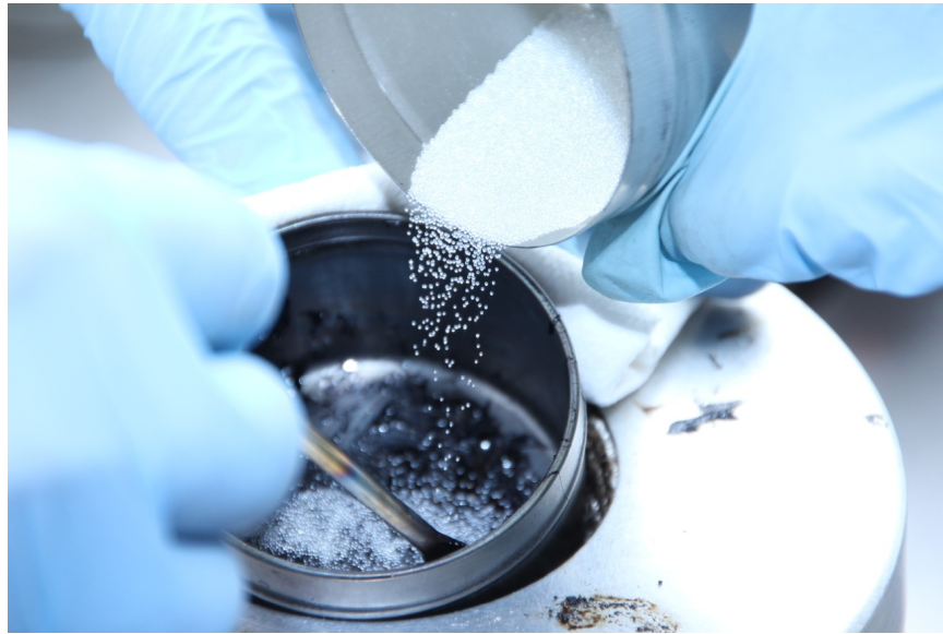
Figure 3.3. Addition of glass beads to asphalt binder in the temperature jacket
