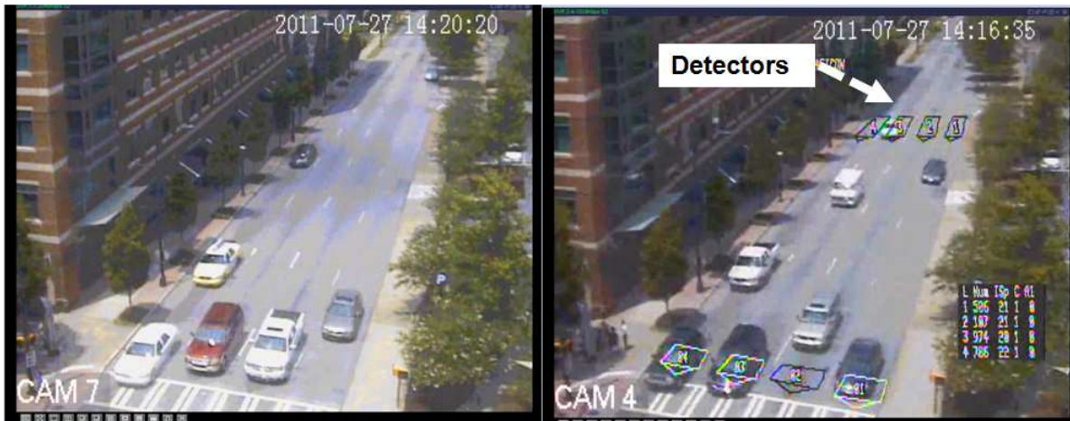
Figure 45 Midblock Detector Camera Data Acquisition View
