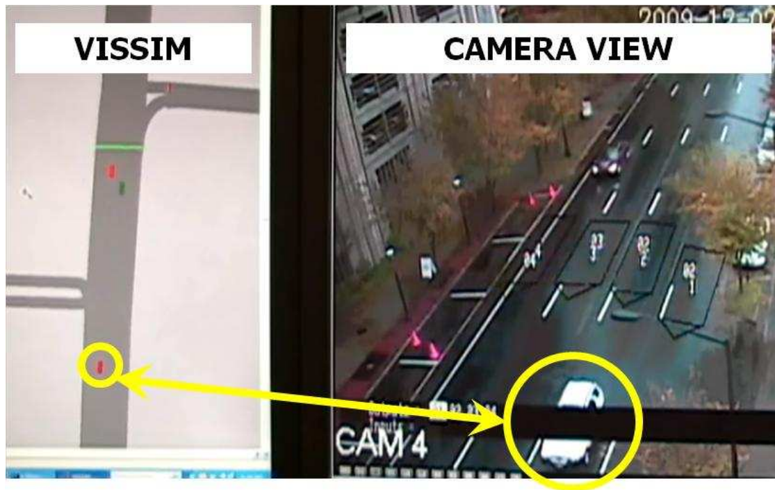
Figure 26 Permanent Detector Generating Vehicle in VISSIM in Real-Time
