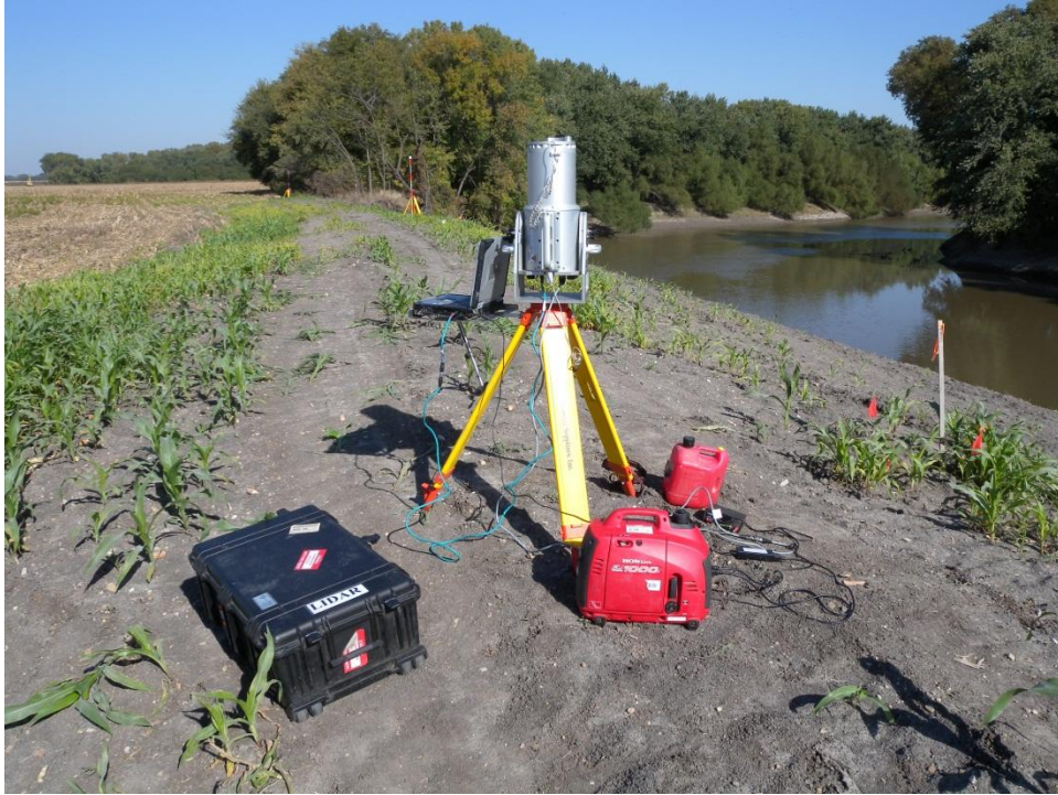
FIGURE 3.3 The Riegl System at Site 25, Including Generator and Laptop. Tiepoints Are Visible to the Right of the Scanner (on the Terrace) and in the Distance at the End of the Project
