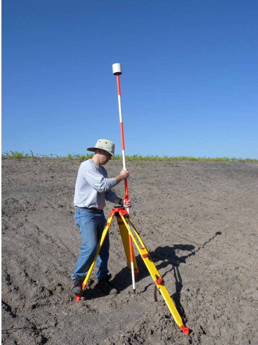
FIGURE 3.4 Leveling a 10 cm Reflective Tie Point The Photograph Shows the Tie Point Mounted on Double Range Poles. Single Range Poles Were Adequate for All Sites in This Study.
