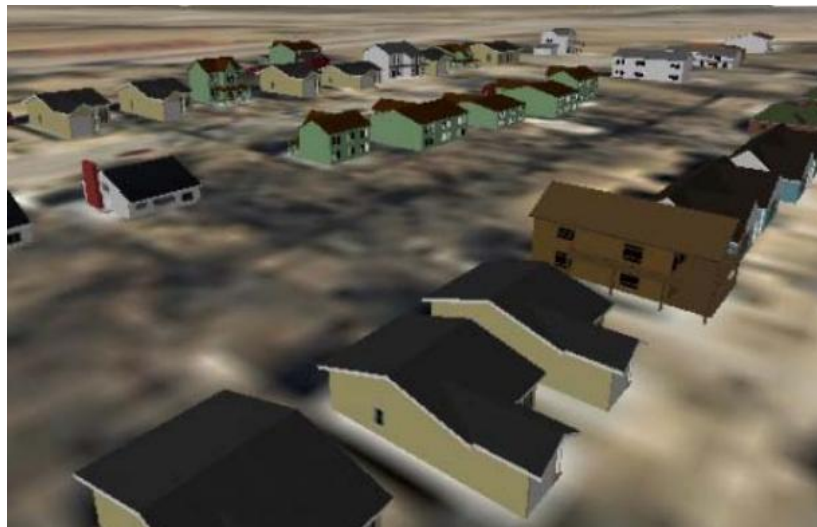
FIGURE 2.8 Development of 3D Structure Model with LiDAR Data
