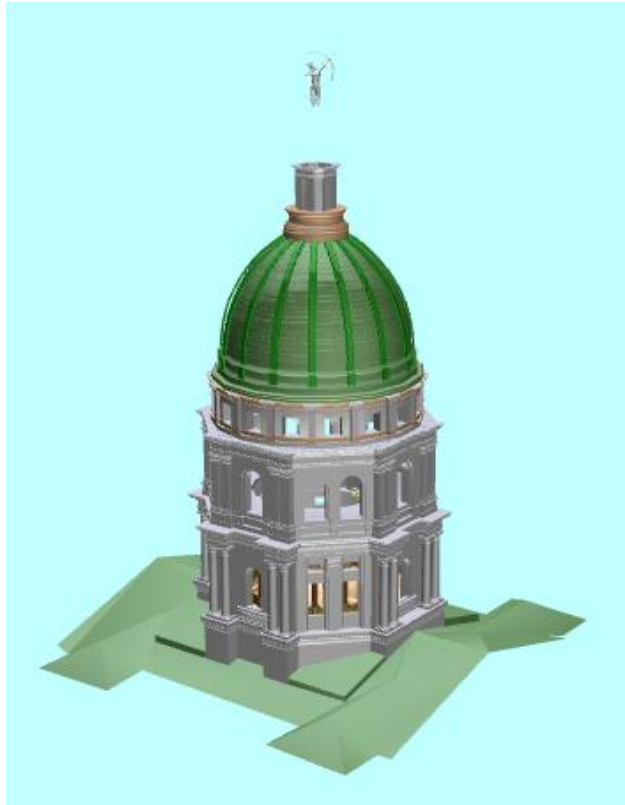
FIGURE 2.13 LiDAR-Derived CAD Model of the Kansas State Capitol Building
