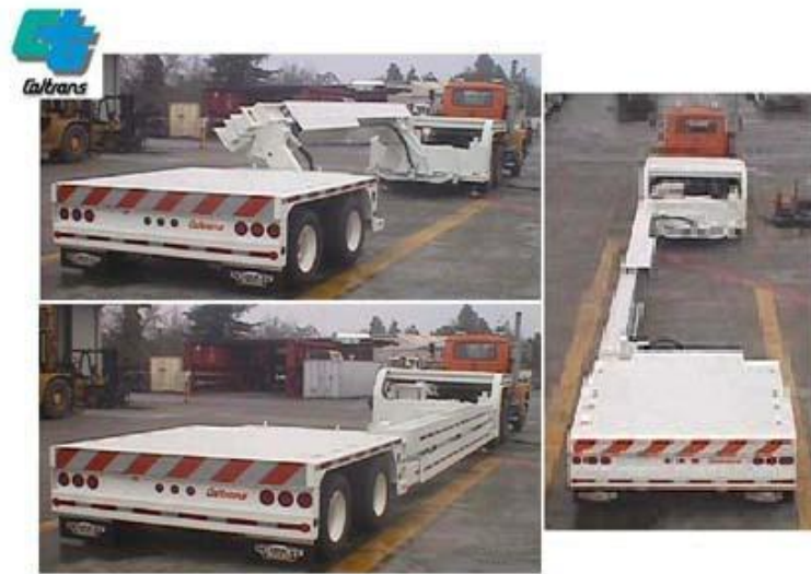
FIGURE 12 Balsi Beam Mobile Barrier System
