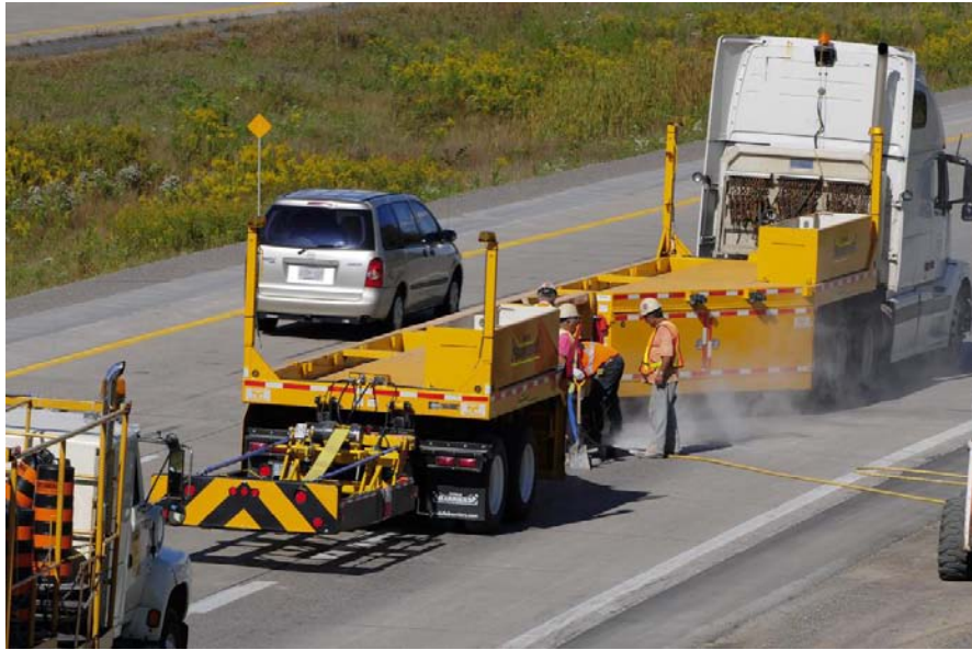
FIGURE 13 Mobile Barrier Trailer (MBT-1) System
