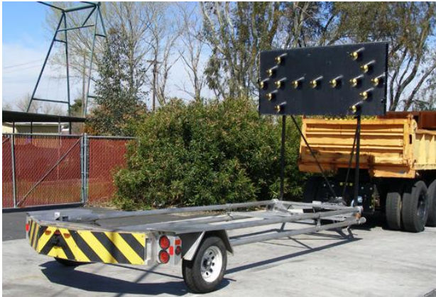
FIGURE 14 Trailer (Left) and Truck (Right) Mounted Attenuators
