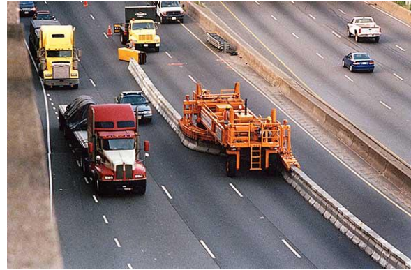
FIGURE 11 Barrier Transfer Machine on an Urban and Interstate Facility
