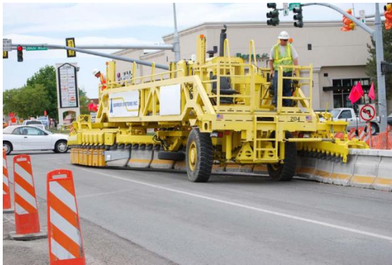
FIGURE 11 Barrier Transfer Machine on an Urban and Interstate Facility
