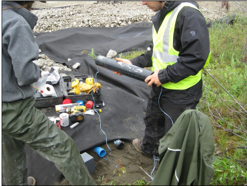
Figure C-14. Routing pull rope for SAA through ABS end cap adapter. (Photograph courtesy of J. Zottola, July 2012)
