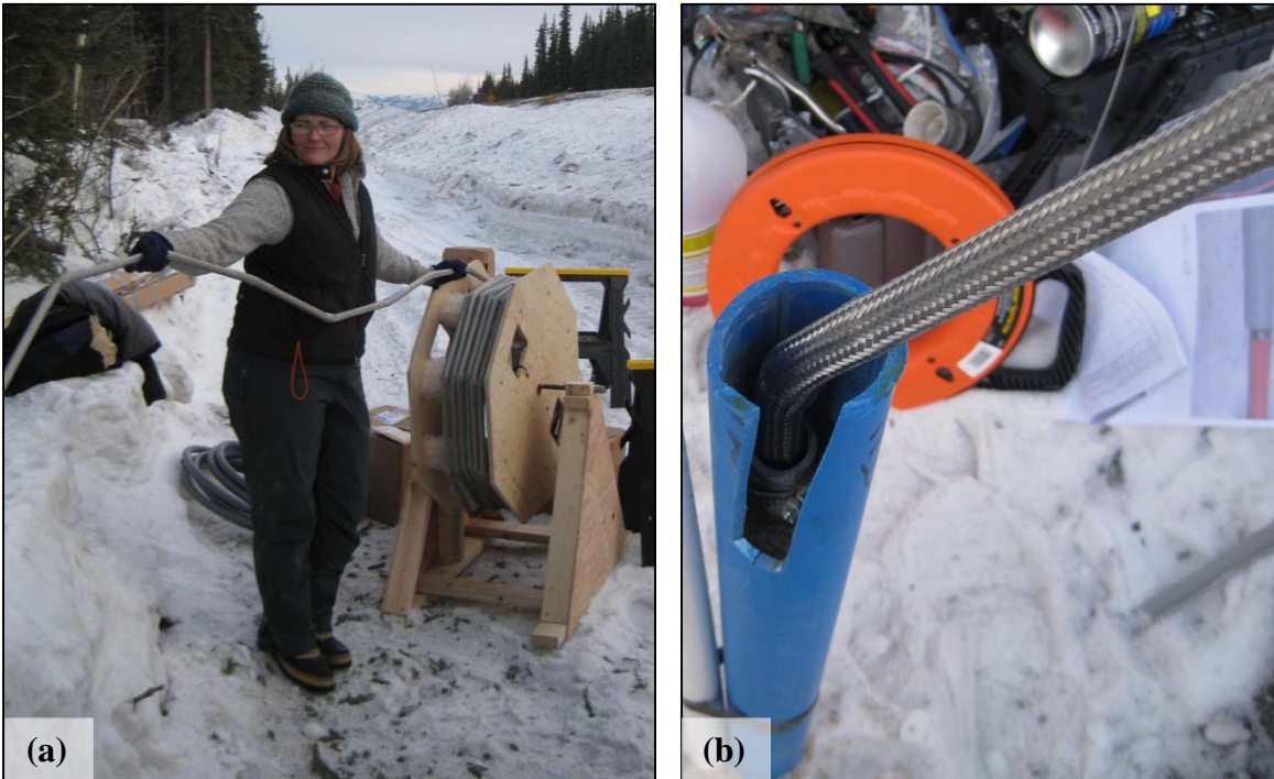
Figure A-15. Installing the SAA device. (a) Guiding the SAA off of the shipment reel, and (b) into the inner 1.05-in. PVC casing. (Photographs by M. Darrow, March 2010)
