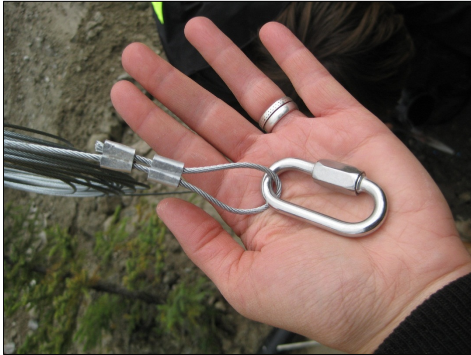
Figure C-20. Attaching 2 1/4-in. locking link to wire rope within guide casing. (Photograph by M. Darrow, July 2012)
