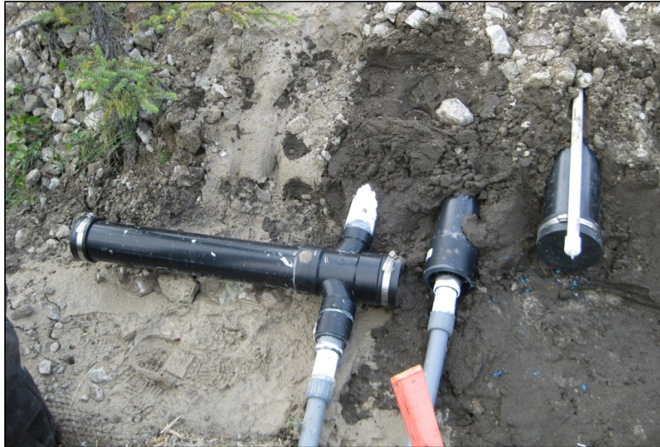
Figure C-24. Downslope casing ends secured. From left to right, ABS casing to flexible conduit adapters for TAC/thermistor cables and SAA device, and sealed guide casing for manual inclinometer probe measurements. (Photograph by M. Darrow, July 2012)
