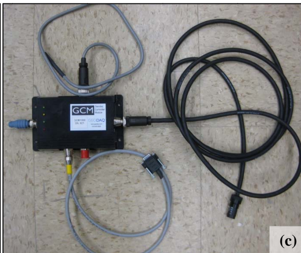
Figure 1. Components of the Geodaq INC500 device. (a) Modules prepared for installation; the yellow arrow indicates a safety line attached to the lowest module. The other components necessary to complete an installation are (b) coupler assemblies, centralizers, a slotted fork to hold the INC500 within the casing, and (c) the GCM controller module. (Photographs by M. Darrow)
