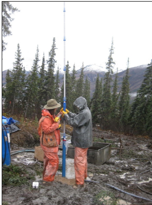
Figure D-4. Installing the INC500 within the guide casing in TH12-9004. (Photograph by J. Simpson, Sept. 2012)
