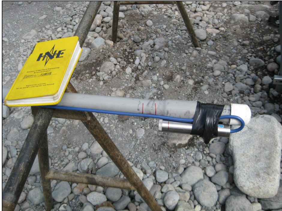
Figure B-5. Placement of vibrating wire piezometer on PVC casing for installation into TH10-1553. (Photograph by M. Darrow, June 2010)
