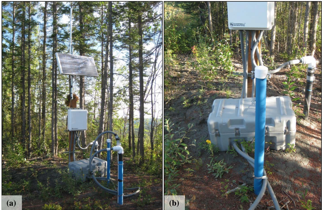
Figure A-19. Final configuration of the Rich113 site. (a) Complete ADAS overview; (b) TH07-1711 in foreground with battery box and ADAS; TH09-1511 is to the right. (Photographs by M. Darrow, Aug. 2011)
