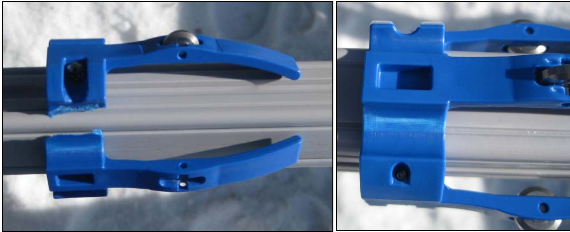
Figure A-7. Damage to centralizers due to improper alignment during the March 2010 installation. (Photographs by M. Darrow)
