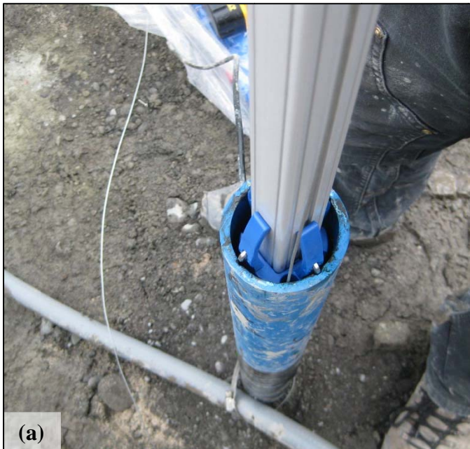
Figure B-4. Installing the INC500 within the guide casing. (a) This photograph shows the arrangement of the centralizers and the wire rope used as a safety line; (b) some of the insets for the machine screw popped out of the plastic housing. (Photographs by M. Darrow, June 2010)
