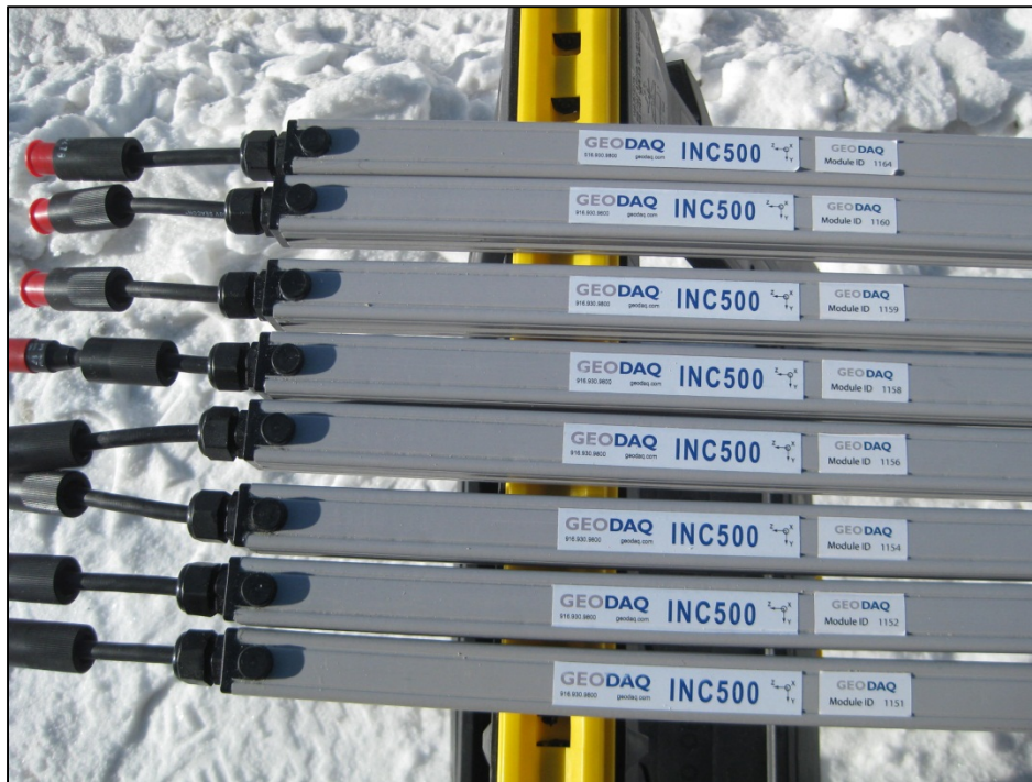
Figure A-6. Order of INC500 module serial numbers before installation. It is good practice to record this order both in a field book and through photographs. (Photograph by M. Darrow, March 2010)
