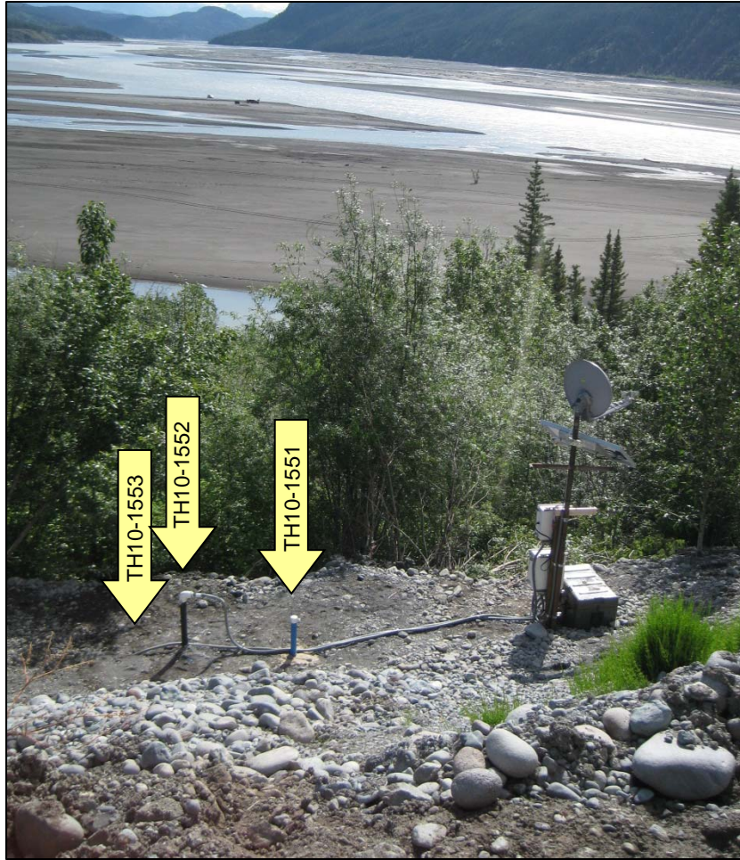
Figure 8. Relative locations of the measured casings and piezometer installation at the Chitina Dump Slide. Vertical arrows are labeled with the test hole identifiers; the installations were located on a drill bench downhill of the roadway embankment. This photograph was taken from the McCarthy Road embankment looking east towards the Copper River. (Photograph by M. Darrow)
