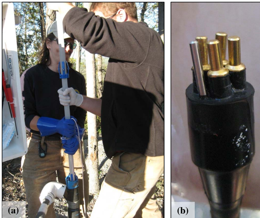
Figure A-21. Retrieving the INC500 in September 2010 to adjust the positioning of the centralizers. (a) Pulling the INC500 from the guide casing. (b) Some of the connectors demonstrated twisting. (Photographs courtesy of S. Huang)
