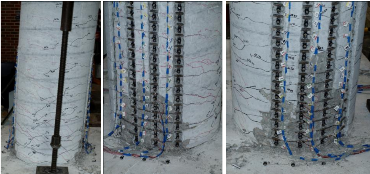
Figure 2-135. Test 12 – Peak Pull Cycle at ( \mu_{-7.9}^{66.88 \text{ sec}} = -6.53'' ) – (Left) Back Side of the Specimen, (Middle) South Side, and (Right) North Side
