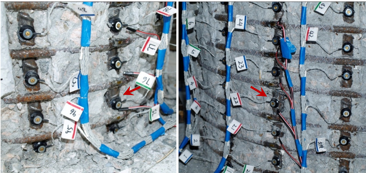
Figure 2-110. Test 11 – (Left) Additional Deformation in North Buckled Region and (Right) Additional Deformation in South Buckled Region
