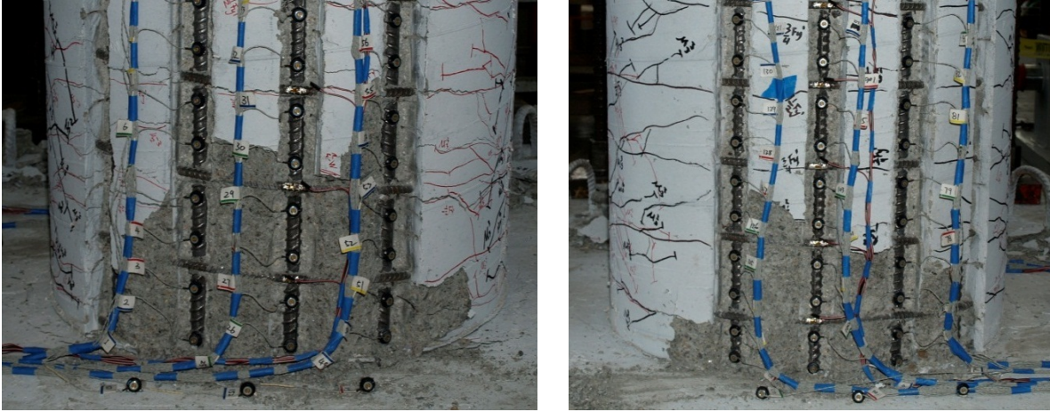
Figure 2-203. Test 14 – (Left) Extent of Crushing on the South Side of the Specimen during ( \mu_4^{+3} = 3.19'' ) and (Right) Extent of Crushing on the North Side during ( \mu_4^{-3} = 3.20'' )
