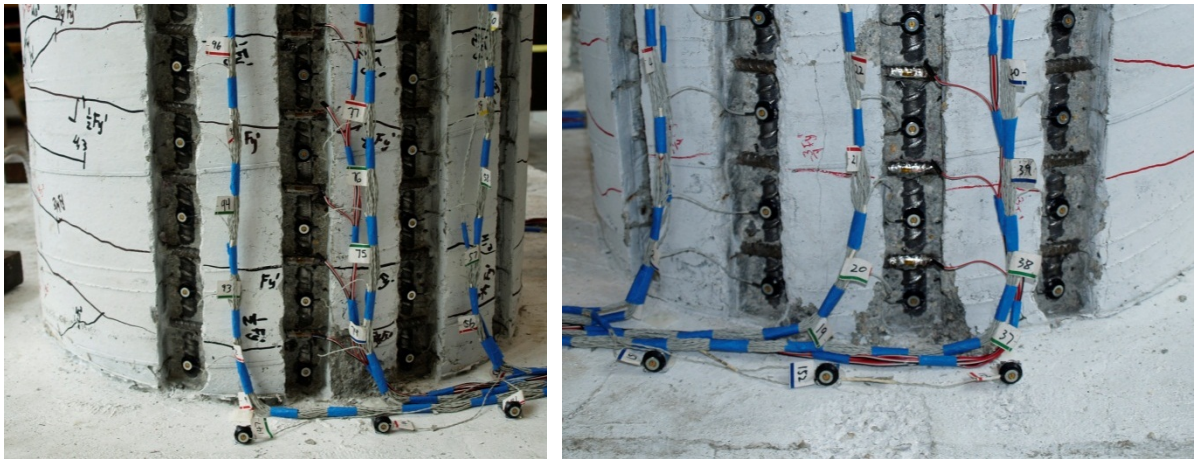
Figure 2-236. Test 15 – (Left) Crushing on the North Side of the Specimen during ( \mu_{1.5}^{-3} = -1.25'' ) and (Right) Crushing on the South Side during ( \mu_2^{+1} = 1.68'' )
