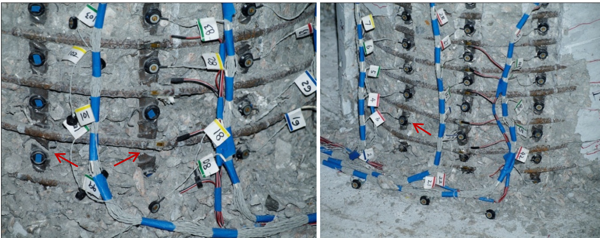
Figure 2-14. Test 9 – Photos during ( \mu_{10}^{+1} = 8.38'' ) (Left) Rupture of N4 and N3 and (Right) Buckling of S2 and Additional Deformation in Previously Buckled Bar S3
