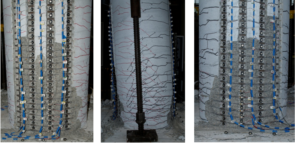
Figure 2-312. Test 17 – (Left, Middle, and Right) South, Back, and North Side of the Specimen during ( \mu_{9,0}^{32.76 \text{ sec}} = 7.49'' ) Respectively
