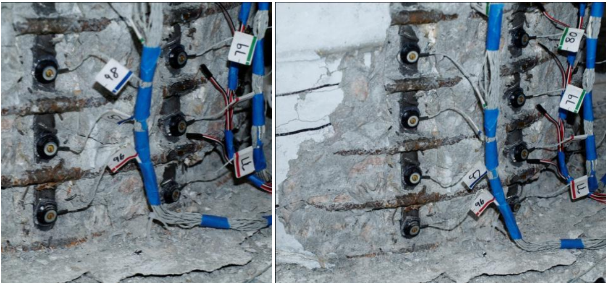
Figure 2-137. Test 12 – (Left) Buckling of Extreme Fiber Bar N3 after Reversal from ( \mu_{9,9}^{68.62sec} = 8.22'' ) and (Right) Buckling of Bar N4 at ( \mu_{-1,4}^{69.4sec} = -1.14'' )
