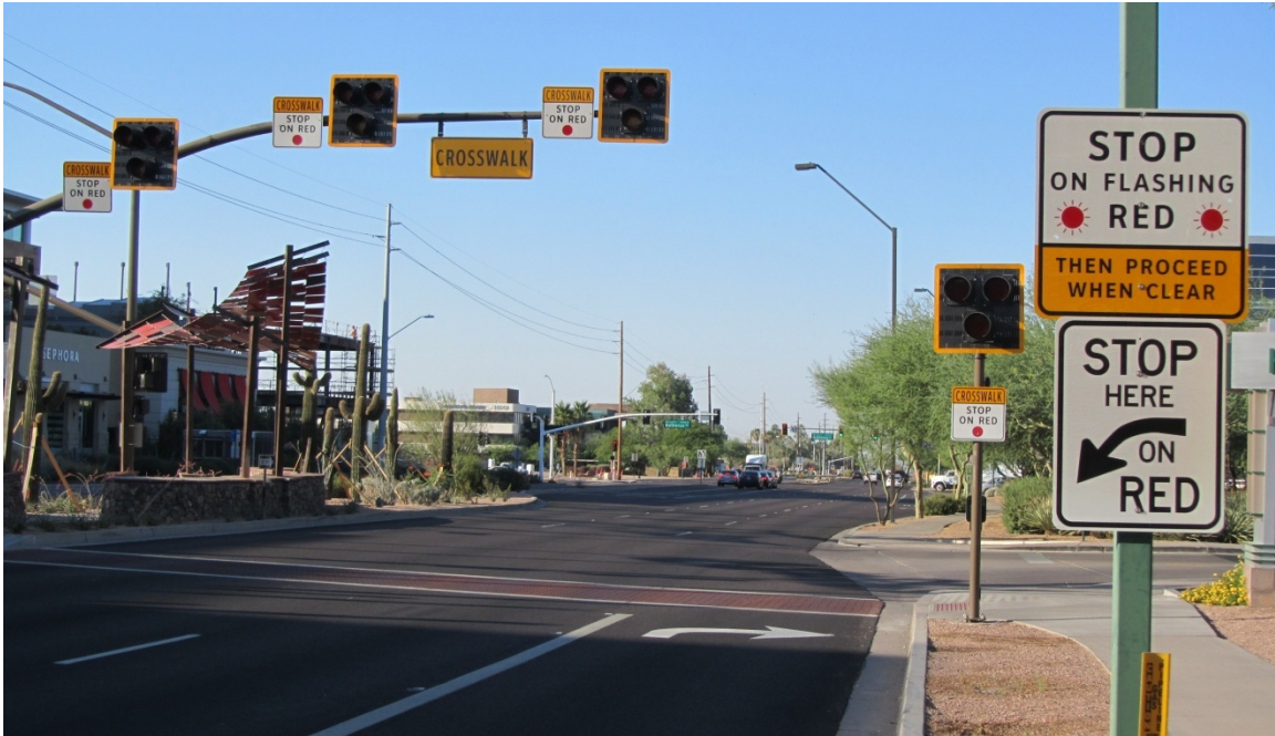
Figure 5-2: A picture of a PHB showing an overhead sign instructing drivers to stop during the solid red indication.
