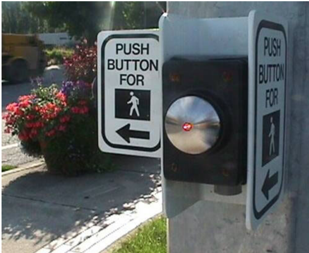
Figure 1-10: A photograph of a push button that confirms it has been pressed
