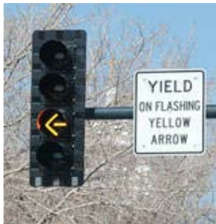
Figure 1-6: Picture of Flashing Yellow Arrow
