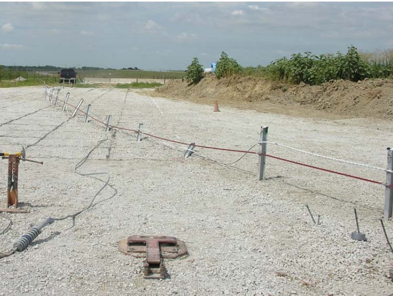
Figure 41. System Damage, Test No. NYCC-1
