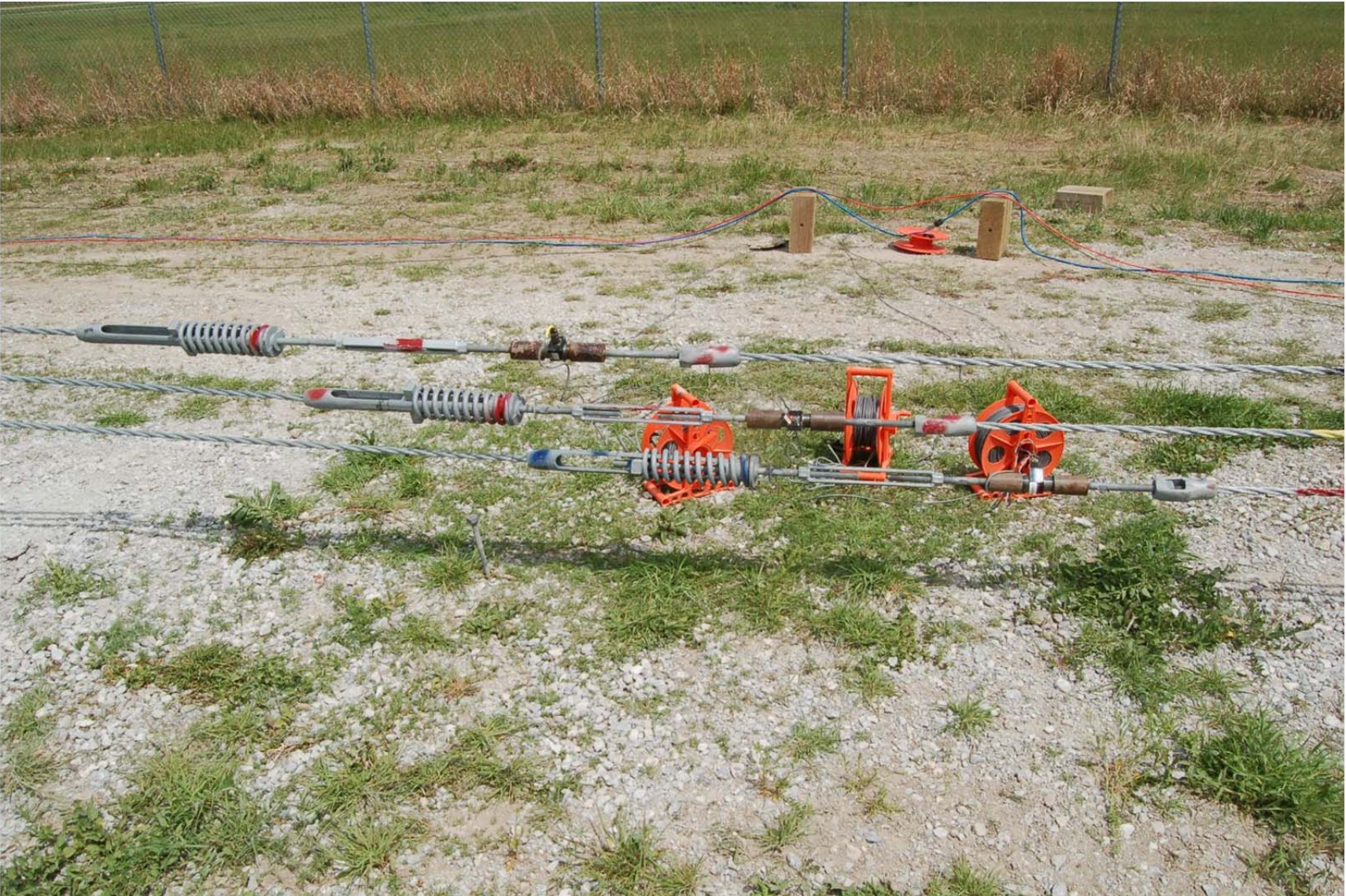
Figure 98. Cable Splices and Load Cells, Test No. NYCC-3
