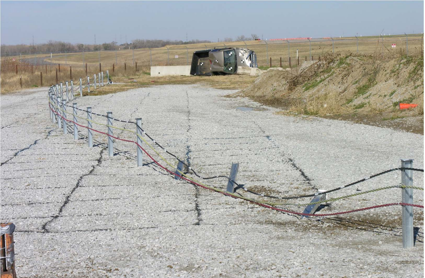
Figure 71. Vehicle Final Position and Trajectory Marks, Test No. NYCC-2
