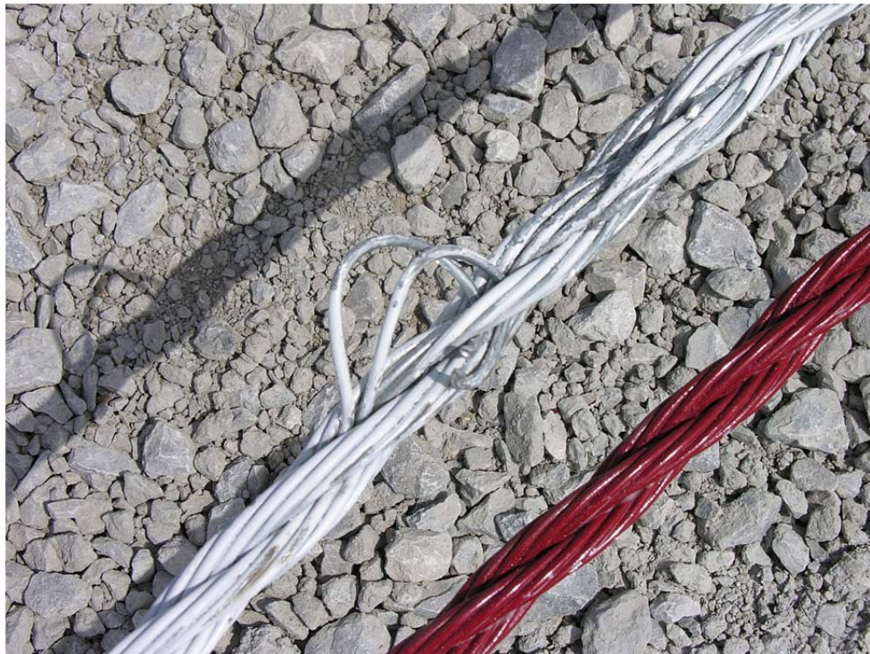
Figure 46. System Damage: Middle Cable between Post Nos. 17 and 18, Test No. NYCC-1
