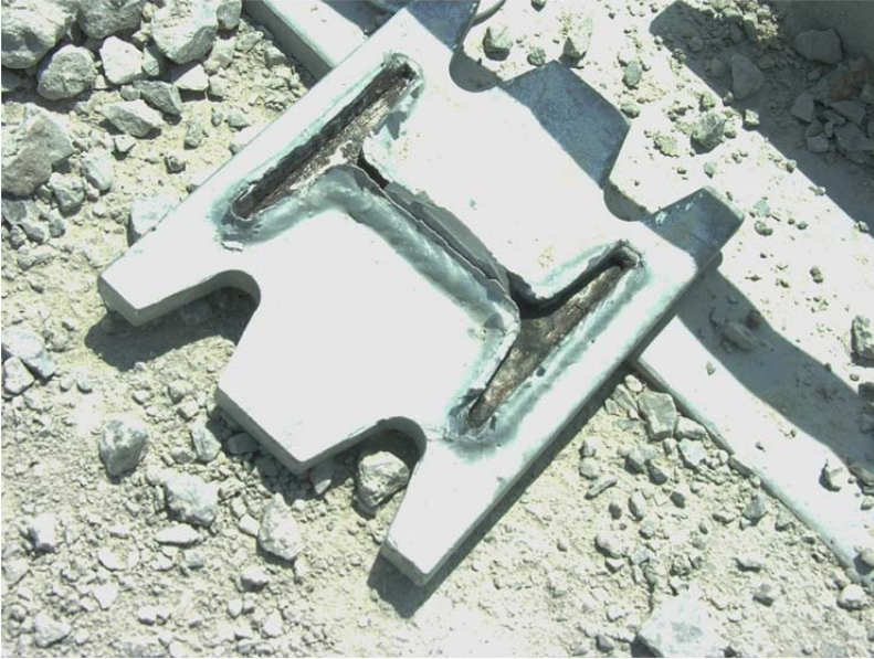
Figure 42. System Damage: Upstream Anchor and Post No. 1, Test No. NYCC-1
