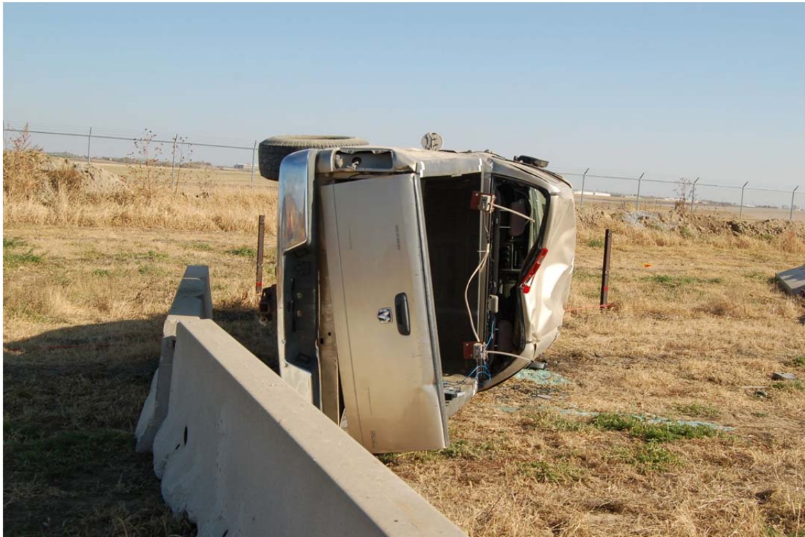
Figure 75. Vehicle Damage, Test No. NYCC-2
