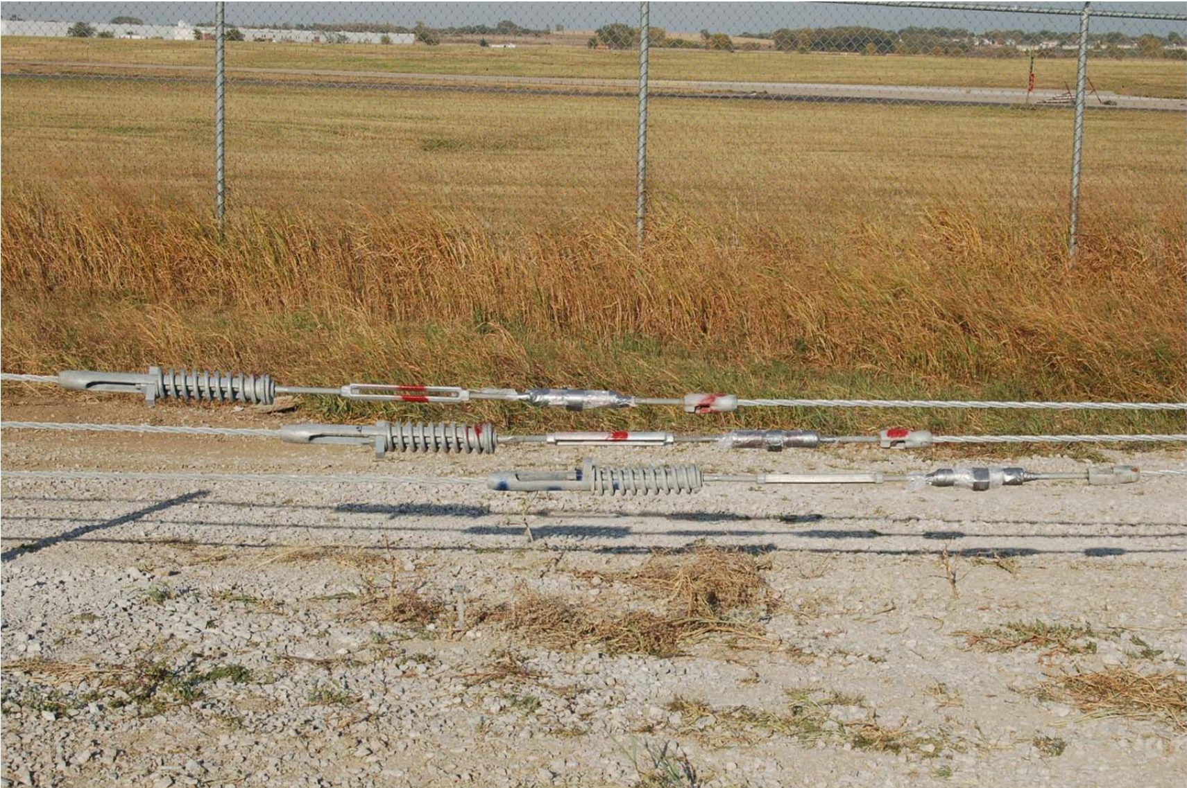
Figure 65. Cable Splices and Load Cells, Test No. NYCC-2
