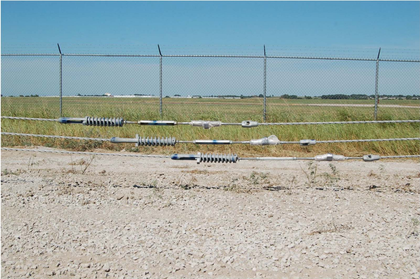
Figure 31. Cable Splices and Load Cells, Test No. NYCC-1
