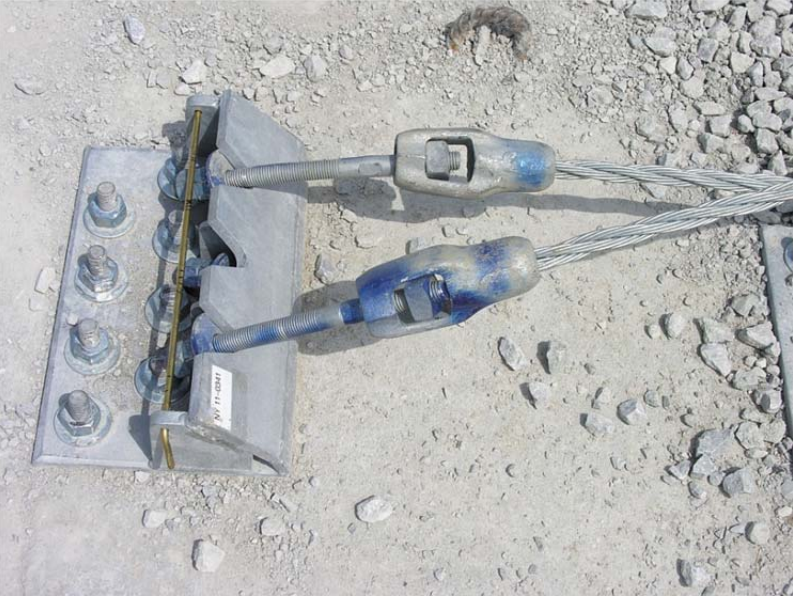
Figure 45. System Damage: Downstream Angle Plate and Middle Cable, Test No. NYCC-1
