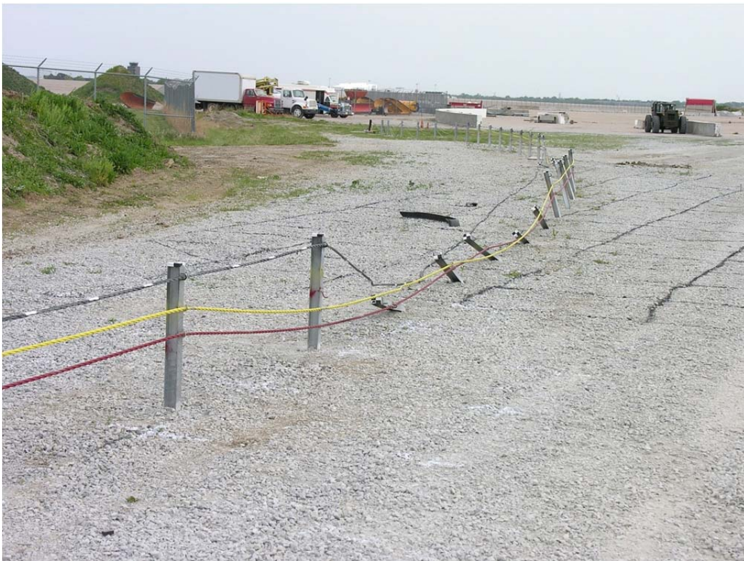
Figure 107. System Damage, Test No. NYCC-3
