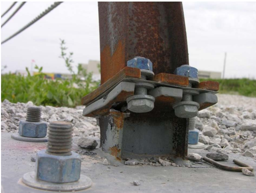
Figure 116. System Damage: Post No. 40, Test No. NYCC-3
