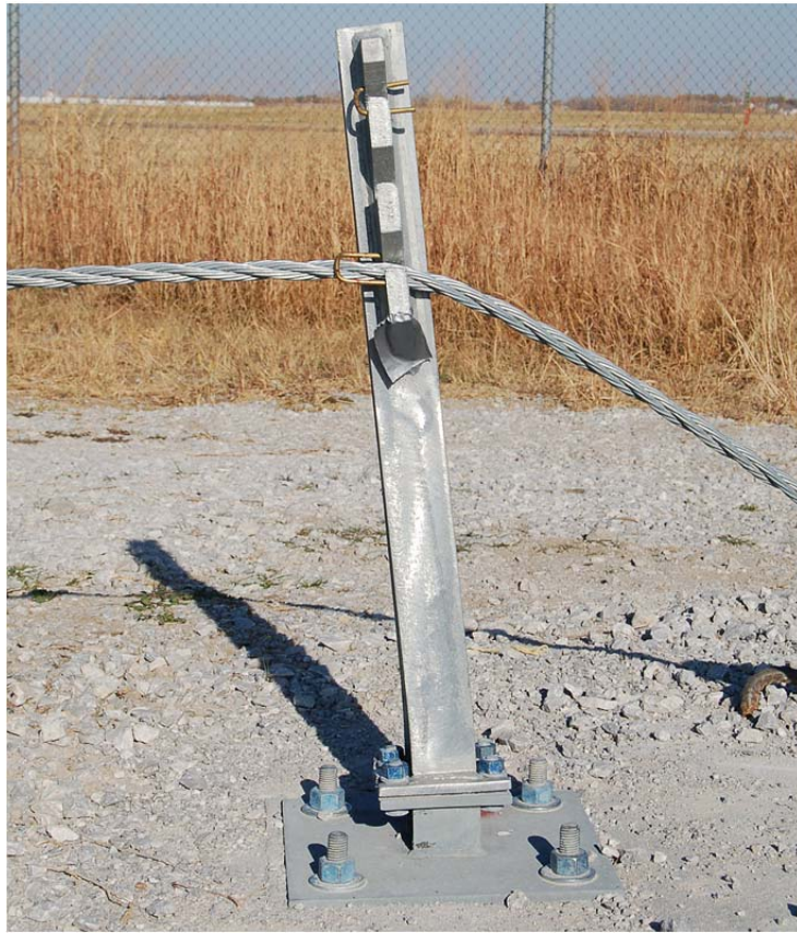
Figure 72. System Damage: Upstream Anchorage, Test No. NYCC-2
