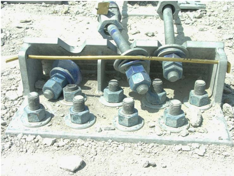
Figure 43. System Damage: Upstream Angle Plate and Top Cable, Test No. NYCC-1
