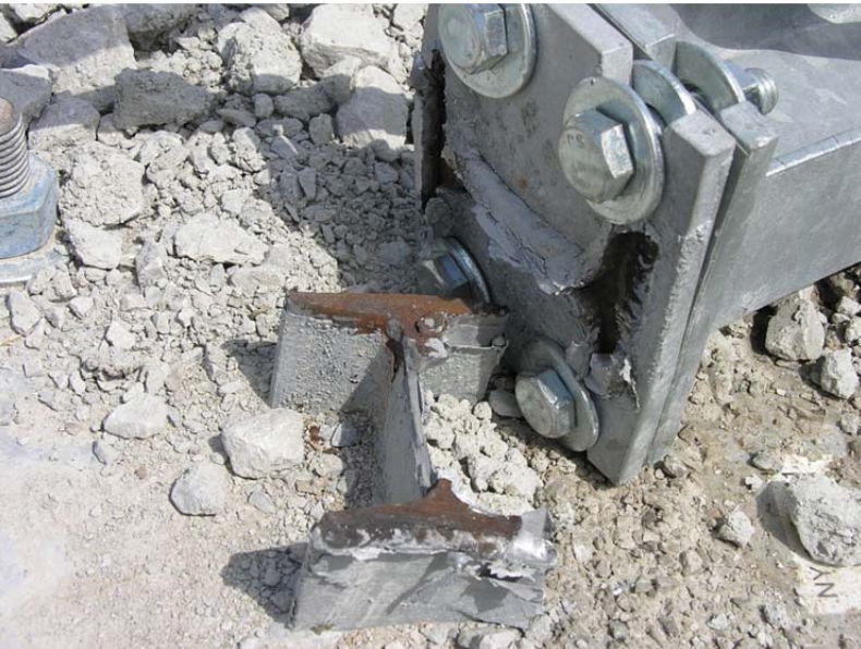
Figure 44. System Damage: Downstream Anchor and Post No. 40, Test No. NYCC-1
