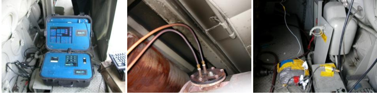
Figure 3-7. Installation of PEMS on an F59PHI Locomotive Prime Mover Engine (a) PEMS main unit (front-view); (b) exhaust sampling port and metal tubes; (c) sensor array box
