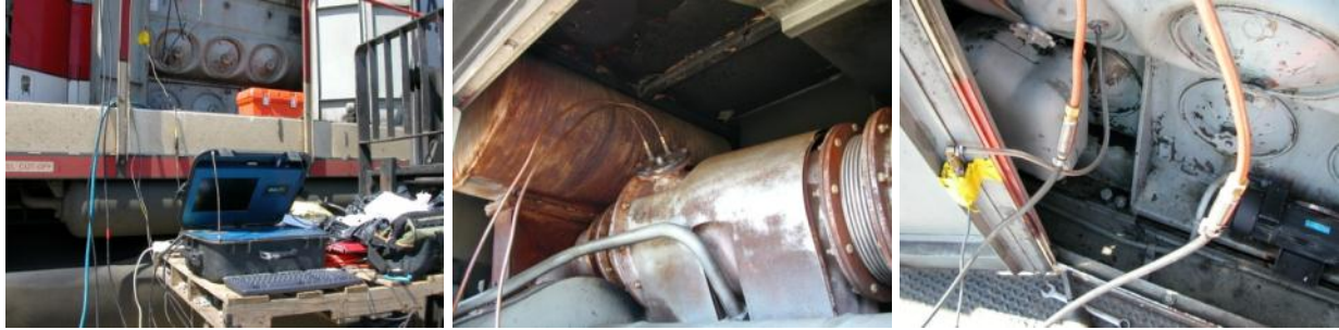
Figure 3-11. Installation of PEMS on a GP40 Locomotive Prime Mover Engine (a) PEMS main unit (front-view); (b) exhaust sampling port and metal tubes; (c) sensor array box
