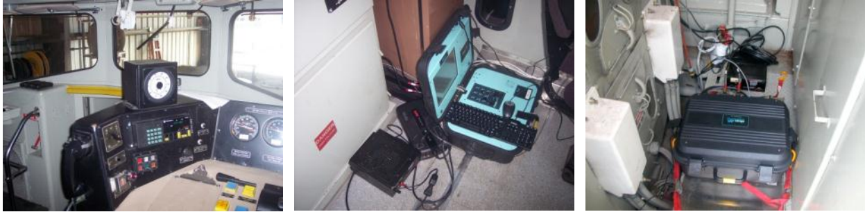
Figure 4-2. Placement of Instrumentation for Over-the Rail Testing of Locomotives (a) GPS units on left side of locomotive cab during testing of F59PH locomotives; (b) PEMS unit in the locomotive cab during testing of F59PH locomotives; (c) PEMS unit in the generator room during testing of GP40 locomotive
