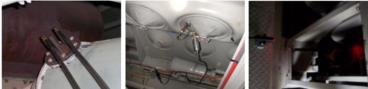
Figure 3-4. Installation of Sensors on an F59PH Locomotive Prime Mover Engine (a) exhaust sampling port and metal tubes; (b) manifold absolute pressure (MAP) sensor; (c) RPM sensor
