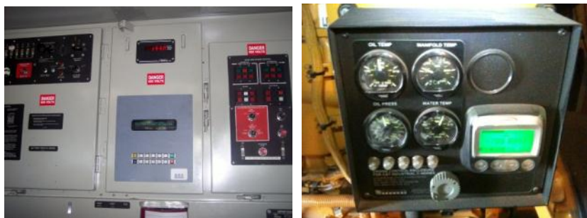
Figure 3-6. Engine Activity Data Sources During Testing of an F59PH Locomotive (a) prime mover engine activity digital display in locomotive cab; (b) head end power engine activity digital display on head end power engine
