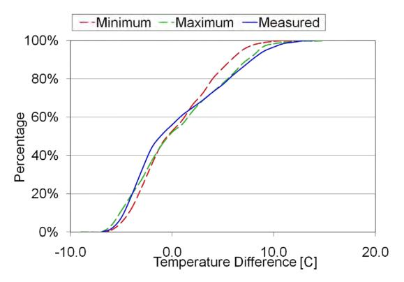
Figure 2-28: Measured versus modeled cumulative frequency distribution for thermal gradient through JPCP pavement in March with k = 0.94 BTU / hr-ft-°F, the adjusted thermal conductivity value.
