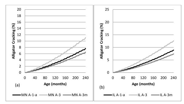
Figure 2-40: Predicted alligator cracking for a flexible pavement with different bases and an A-6 subgrade (a) in Minneapolis analyzed with DARWin-ME, and (b) in Champaign analyzed with DARWin-ME.
