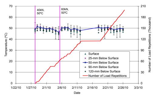
Figure 4-13: Daily average temperatures at surface and various depths of Section 609HB.
