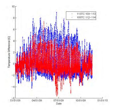
Figure 2-21: Hourly PCC temperature differences throughout AC-over-PCC (Cell 106 in red) and JPCP (Cell 113 in blue) thicknesses illustrating the insulating effect of an AC overlay.
