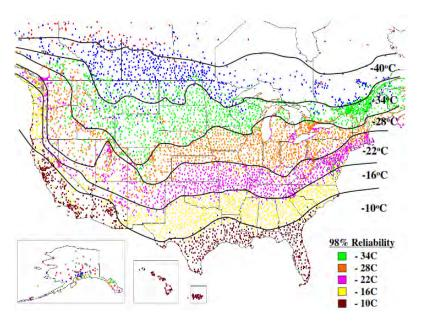
Figure 5-23: Recommended low temperature PG grade from LTPPBind (from Bennert 2009).
