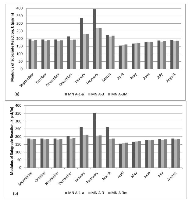
Figure 2-37: Modulus of subgrade reaction, k, under a rigid pavement with different bases and an A-6 subgrade in Minneapolis analyzed with a) the MEPDG and b) DARWin-ME.
