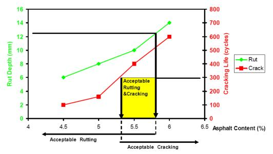
Figure 5-26: Overlay binder content to optimize resistence to rutting and fatigue cracking from Zhou et al (2006).
