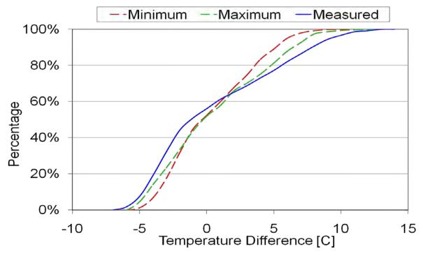
Figure 2-25: Measured versus modeled cumulative frequency distribution for thermal gradient through JPCP pavement in July with k = 1.25 BTU / hr-ft-°F.
