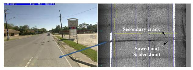
Figure 5-16: Illinois tollway saw-and-seal (Elsefi 2011).
