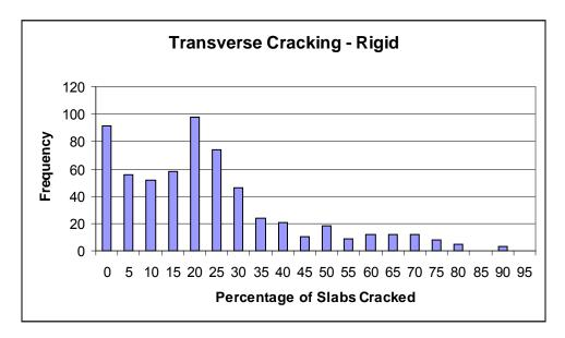
Figure 2-7: Frequency distribution of predicted transverse cracking values for rigid pavement structure.
