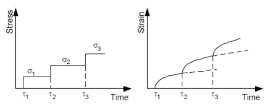
Figure 3-8: Schematic representation of Boltzman's superposition principle (adopted from *UMN Online Lecture 2011*).
