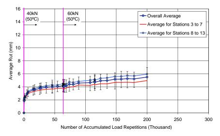
Figure 4-16: Average deformation for Section 609HB.
