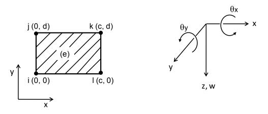
Figure 3-10: Finite element *ijkl*.
