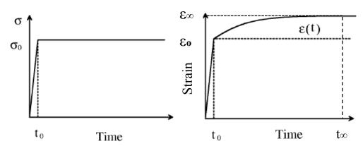
Figure 3-7: Stress-strain responses under different load durations (adopted from Chen 2000).
