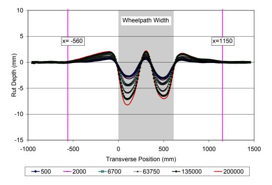
The average transverse cross-section for the example section discussed here is illustrated in Figure 4-15. Note the evolution of rut depth of the course of repeated loading.
