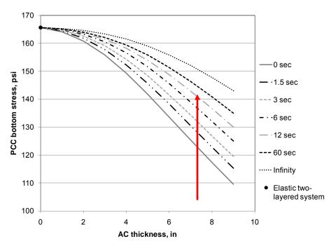
Figure 3-26: PCC bottom stresses versus AC thickness.
