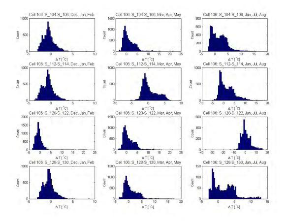
Figure 2-19: ΔT Histograms for cell 106 sensor pairings, organized vertically by season.
