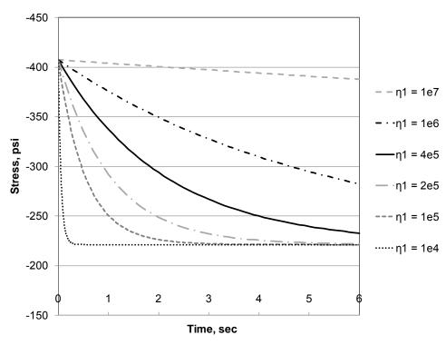
Figure 3-21: Stress versus time for a factorial of dashpot viscosities of the Kelvin-Voigt element.
