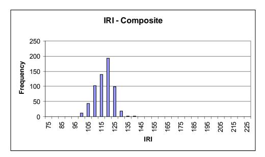
Figure 2-2: Frequency distribution of predicted IRI values for composite pavement structure.
