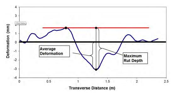
Figure 4-14: Illustration of maximum rut depth and average deformation of a leveled profile.
