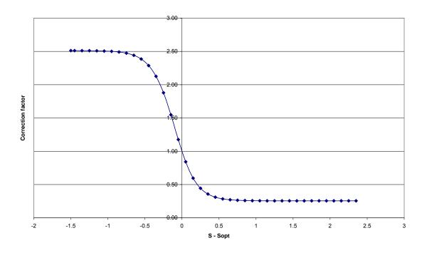
Figure 2-32: Correction factor as a function of the degree of saturation (24).
