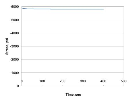
Figure 3-14: Stress at the bottom of the viscoelastic placed on viscoelastic Winkler foundation.
