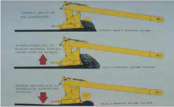
Figure 5-10: Screed movement with material head variation.
