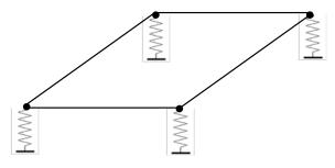
Figure 3-11: Spring idealization of Winkler foundation using concentrated springs at the nodes of the plate element.
