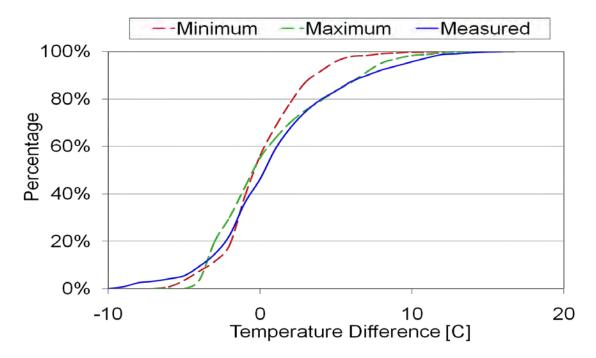
Figure 2-27: Measured versus modeled cumulative frequency distribution for thermal gradient through JPCP pavement in March with k = 1.25 BTU / hr-ft-°F, which is the MEPDG default value.
