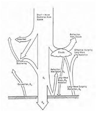
Figure 2-1: Heat transfer between pavement and air on a sunny day (NCHRP 2004).
