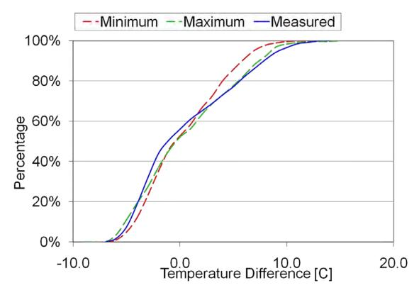
Figure 2-26: Measured versus modeled cumulative frequency distribution for thermal gradient through JPCP pavement in July with k = 0.94 BTU / hr-ft-°F.
