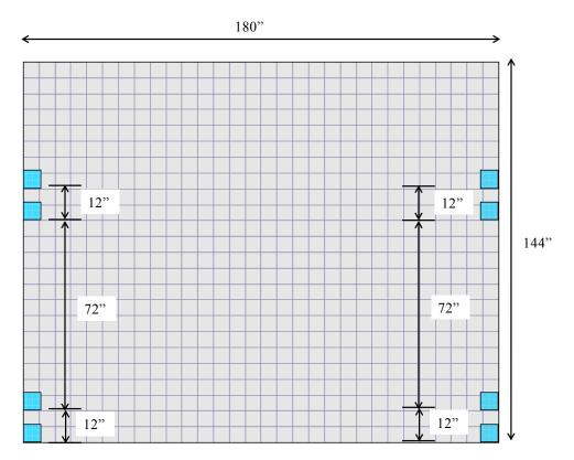
Figure 3-34: Mesh and load configuration for the composite pavement subjected to SADW edge loading.
