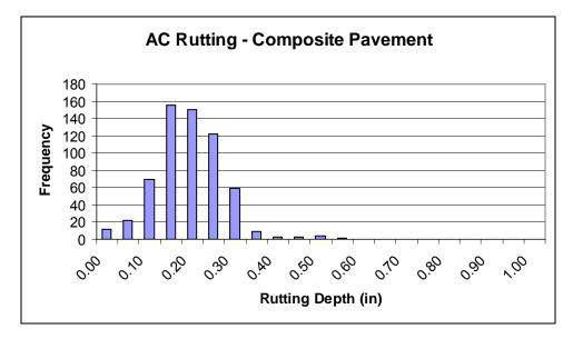
Figure 2-4: Frequency distribution of predicted rutting values for composite pavement structure.
