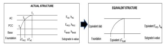
Figure 3-5: Conversion of a composite pavement to an equivalent PCC structure.
