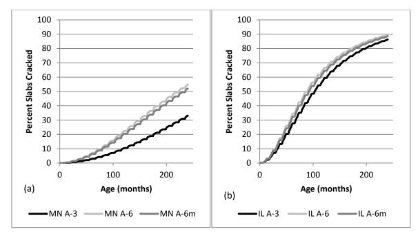
Figure 2-36: Predicted cracking for a rigid pavement with different subgrades and an A-1a (a) in Minneapolis analyzed with DARWin-ME, (b) in Champaign analyzed with DARWin-ME.
