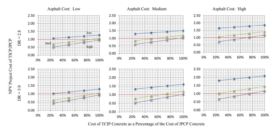
Figure 6-1: The ratio of the NPV of TICP to the NPV of JPCP, which are dependent on asphalt cost, JPCP concrete cost, TICP concrete cost as a percentage of JPCP concrete cost, and discount rate.
