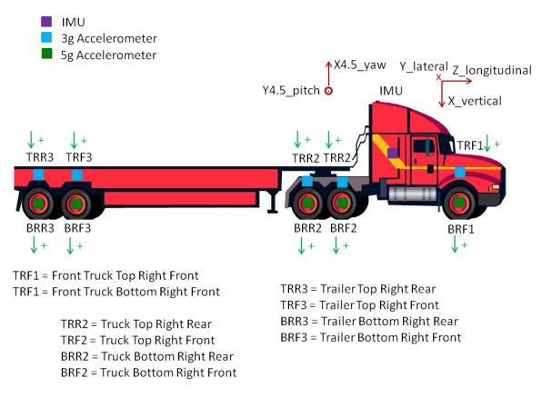
Figure 2.2: Accelerometer locations on right side of truck.
