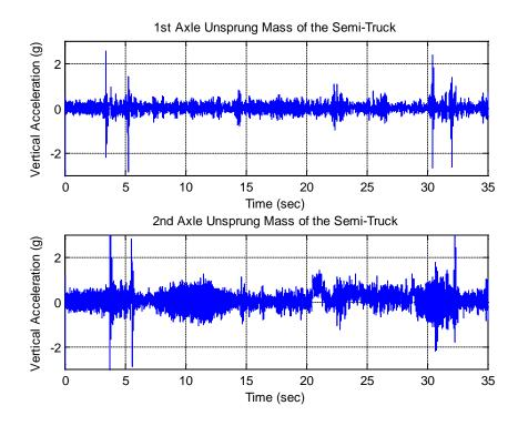
Figure 2.14: Axle vibrations on semi-truck at 50 mph.
