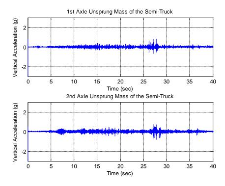
Figure 2.11: Axle vibrations on semi-truck at 20 mph.
