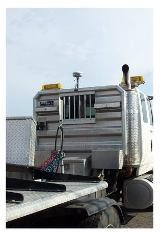
Figure 2.17: Differential GPS system located above tractor cab.
