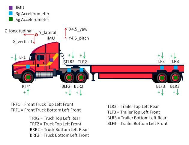
Figure 2.4: Accelerometer locations on left side of truck.
