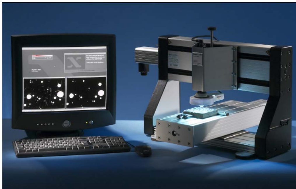
Figure 1.5. Basic configuration of RapidAir 457 (Jakobsen et al., 2006)
