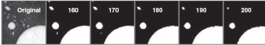
Figure 1.17. Example of threshold value comparison (Carlson, 2006)
