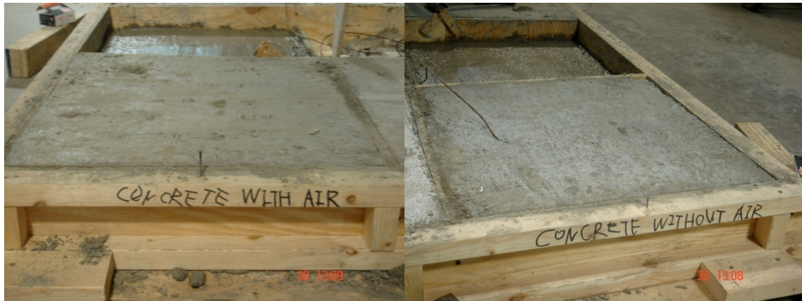
Figure 2.10. 2 ft x 2 ft NA and NN concrete placed in forms
