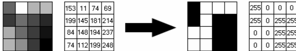
Figure 1.18. Example of threshold conversion from scanned to binary pixel intensities (Sutter, 2007)
