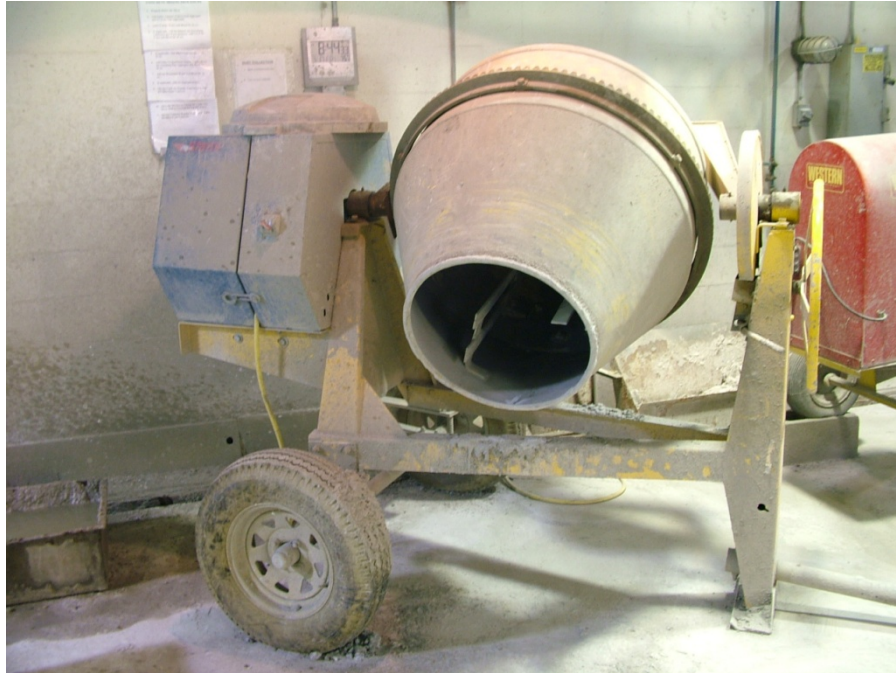
Figure 2.1. Portable concrete mixer
