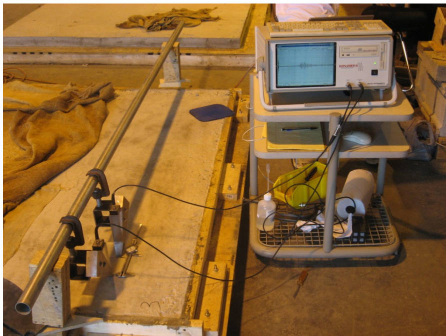
Figure 2.9. Rayleigh wave test setup on hardened concrete
