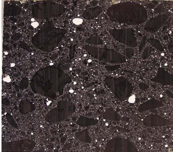
Figure 1.6. Image of specimen surface after contrast enhancement (Jakobsen et al., 2006)
