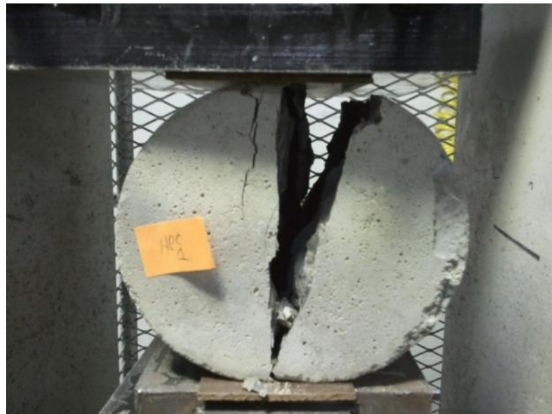
Figure 3-4: Typical tensile splitting test failure (ASTM C 496-11)
