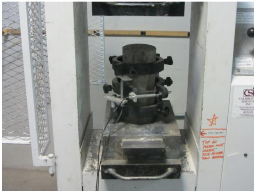
Figure 3-7: Setup for modulus of elasticity and Poisson's ratio (ASTM C 469-10)
