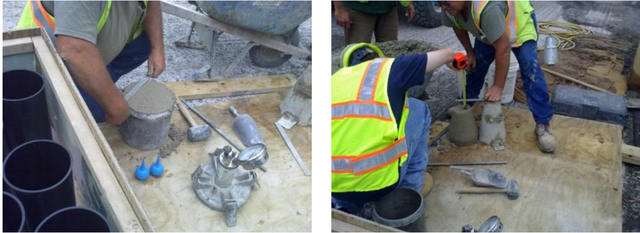
Figure 2-10: Fresh concrete properties tests. Left: air content test; Right: slump test
