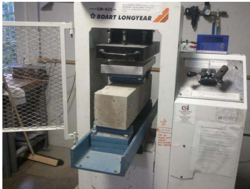
Figure 3-6: Flexural strength test setup (ASTM C 78-10)
