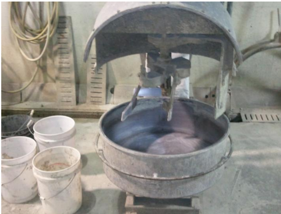
Figure 3-2: Eirich S-1 counter-current concrete mixer
