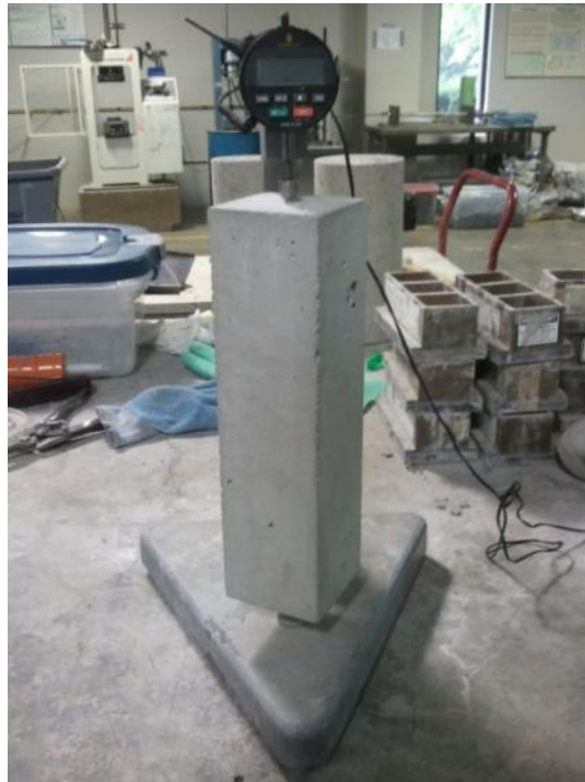
Figure 3-13: ASTM C 157-08 setup for drying shrinkage of concrete
