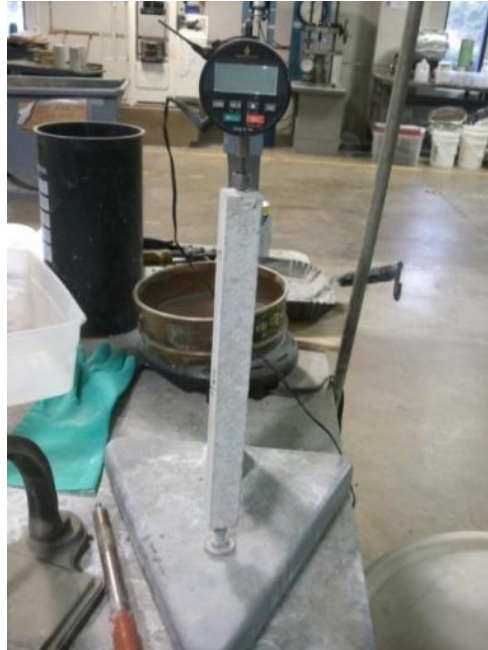
Figure 3-10: Humboldt digital comparator model BG2600-16001 (ASTM C 531-00 setup)
