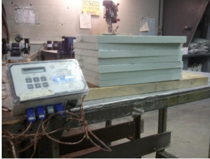
Figure 3-9: Heat of hydration setup (ASTM C 1064-08)
