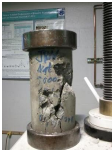
Figure 3-3: Sample concrete specimen post compressive strength testing
