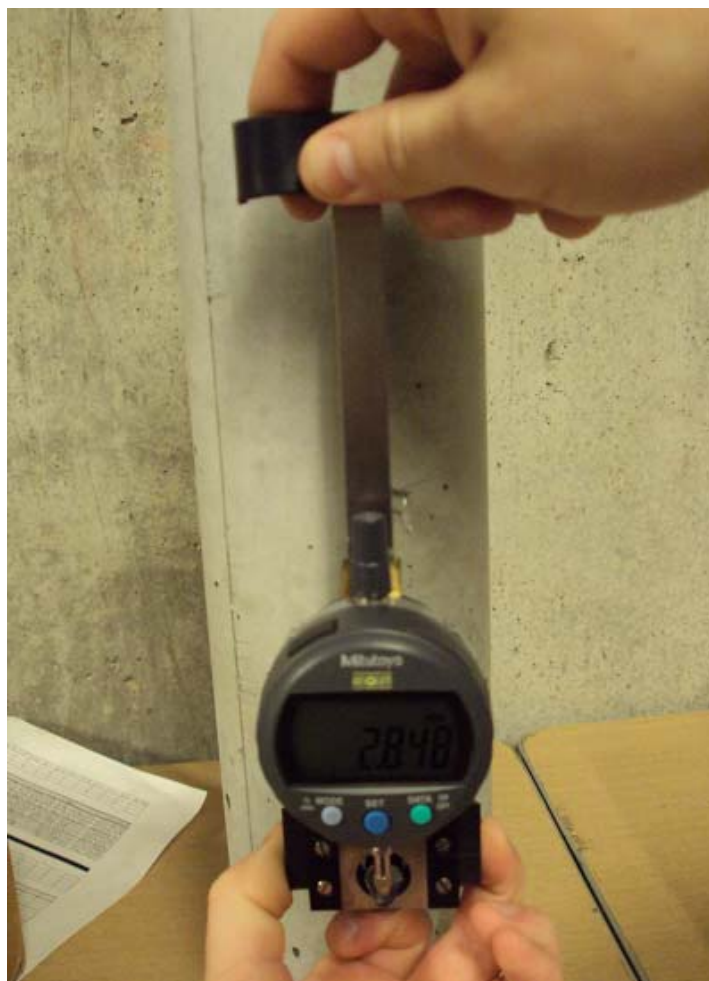
Figure 2.3 – DEMEC Reading Taken on Specimen
