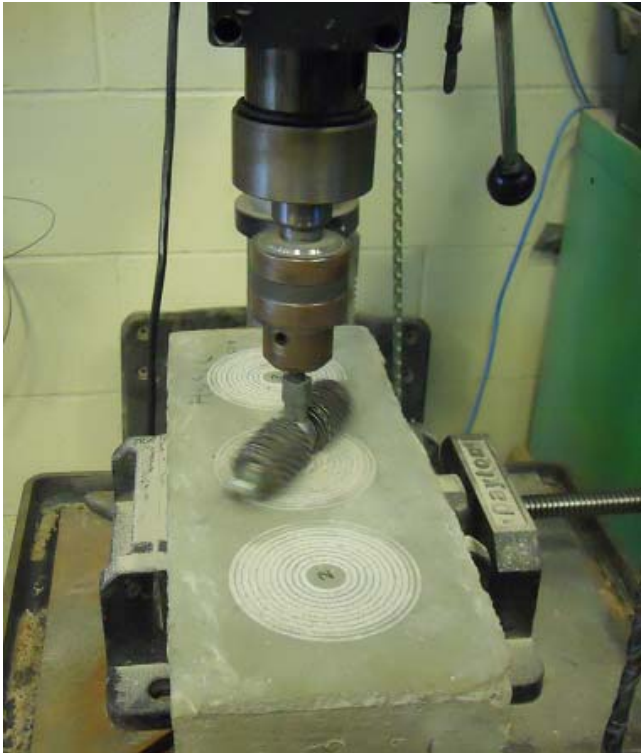
Figure 2.13 - Abrasion Resistance Test In Progress
