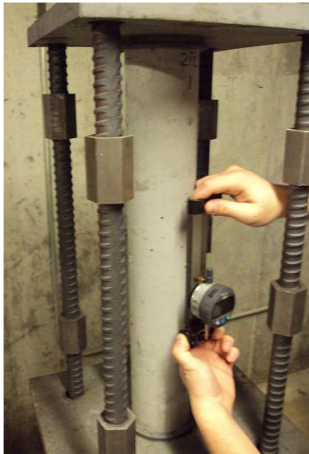
Figure 2.10 - Reading Taken on Creep Specimen
