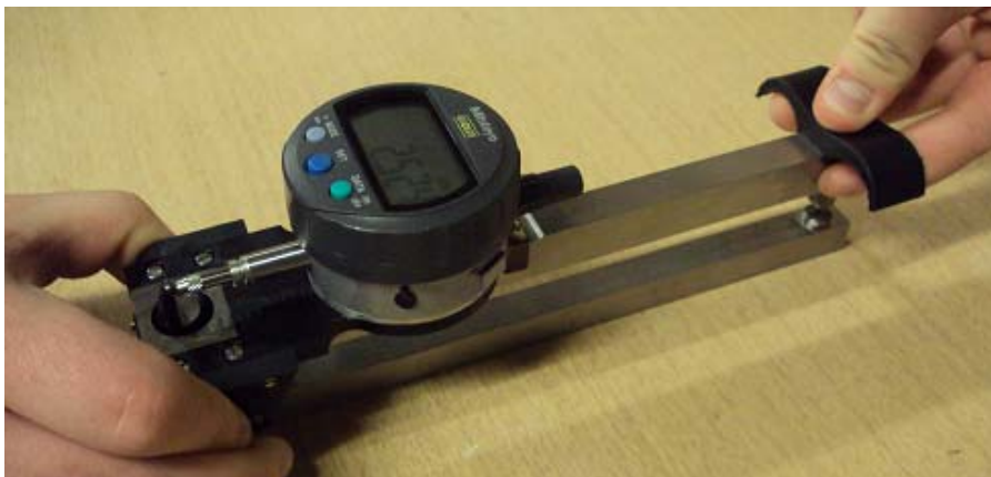
Figure 2.5 - Reading Taken on Reference Bar
