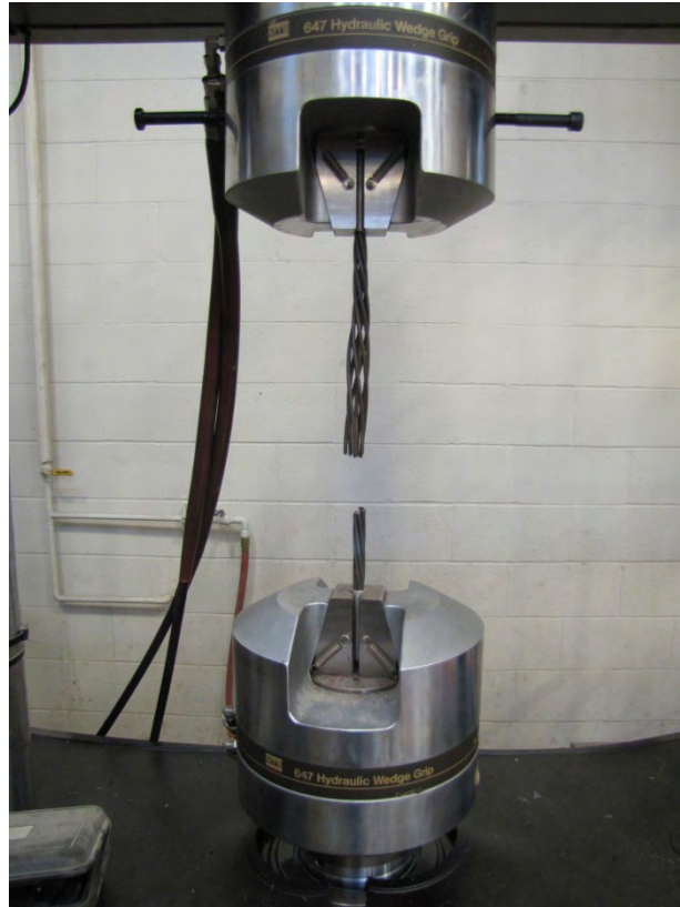
Figure 3.4 – Fractured Tension Test Specimen
