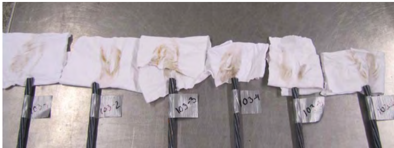
Figure 3.31 – Towel Wipe Results for Strand Type 103
