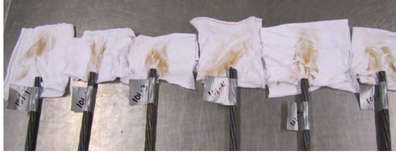
Figure 3.29 – Towel Wipe Results for Strand Type 101
