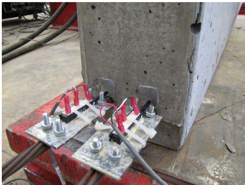
Figure 4.28 – Linear Potentiometer Setup on Four-Point Loading Tests
