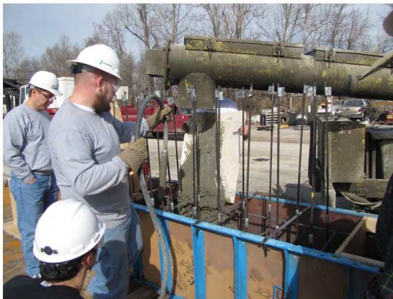
Figure 3.23 – Casting the LBPT Specimen
