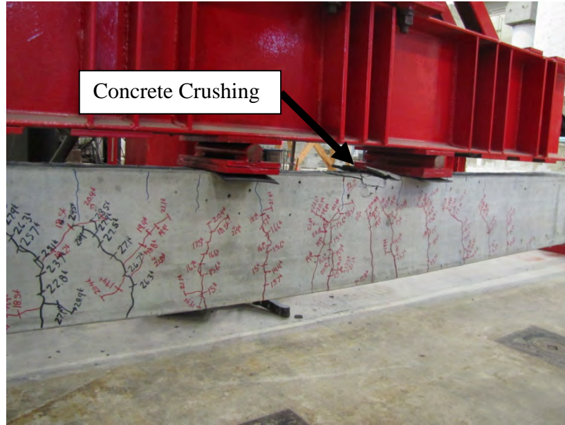
Figure F.31 – S10-2-2_73 at Failure
