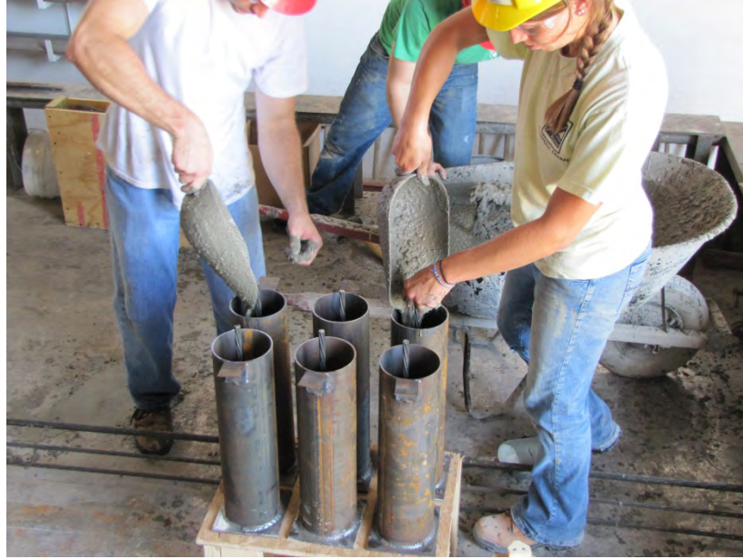
Figure 3.11 – Filling Specimens for NASP Test in Concrete
