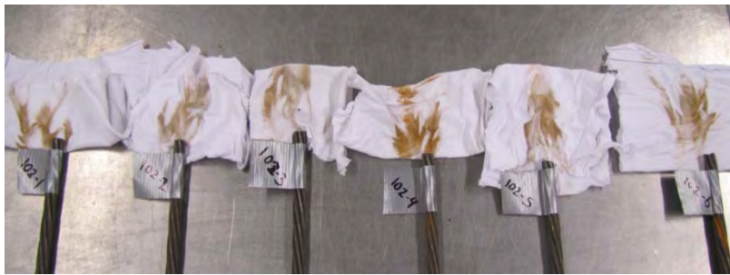
Figure 3.30 – Towel Wipe Results for Strand Type 102
