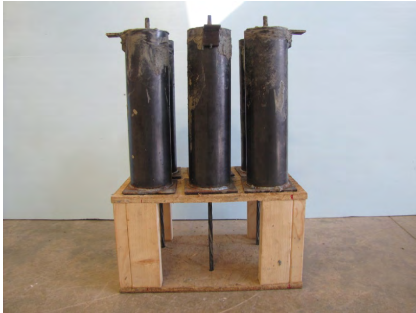
Figure 3.10 – NASP Mold and Strand Setup
