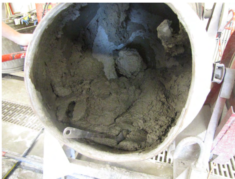
Figure 3.7 – Mortar Mix in Drum Mixer
