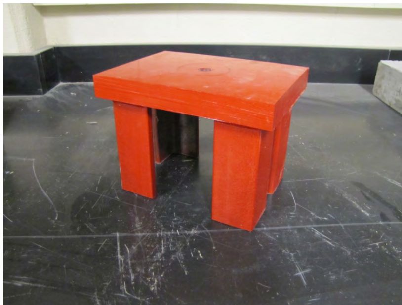
Figure 3.26 – Steel Table for LBPT
