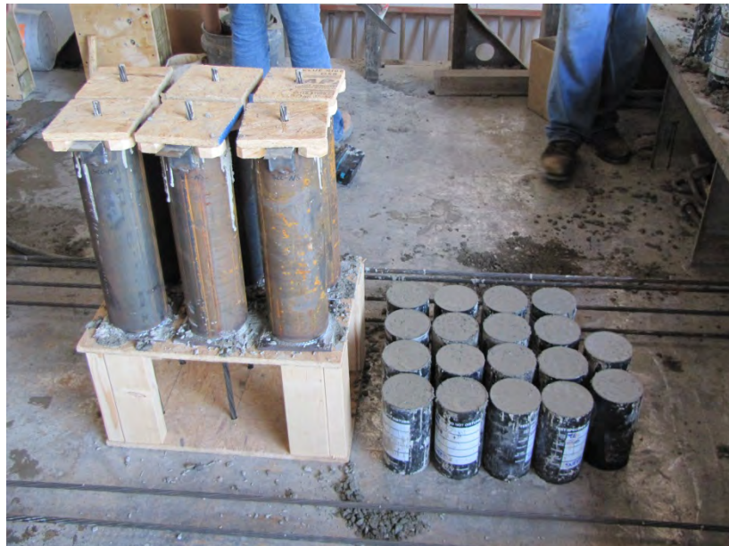
Figure 3.12 – Capped NASP in Concrete Specimens and Cylinders
