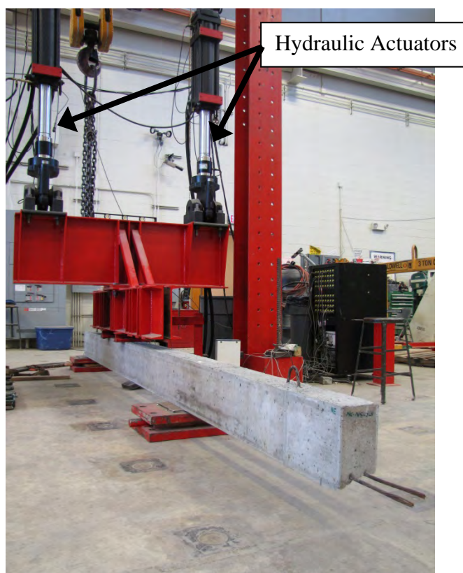
Figure 4.24 – Four-Point Loading Test Setup for Evaluating 58-in. (1,473 mm) Embedment Length
