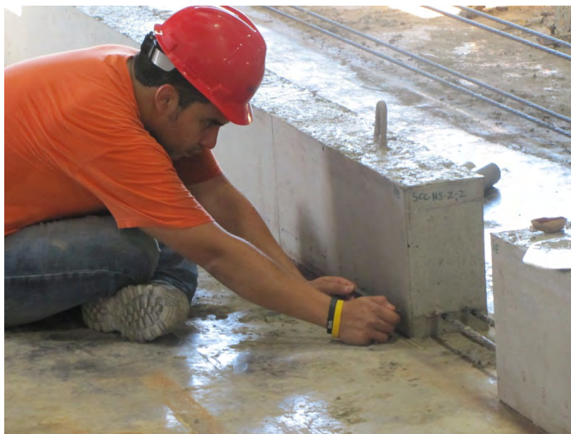
Figure 4.11 – Setting DEMEC Points with Setting Bar
