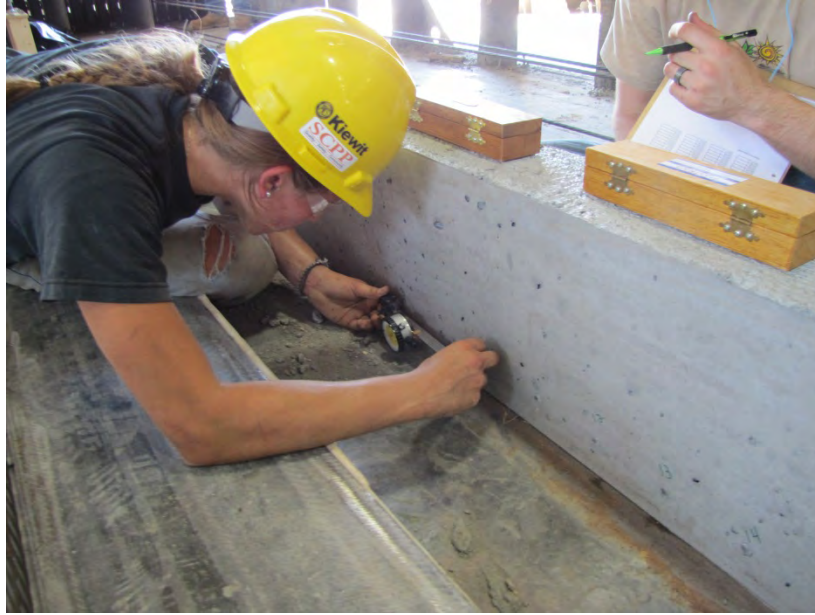
Figure 4.13 – Taking DEMEC Readings
