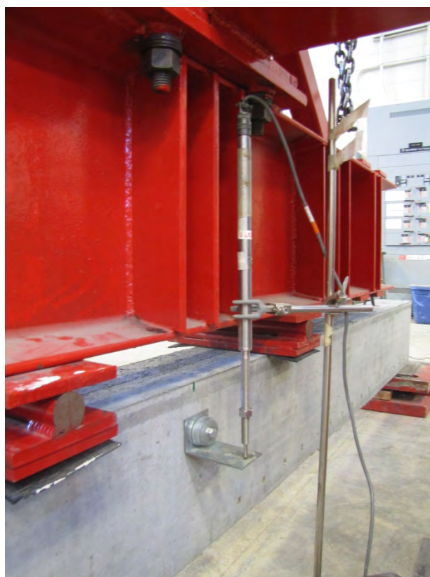
Figure 4.27 – LVDT Setup for Measuring Deflection at Midspan
