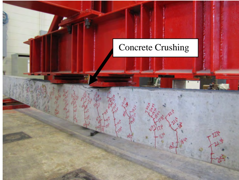
Figure F.19 – C10-2-1_73 at Failure
