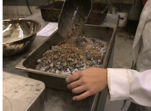
(b) Mixing Water in the Aggregates
