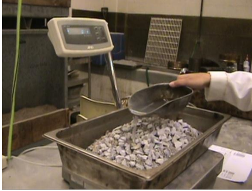
(a) Adding Water to Aggregates
