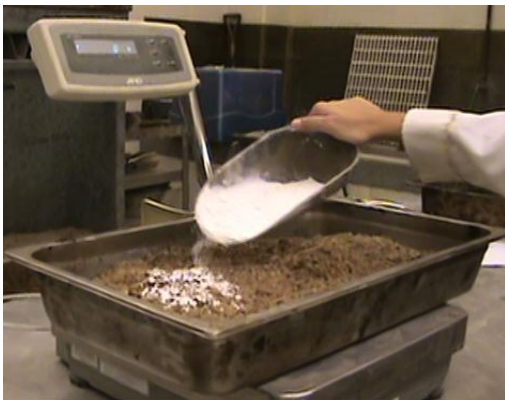
(c) Adding Additive to the Wet Aggregates
