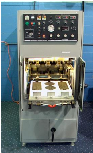
(a) APA with Beam and Cylindrical Samples
