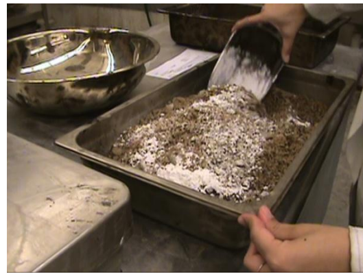
(d) Mixing Additive with Aggregates
