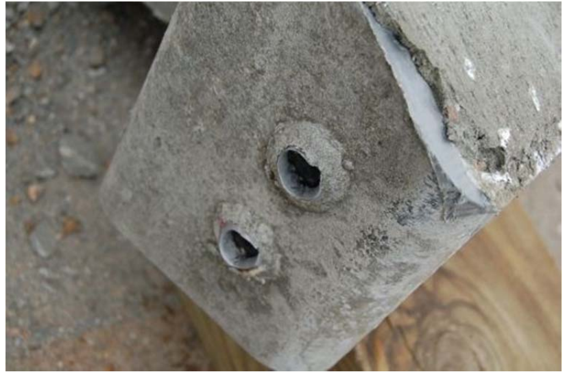
Figure 79. Component Damage – Long Rail Segment, Test No. PCRB-1
