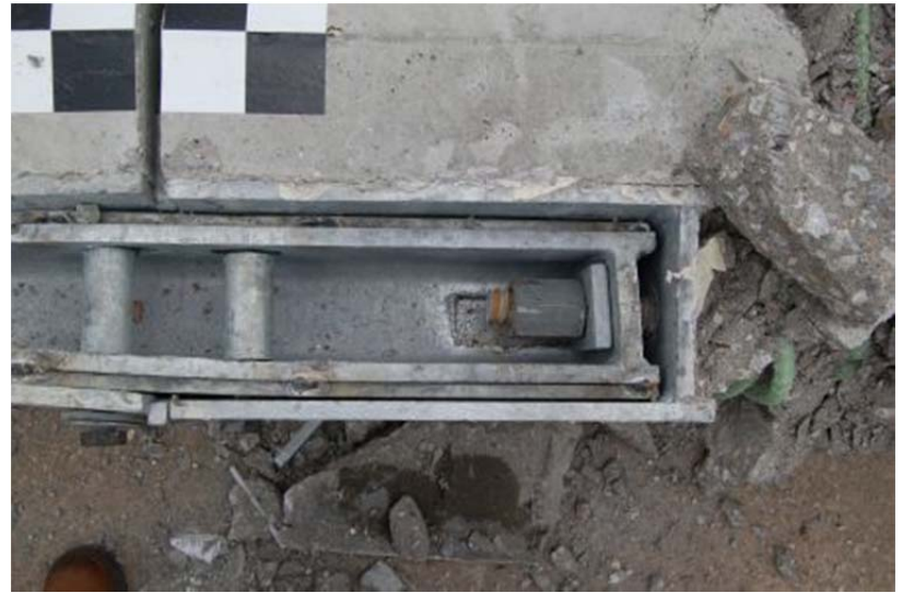
Figure 155. Component Damage – Steel Pockets, Test No. PCRB-4
