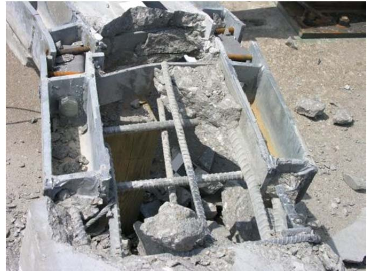
Figure 89. Component Damage – Loose Concrete Removed, Test No. PCRB-2
