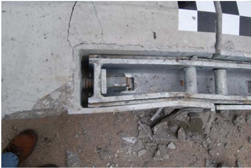
Figure 155. Component Damage – Steel Pockets, Test No. PCRB-4
