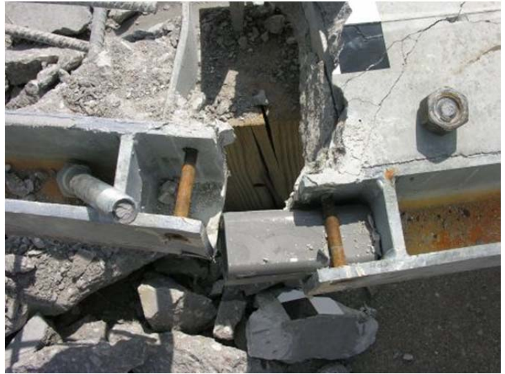
Figure 88. Component Damage – Back Pocket Assembly, Test No. PCRB-2
