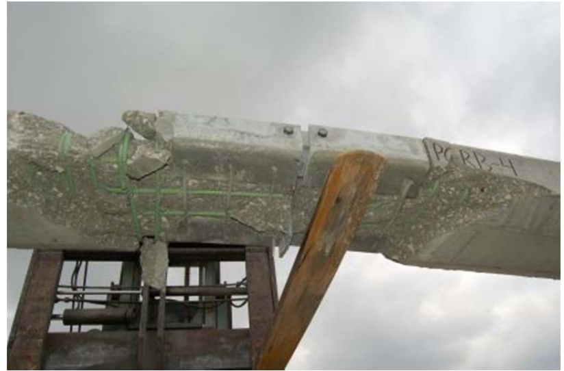
Figure 156. Component Damage – Concrete Damage, Test No. PCRB-4
