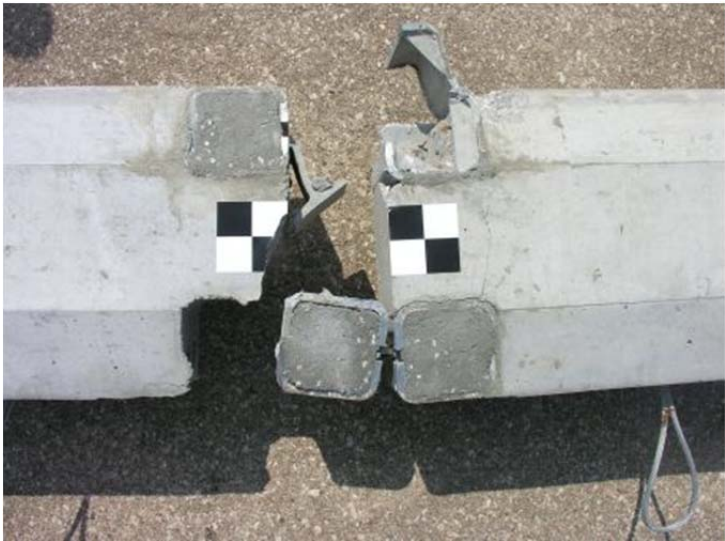
Figure 78. Component Damage, Test No. PCRB-1
