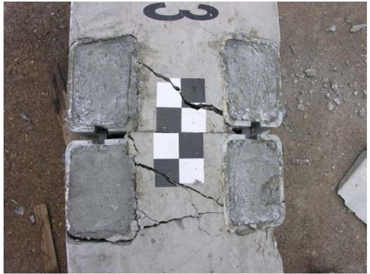
Figure 148. Component Damage, Test No. PCRB-3
