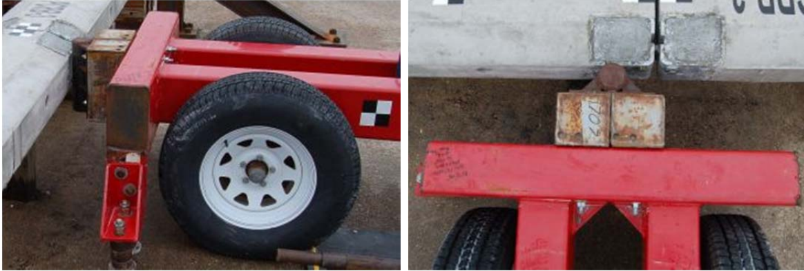
Figure 95. Bogie Impact Head with Steel Tube Blockouts
