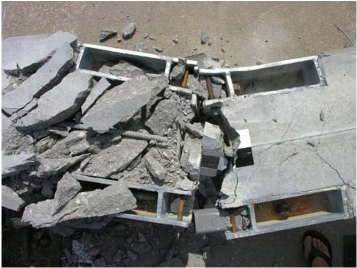
Figure 86. Component Damage, Test No. PCR-B-2
