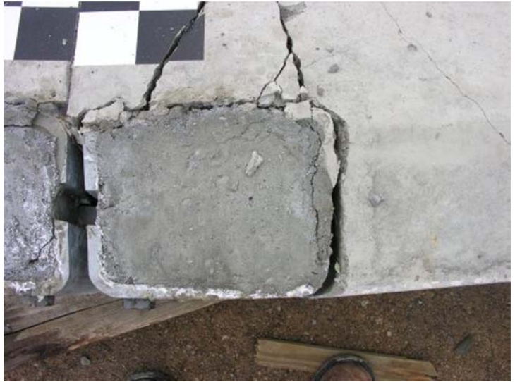
Figure 149. Component Damage – Steel Pockets, Test No. PCRB-3
