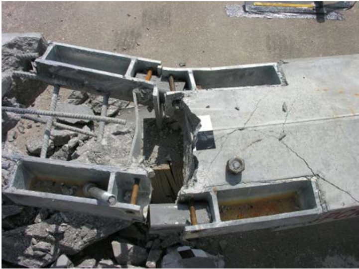
Figure 89. Component Damage – Loose Concrete Removed, Test No. PCRB-2
