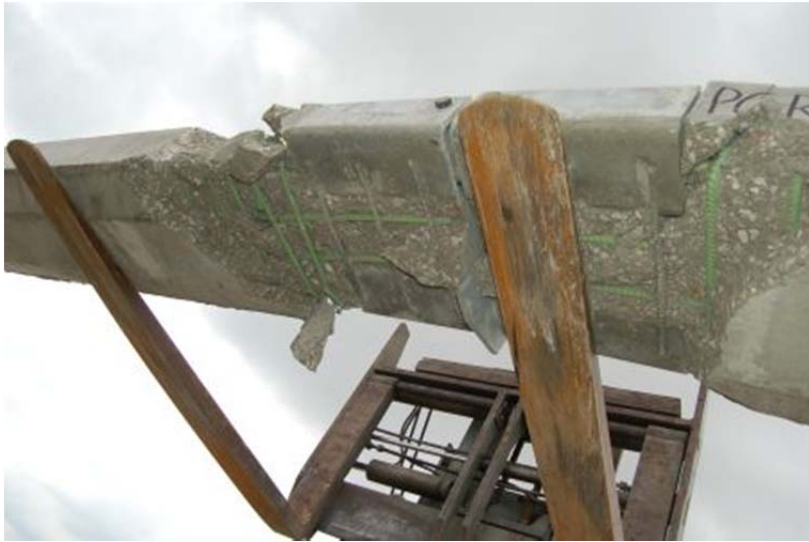
Figure 156. Component Damage – Concrete Damage, Test No. PCRB-4
