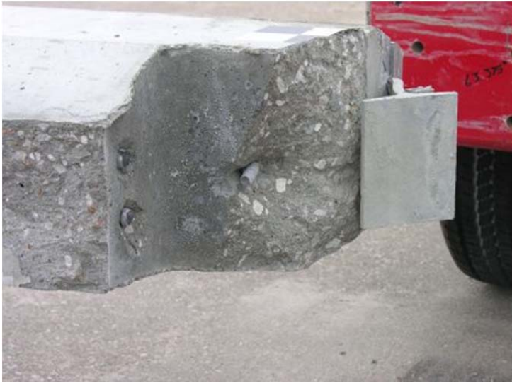
Figure 79. Component Damage – Long Rail Segment, Test No. PCRB-1
