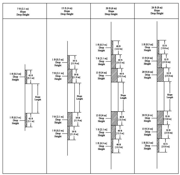
Figure 17. Schematic of Foreslopes in RSAP
