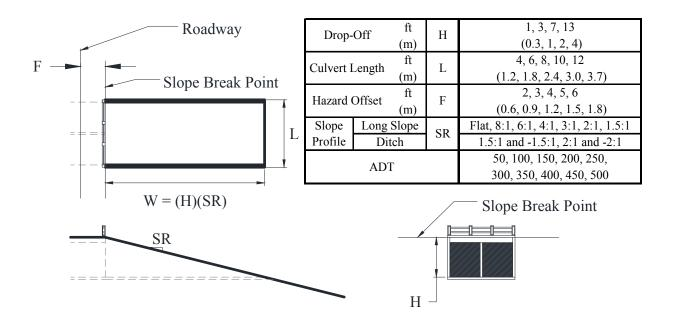
Figure 9. Representative Culvert and Primary Dimensions
