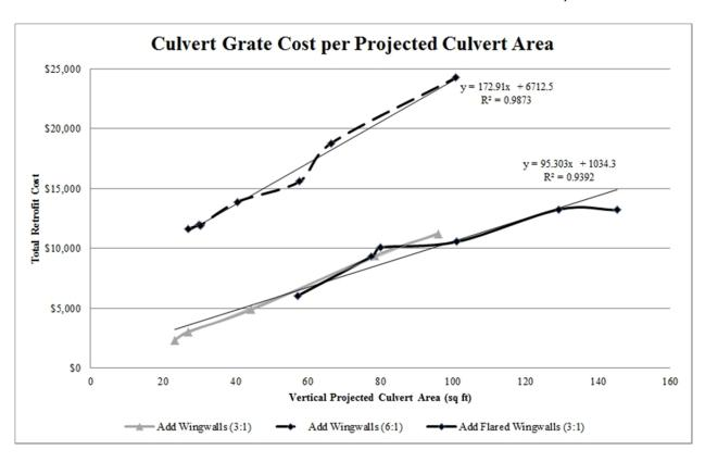
Figure 12. Culvert Grate Cost per Projected Area (KDOT Data and Approximation)
