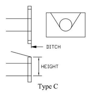
Figure 8. Type-C Culvert Used in RSAP
