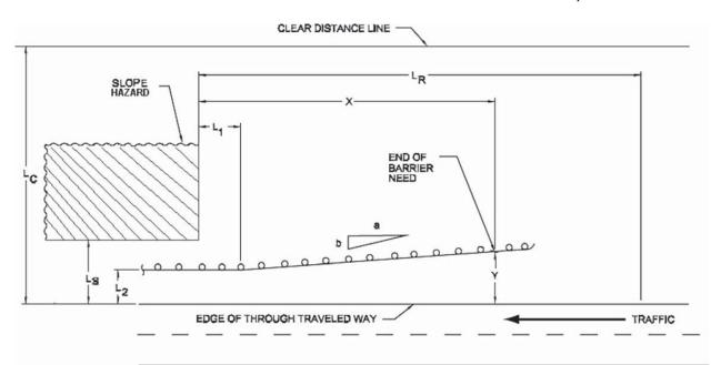
Figure 18. Guardrail Runout Length Schematic
