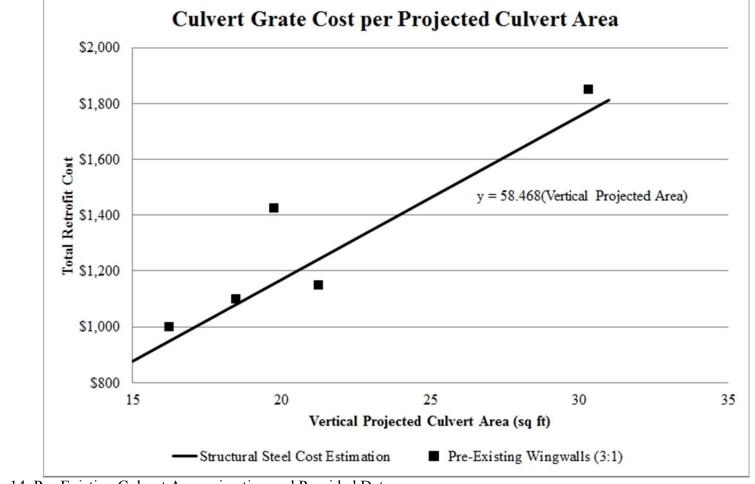
Figure 14. Pre-Existing Culvert Approximation and Provided Data
