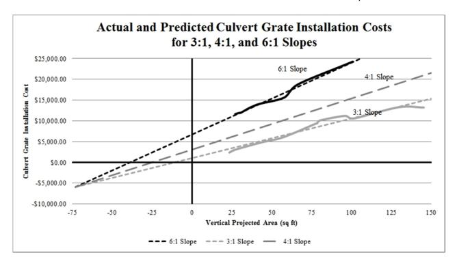
Figure 13. Interpolated Estimate for 4H:1V Culvert Grate Cost with Wingwall Construction
