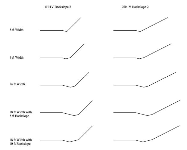
Figure 21. Schematic of Ditches Modeled in RSAP
