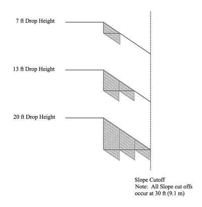
Figure 23. Slope Modeling Dimensions and Simulated Drop-Off Heights
