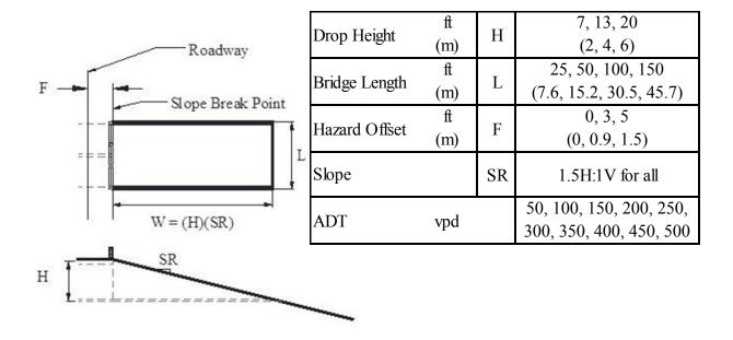
Figure 22. Representative Bridge and Primary Dimensions
