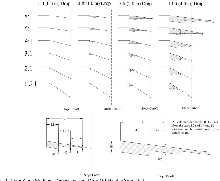
Figure 10. Long Slope Modeling Dimensions and Drop-Off Heights Simulated
