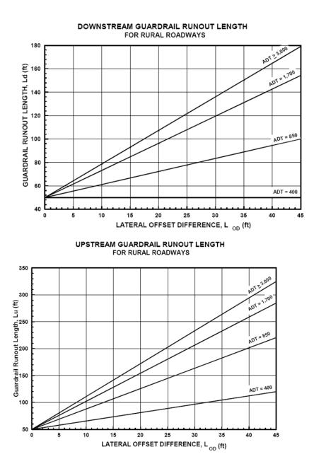
Figure 19. Upstream and Downstream Guardrail Runout Lengths
