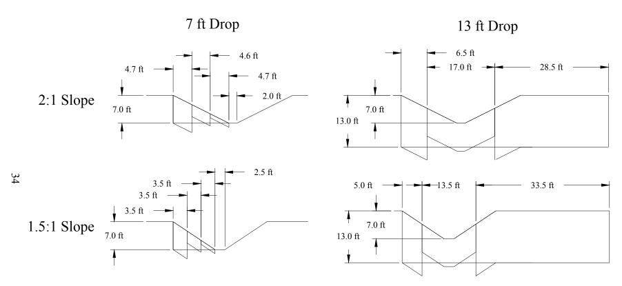
Figure 11. Cross-Sectional Ditch Modeling Dimensions and Drop-Off Heights
