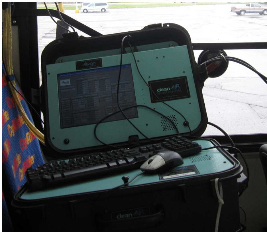
Figure 4-1: PEMS installed on CyRide bus
