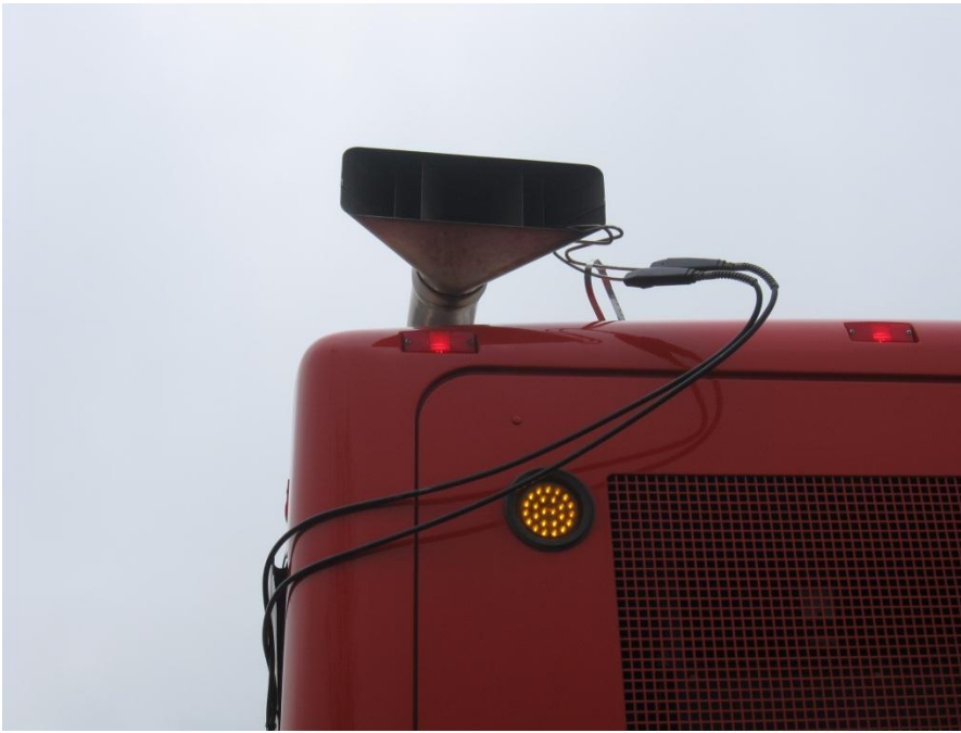
Figure 4-2: PEMS tailpipe probe on CyRide bus
