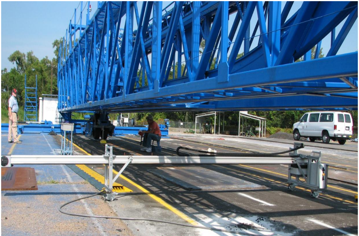
c) Condition assessment under APT
