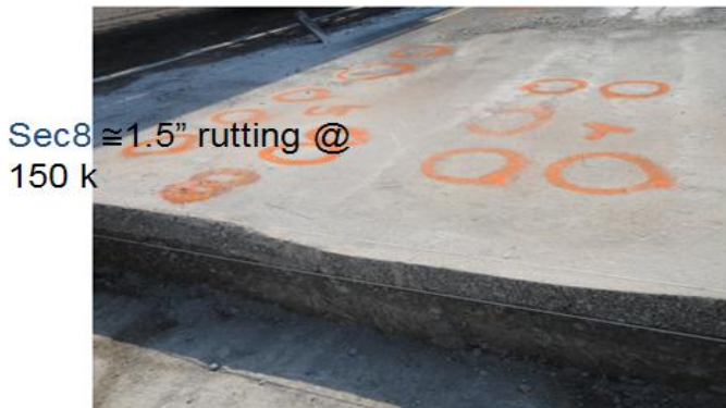
Figure F-8. Base Related Rut Failure of Fatigue Crack Sections.
