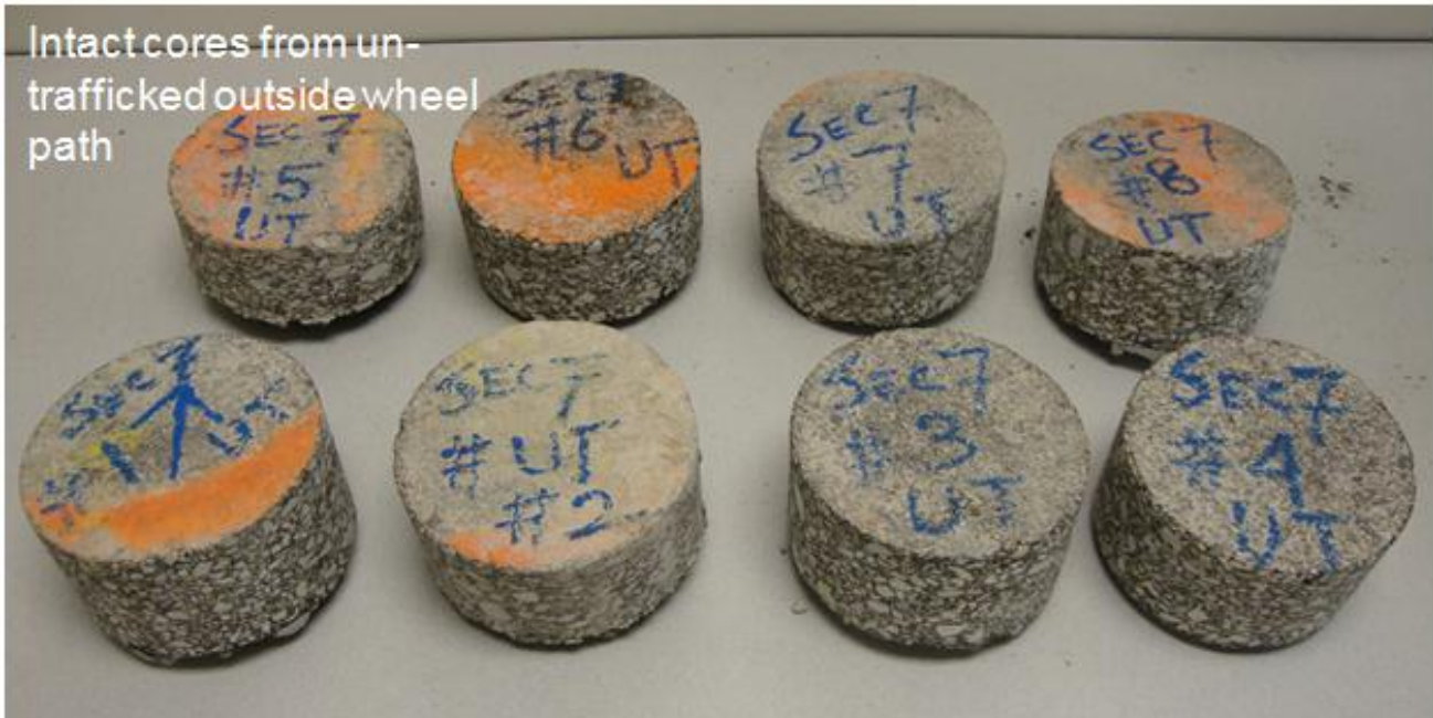
Figure G-1. Cracked and Un-Cracked Cores on Section 7 (5.2% OAC).
