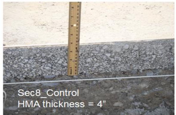
Figure F-8. Base Related Rut Failure of Fatigue Crack Sections.
