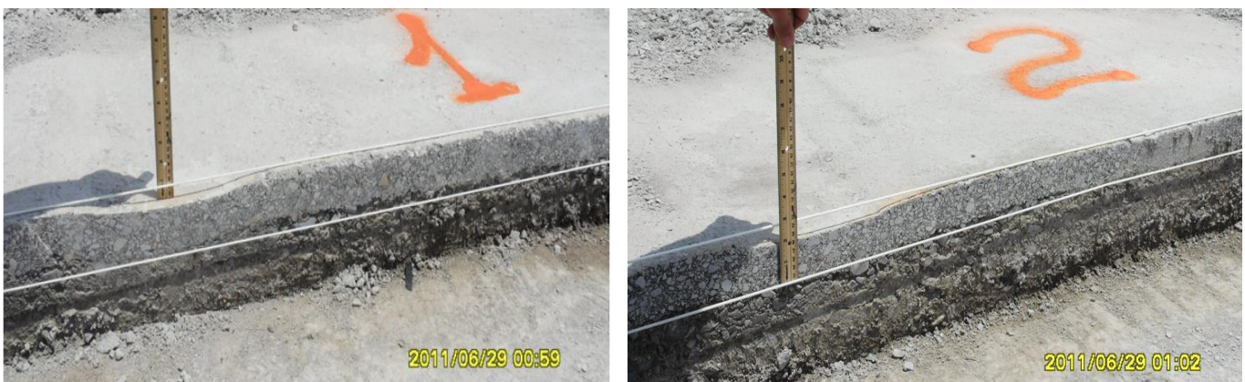
Figure F-2. Trenching and Pictorial Comparison of Rutting.
