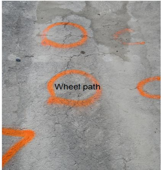
Cores from un-cracked wheel path cracked during the coring process; indication of microdamage/microcracks
