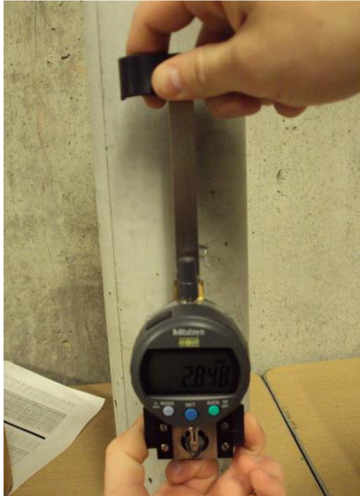
Figure 2.3 – DEMEC Reading Taken on Specimen
