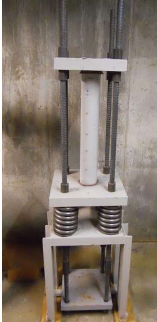
Figure 2.9 - Creep Loading Frame with Specimen
