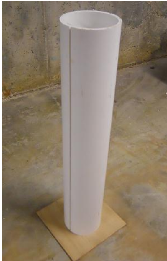
Figure 2.1 - Shrinkage and Creep Form
