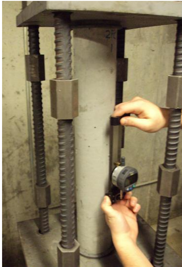
Figure 2.10 - Reading Taken on Creep Specimen
