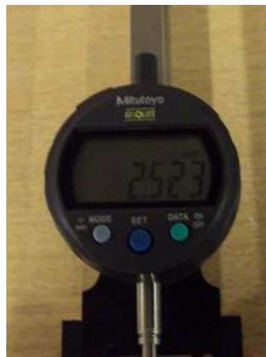
Figure 2.7 - Example DEMEC Gauge Reading
