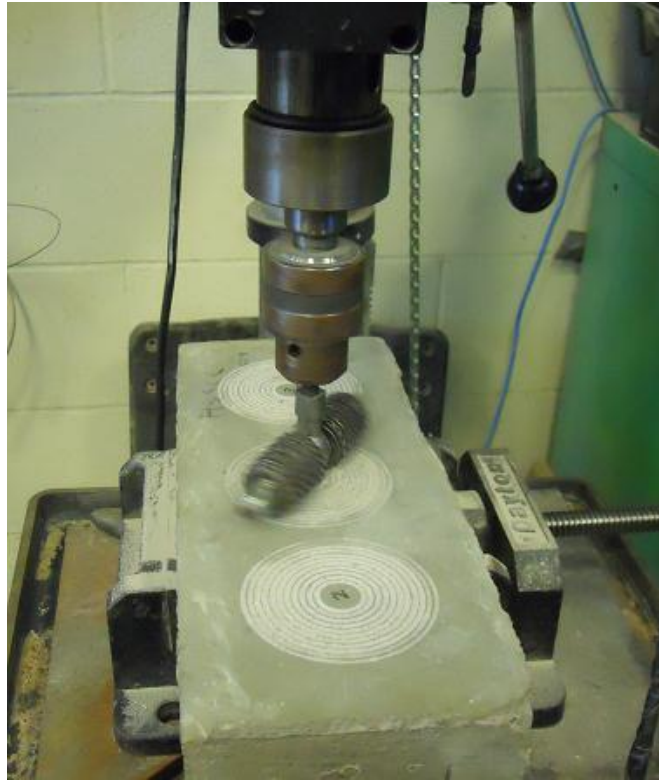
Figure 2.13 - Abrasion Resistance Test in Progress
