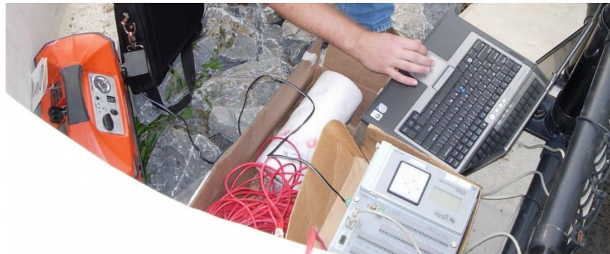
Figure 5-12 Data Acquisition System Monitoring the Strain Gauges During the Live Load Test
