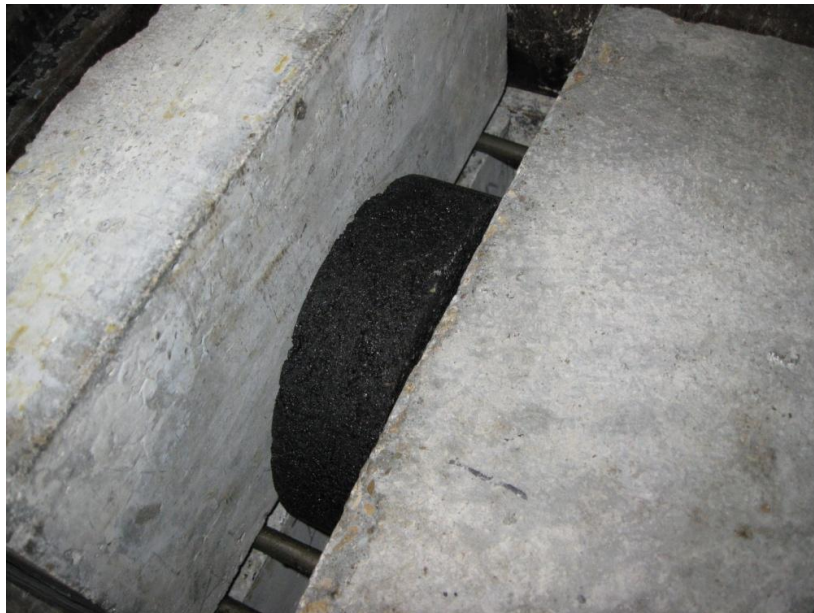
FIGURE 3.16 The HMA Specimen between Lower and Upper Concrete Blocks
