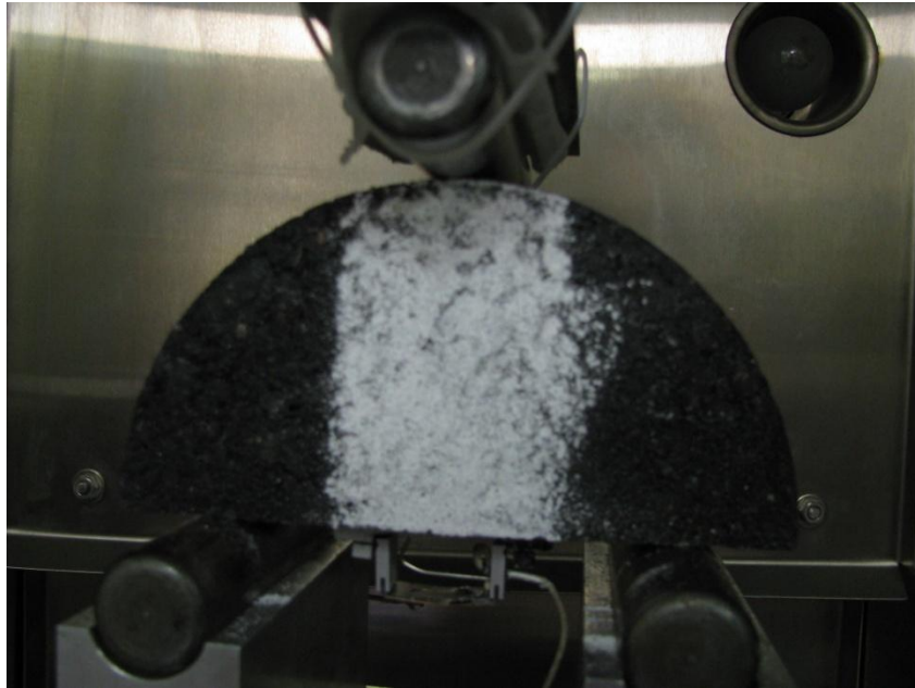
FIGURE 3.18 A Semi-Circular Bend Test with an Extensometer Attached at the Bottom of the Specimen
