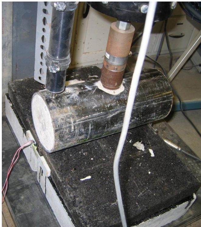
FIGURE 3.8 Picture of the Cylinder Used for Loading with the Displacement Transducer to Measure the Vertical Displacement
