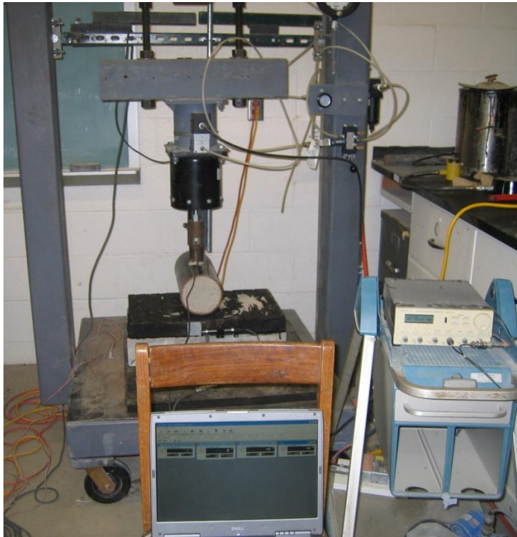
FIGURE 3.10 Picture of the Test Setup Including the Loading System, Controller, and Data Recording System
