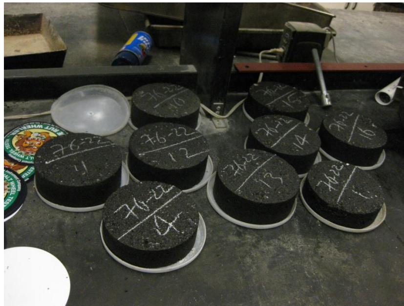
FIGURE 3.14 Prepared HMA Specimens
