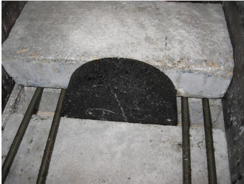
FIGURE 3.15 Concrete Blocks and Steel Bars with an HMA Specimen
