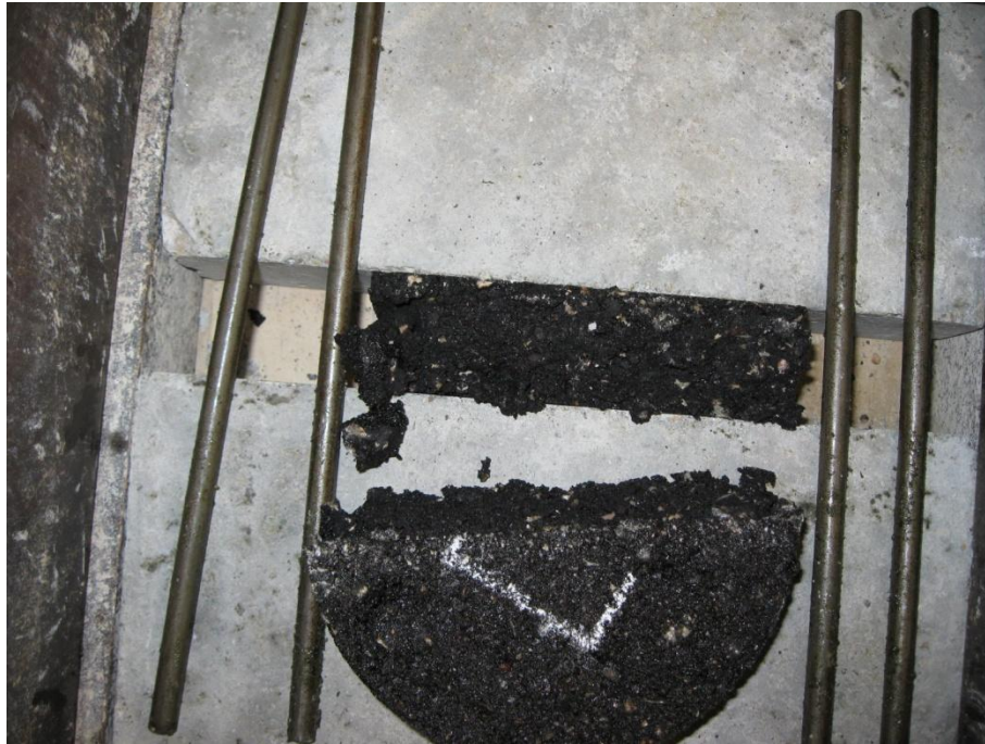
FIGURE 3.17 The Failed Specimen after the Direct Shear Box Test
