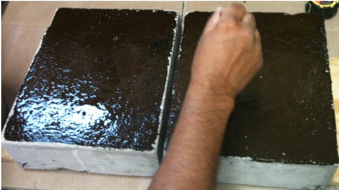
FIGURE 3.6 Application of EBL Tack Coat before Placing an HMA Overlay
