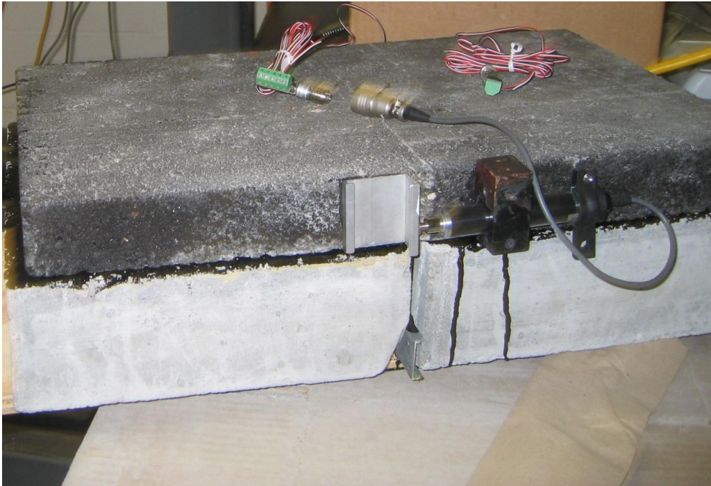
FIGURE 3.7 A Displacement Transducer Affixed on the HMA Overlay
