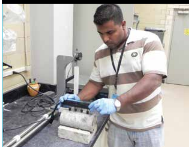
Figure 1. SR test using a four-point Wenner probe.
