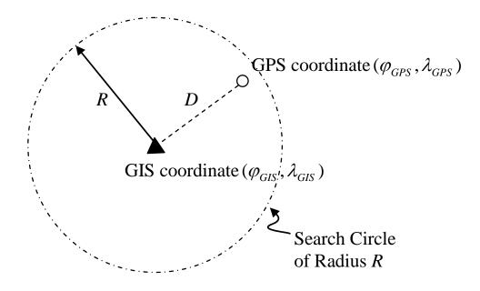
Figure 4. Quantitative Position Validation Procedure
