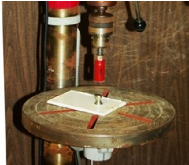
Figure 12. Photo. Drill press to score a test area around a dolly.
