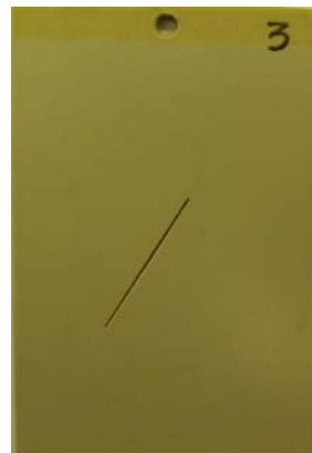
Figure 23. Photo. Progressive changes of IOZ/E/PU—type I in ALT, NW, and NWS.
