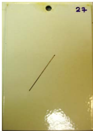
Figure 25. Photo. Progressive changes of MCU/E/F—type I in ALT, NW, and NWS.
