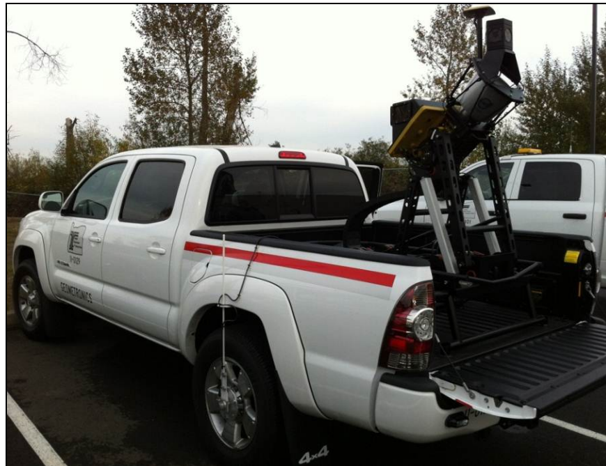
Figure 2.6: Oregon DOT's mobile laser scanner
