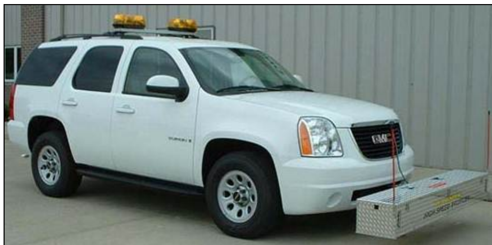
Figure 2.2: High speed inertial profiler ( Ames Engineering 2010 )
