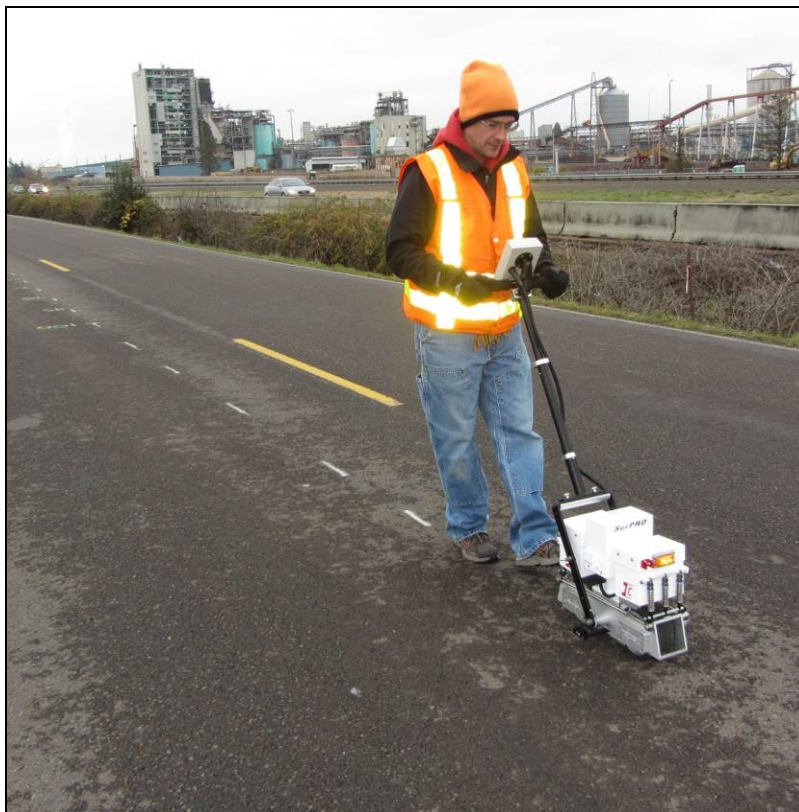
Figure 2.1: SurPRO inclinometer-based profiler operated by ODOT
