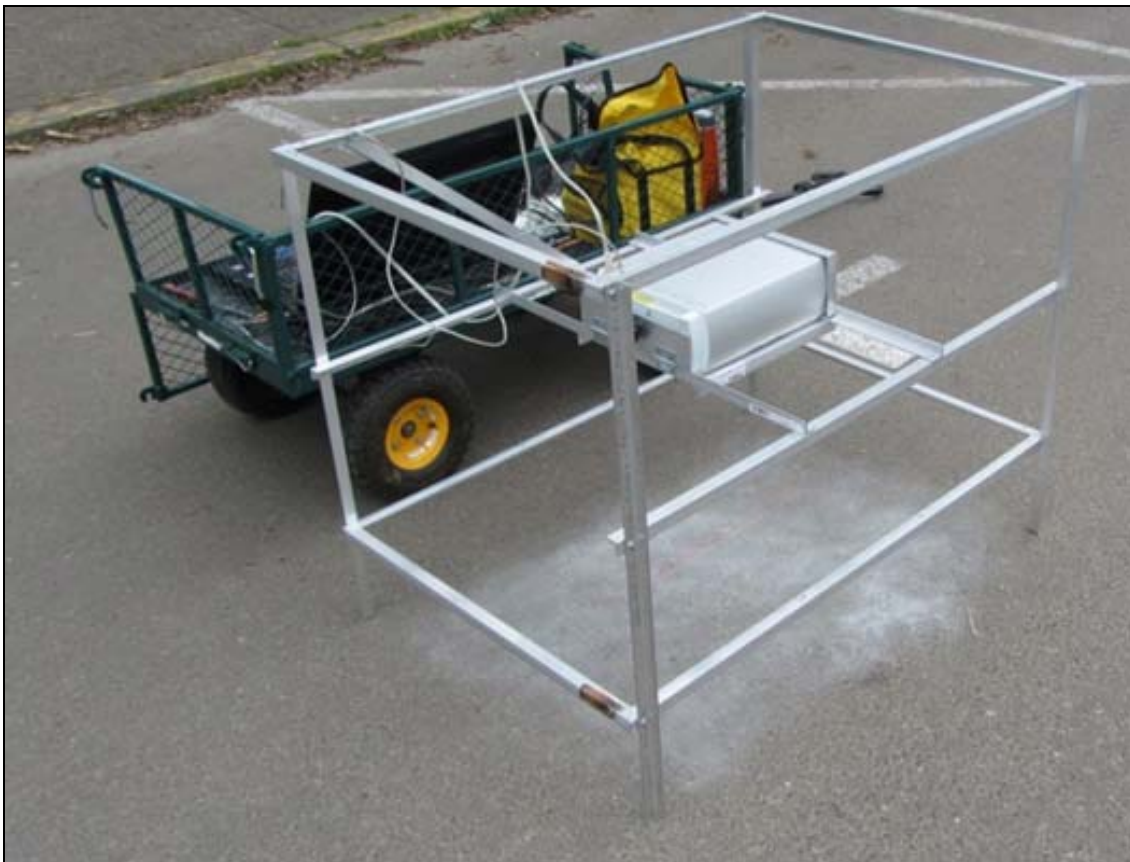
Figure 9.2: Pavement texture analysis scanner set up
