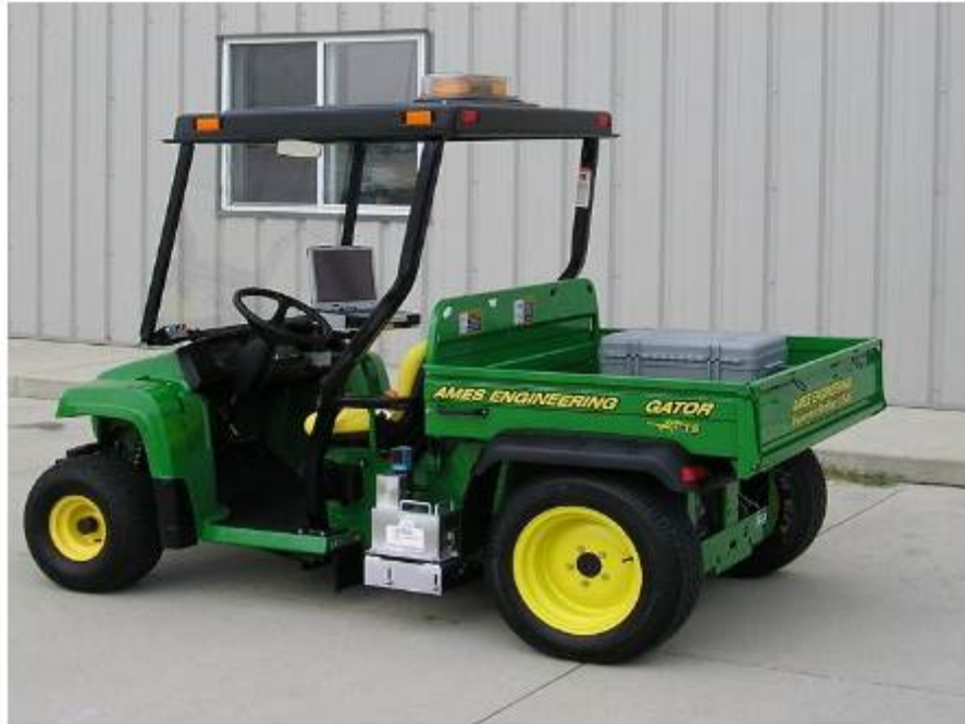
Figure 10.1: Example of a light weight inertial profiler (Ames Engineering 2010)
