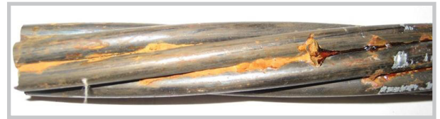
Close-up of Strand in Simulated Gypsum Grout Pore Solution, Specimen G/PC-1
