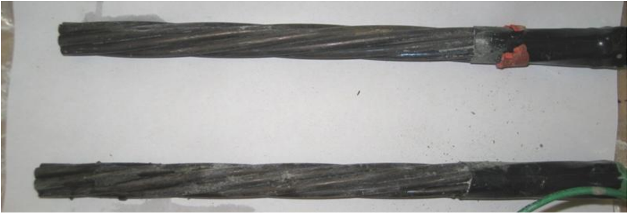
FIGURE 9f Specimen S/PC-2, 30 Weeks, after Removal of Grout. Strand in Sika Grout (Top) and Portland Cement Grout (Bottom)
