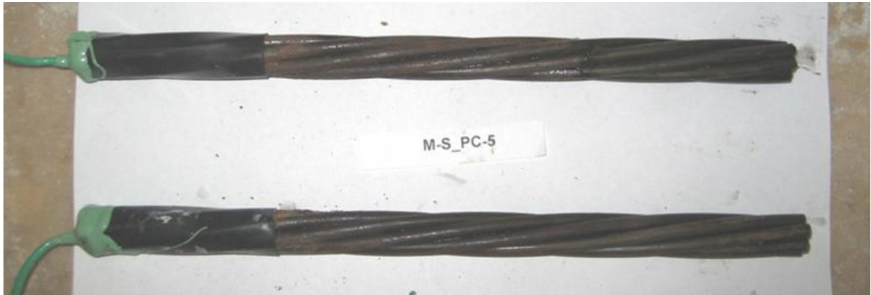
FIGURE 6g Specimen S/PC-5, 15 Weeks. Strand in Simulated Sika Grout Pore Solution (Top) and Simulated Portland Cement Grout Pore Solution (Bottom)
