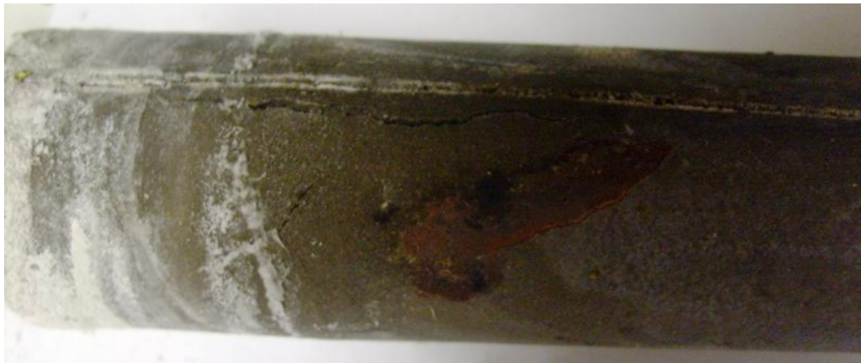
FIGURE 9b Specimen G/SFG-2, 15 Weeks. Close-up on Strand in Gypsum Grout
