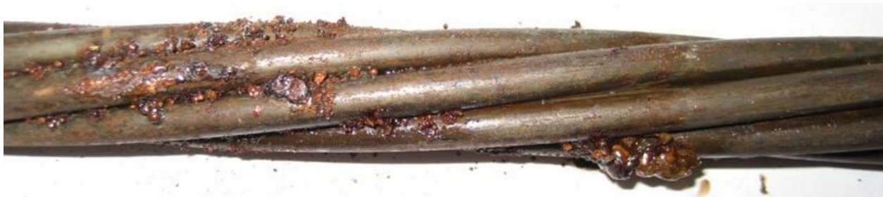
FIGURE 15e Specimen SFG/PC with Salt-4, 15 Weeks. Close-up of Strand in Simulated Sika with FerroGard Pore Solution with 3% NaCl
