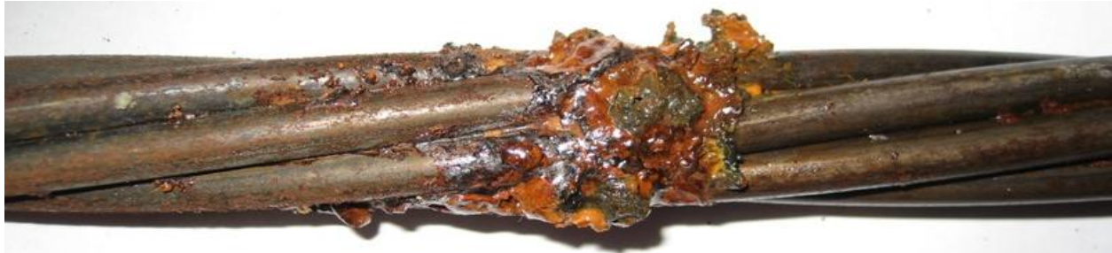
FIGURE 15b Specimen NA/PC with Salt-3, 15 Weeks. Close-up of Strand in Simulated NA Pore Solution with 3% NaCl
