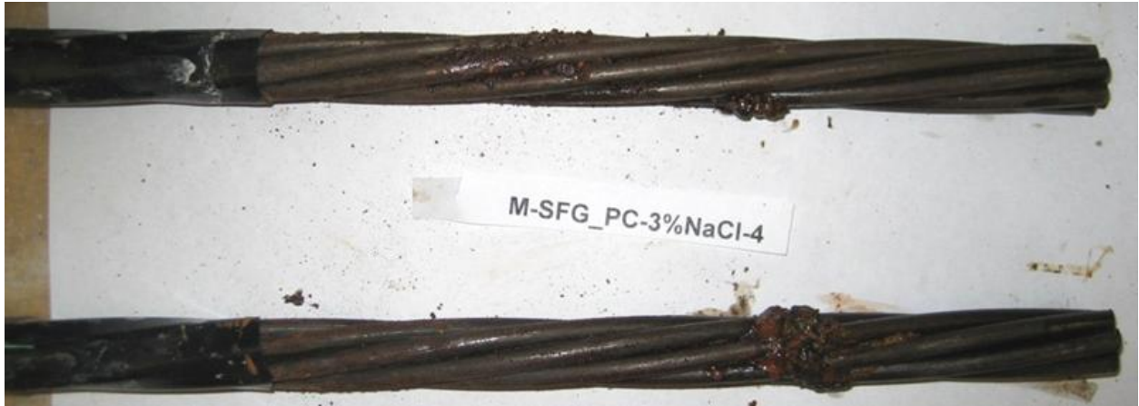
FIGURE 15d Specimen SFG/PC with Salt-4, 15 Weeks. Strand in Simulated Sika with FerroGard (Top) and Portland Cement Pore (Bottom) Solutions with 3% NaCl
