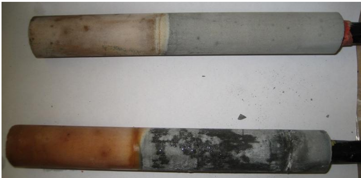
FIGURE 9e Specimen S/PC-2, 30 Weeks. Strand in Sika Grout (Top) and Portland Cement Grout (Bottom)
