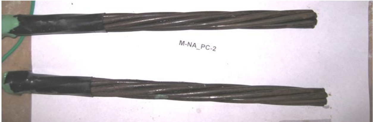
FIGURE 6f Specimen NA/PC-2, 15 Weeks. Strand in Simulated NA Grout Pore Solution (Top) and Simulated Portland Cement Grout Pore Solution (Bottom)
