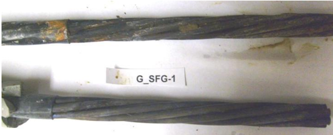
FIGURE 9c Specimen G/SFG-1, 15 Weeks, after Removal of Grout. Strand in Gypsum Grout (Top) and Sika with FerroGard Grout (Bottom)
