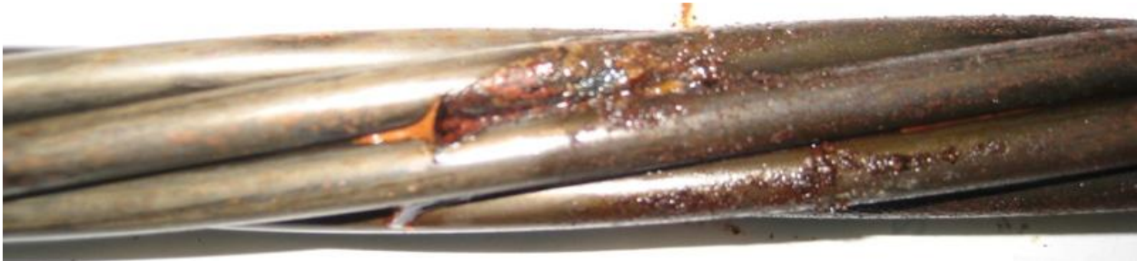
FIGURE 6b Close-up of Strand in Simulated Gypsum Grout Pore Solution, Specimen G/SFG-3
