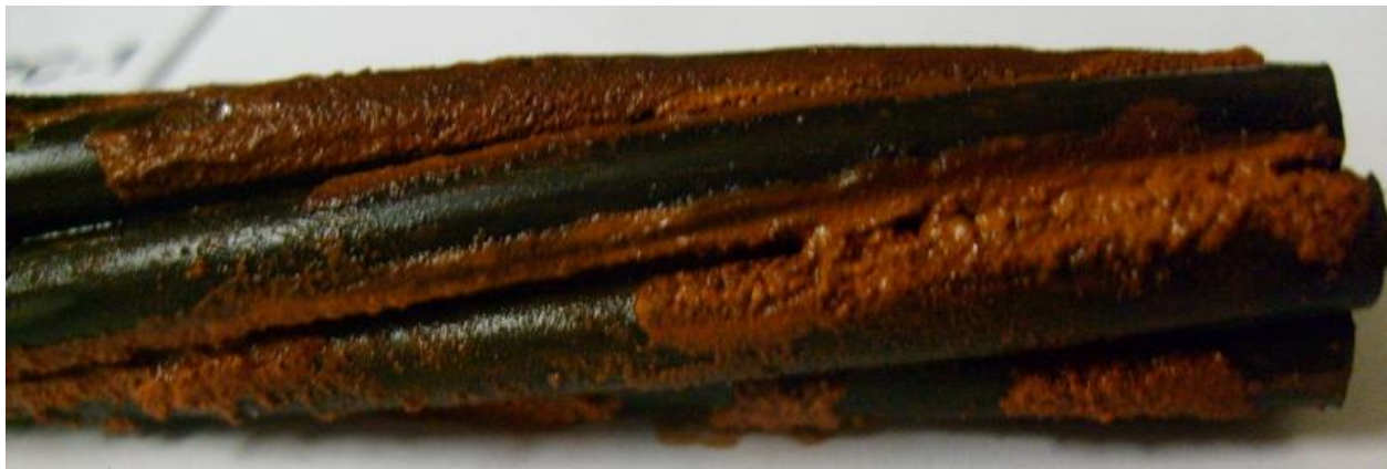
FIGURE 12b Specimen H 2 O/PC-1, 15 Weeks. Close-up of Strand in Deionized Water
