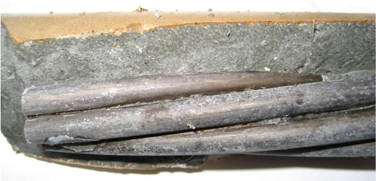
FIGURE 9i Staining below the Waterline on Grout-Wrapped Specimens
