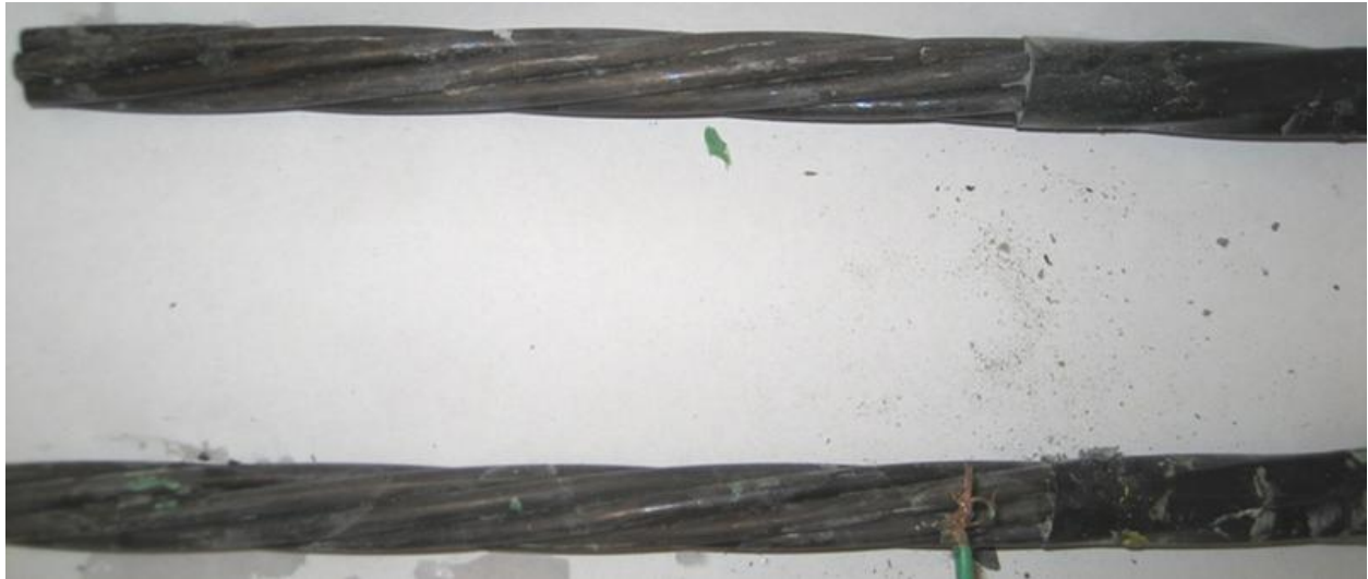
FIGURE 9h Specimen SFG/PC-1, 30 Weeks, after Removal of Grout. Strand in Sika with FerroGard Grout (Top) and Portland Cement Grout (Bottom)
