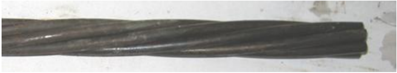
FIGURE 6i Specimen SFG/PC-6, 15 Weeks. Strand in Simulated Sika with FerroGard Grout Pore Solution Showing No Significant Corrosion Products
