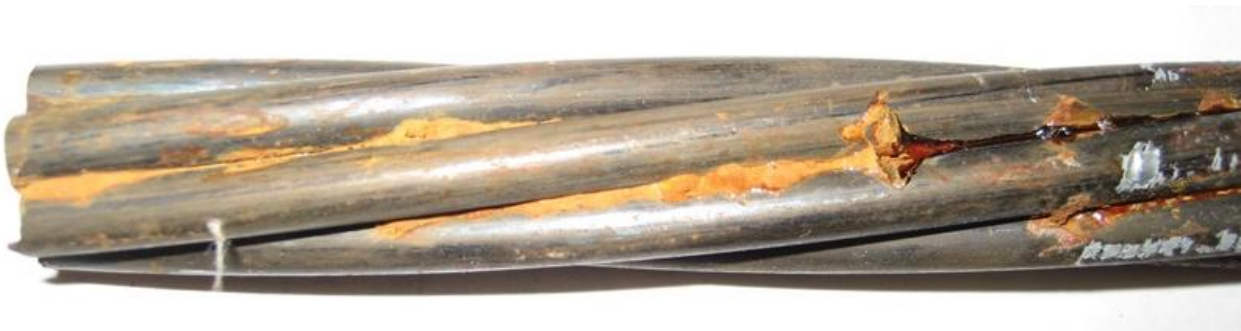
FIGURE 6d Close-up of Strand in Simulated Gypsum Grout Pore Solution, Specimen G/PC-1
