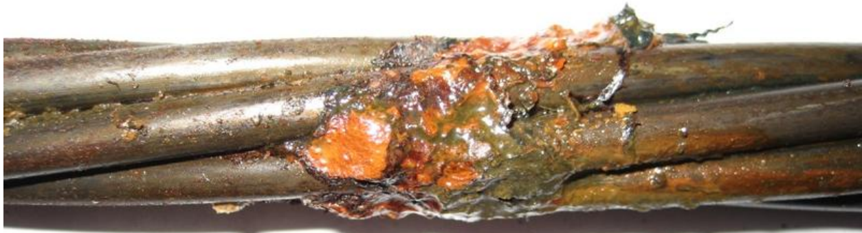
FIGURE 15c Specimen NA/PC with Salt-3, 15 Weeks. Close-up of Strand in Simulated Portland Cement Pore Solution with 3% NaCl
