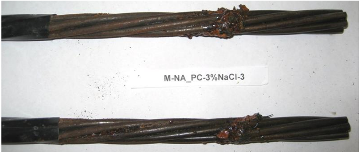
FIGURE 15a Specimen NA/PC with Salt-3, 15 Weeks. Strand in Simulated NA (Top) and Portland Cement Pore (Bottom) Solutions with 3% NaCl
