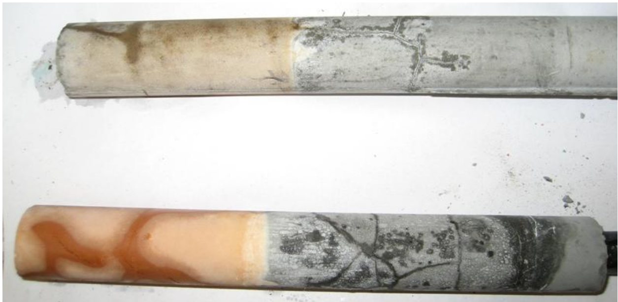
FIGURE 9g Specimen SFG/PC-1, 30 Weeks. Strand in Sika with FerroGard Grout (top) and Portland Cement Grout (Bottom)
