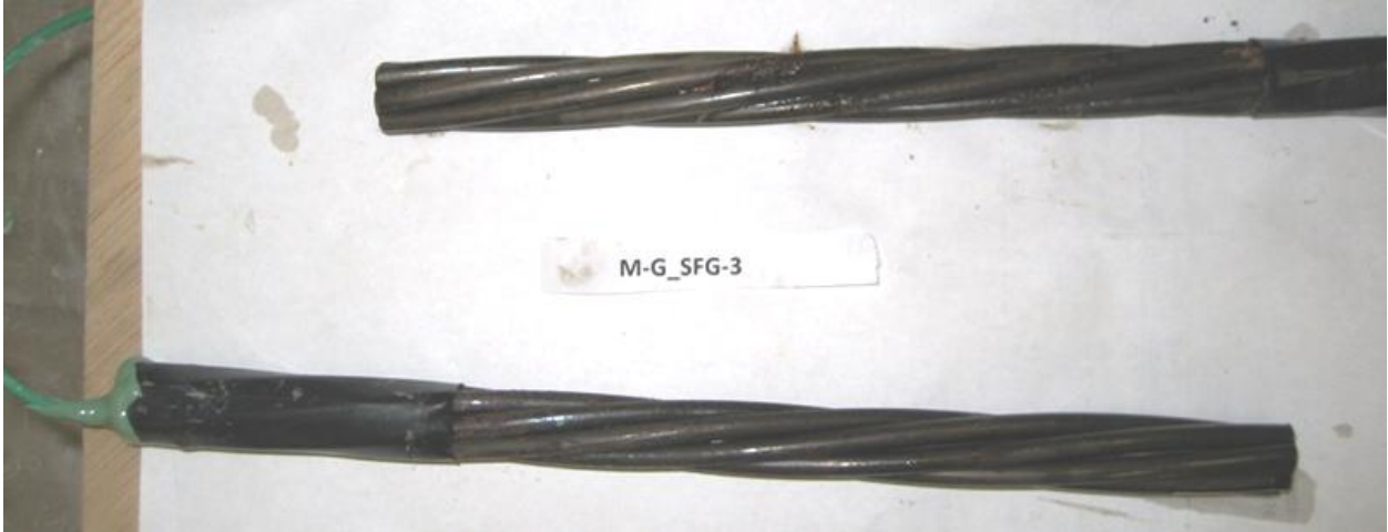
FIGURE 6a Specimen G/SFG-3, 15 Weeks. Strand in Simulated Gypsum Pore Solution (Top) and Simulated Sika with FerroGard Pore Solution (Bottom)
