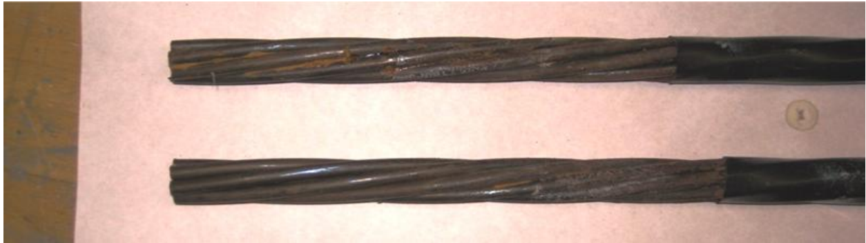
FIGURE 6c Specimen G/PC-1, 15 Weeks. Strand in Simulated Gypsum Grout Pore Solution (Top) and Simulated Portland Cement Grout Pore Solution (Bottom)
