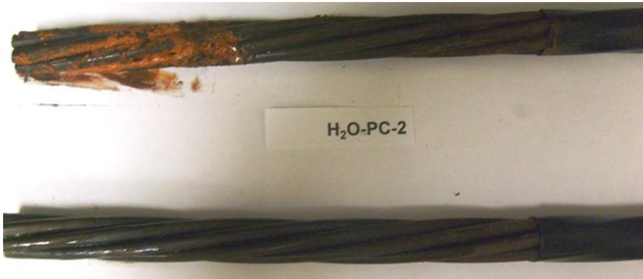
FIGURE 12a Specimen H 2 O/PC-1, 15 Weeks. Strand in Deionized Water (Top) and Simulated Portland Cement Pore Solution (Bottom)
