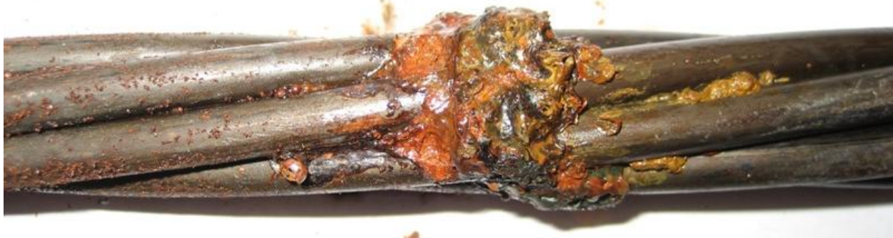
FIGURE 15f Specimen SFG/PC with Salt-4, 15 Weeks. Close-up of Strand in Simulated Portland Cement Pore Solution with 3% NaCl
