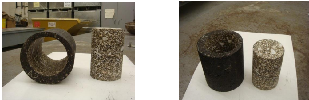
Figure 3.14 A specimen cored and sawed from the gyratory compacted sample
