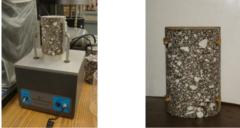
Figure 3.15 A device used to place the mounting studs for LVDTs
