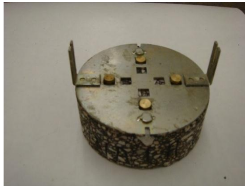
Figure 3.21 Gauge-point mounting device
