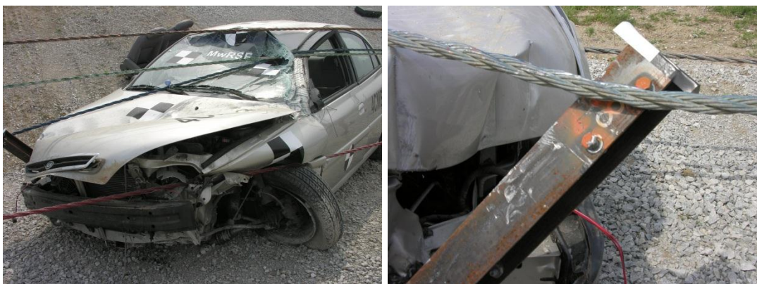
Figure 2. 1100C Full-Scale Crash Test Failure
