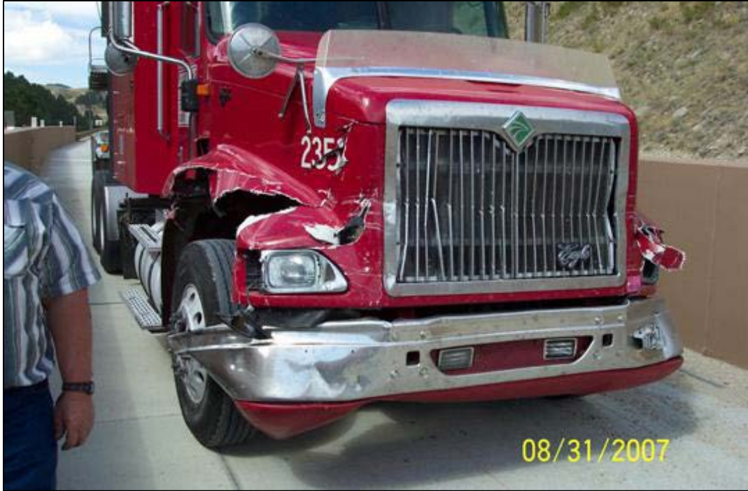
Figure 4.6 The front of the truck after stopping, showing the relatively minimal damage to the vehicle.
