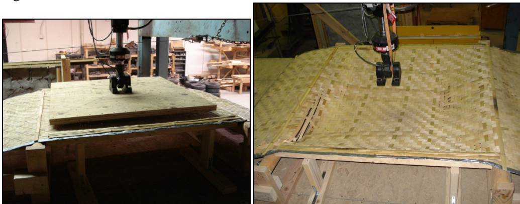
Figure 4.7 The puncture shear testing of a woven bamboo mat.
