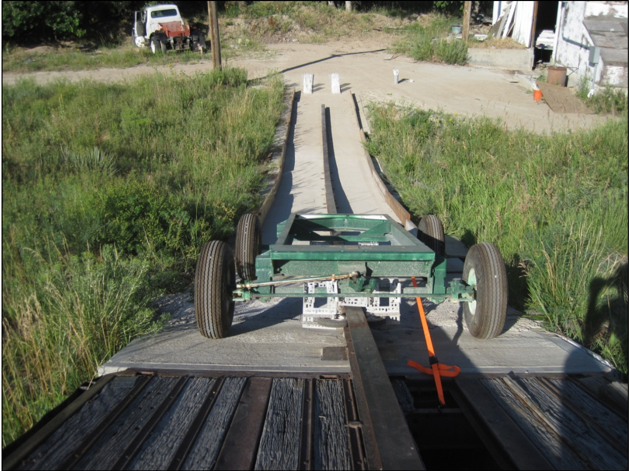
Figure 3.4 CSU vehicle testing ramp. The change in elevation allows a vehicle speed of up to 25 mph to be achieved with little effort, providing a reasonable amount of kinetic energy that needs to be absorbed by the flexible ramp system. The two white blocks at the bottom of the ramp (after the center rail, which guides the vehicle, ends) are in fact the array of fiberglass rods.
