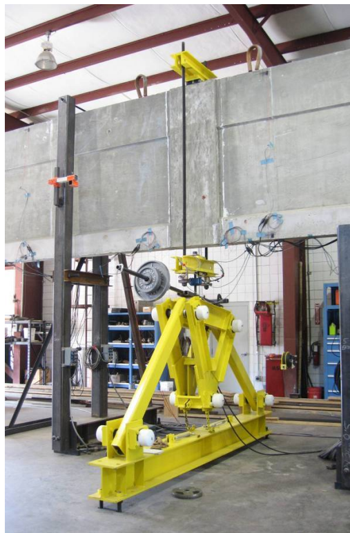
Figure 11.9. UF/FDOT gravity load simulator and load frame in testing position
