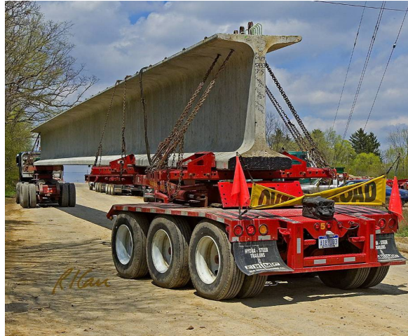
Figure 9.4. Transport of bridge girders (photo courtesy of Dr. Robert I. Carr)
