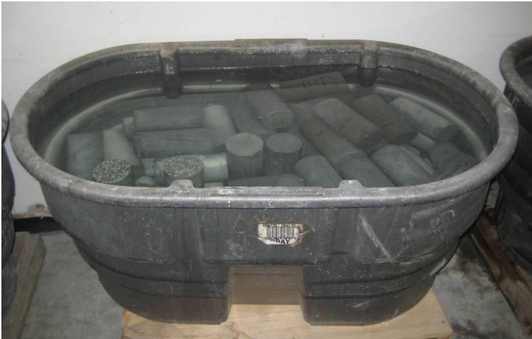
Figure 10.21. Moist-cured cylinders submerged in a tank of lime water
