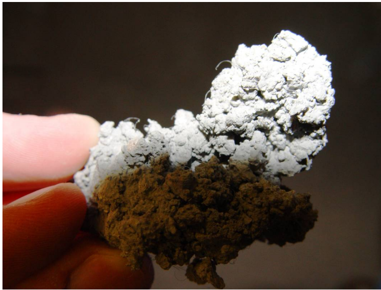
Figure 10.14. Concrete used in closure strip and end block concrete mix, showing presence of Propex Fibermesh® 150 reinforcing fibers
