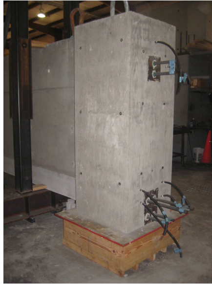
Figure 10.19. End block after removal of formwork
