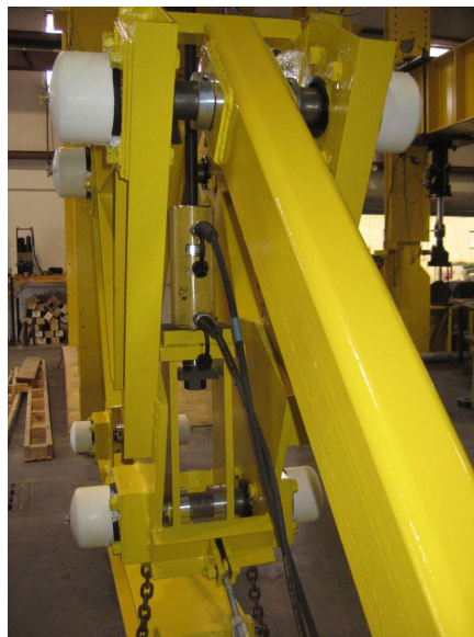
Figure 11.6. Hydraulic jack connection to simulator center pin
