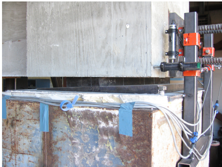
Figure 12.5. Beveled plate and bearing pad positioned between end block and end support
