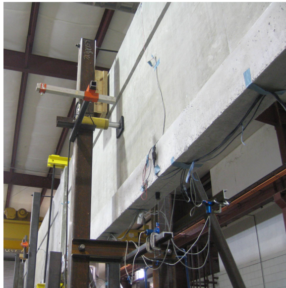
Figure 12.9. Jack used to straighten test girder
