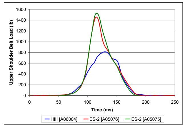
Figure 6. Comparison of FAA Hybrid-III and ES-2 Shoulder Belt Tension
