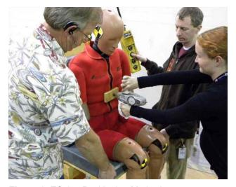
Figure 2. ES-2re Positioning Method
