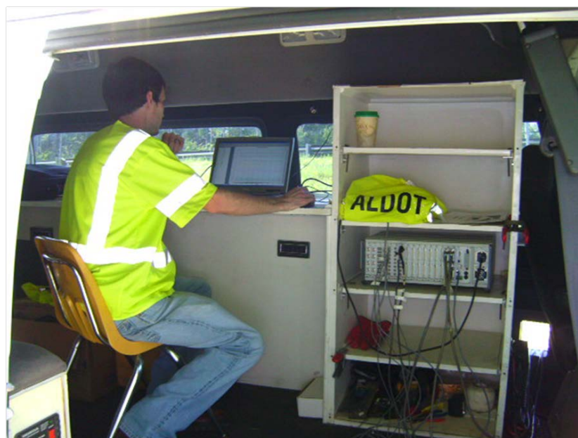
Figure 5-15. The data acquisition system inside the ALDOT van parked next to the structure
