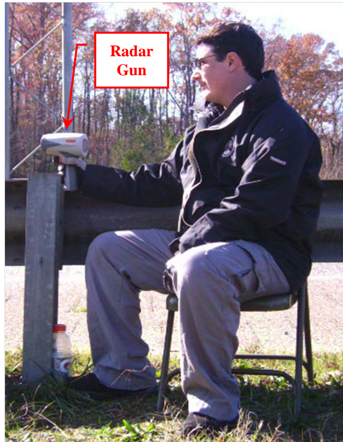
Figure 6-1. Radar speed gun used to measure the speed of passing semi-trailers
