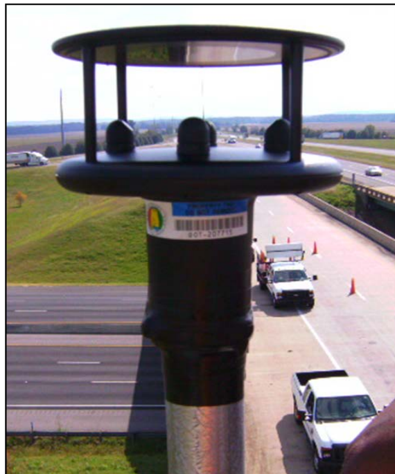
Figure 5-6. WindSonic ultra-sonic wind and direction sensor used to measure the wind dynamic behavior
