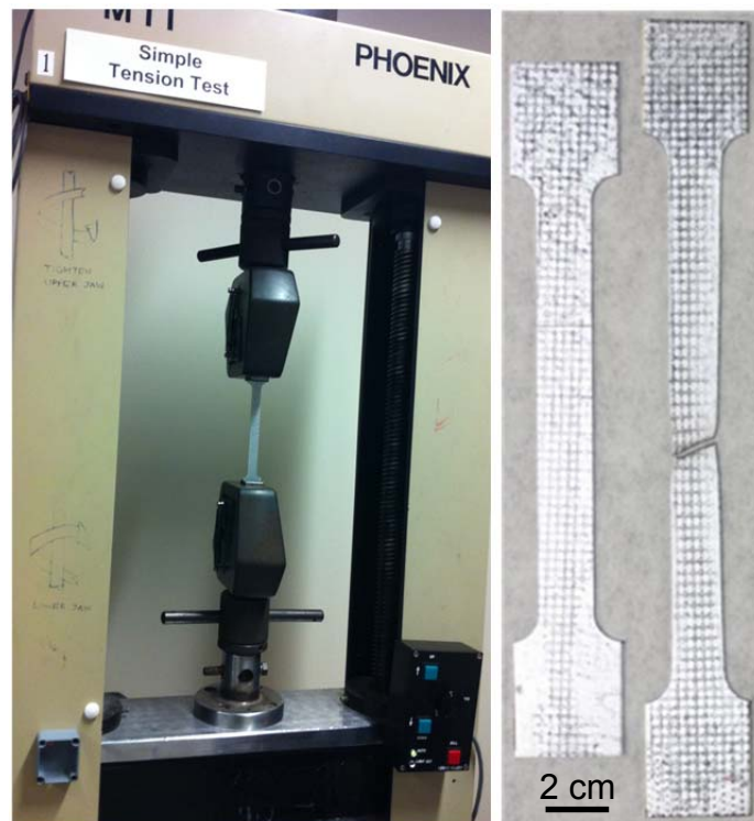
Figure 9: specimens before and after tensile test.
