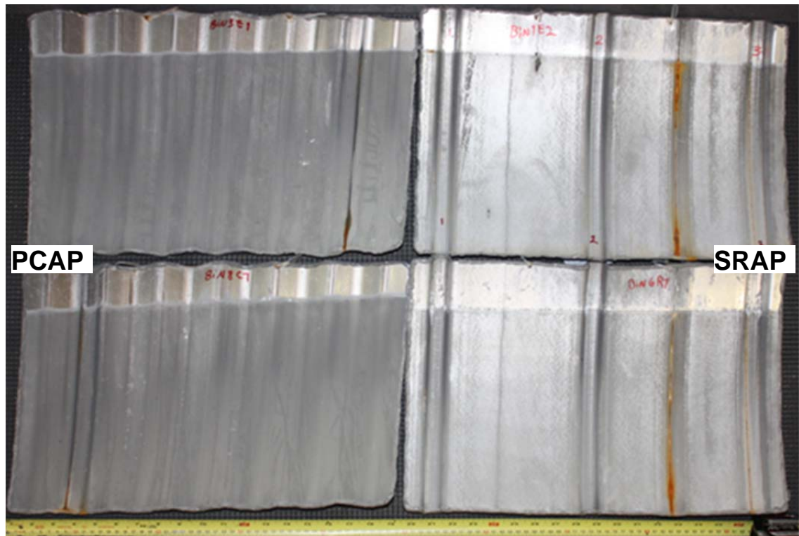
Figure 17 : PCAP and SRAP specimens in S solution [Top] and S + solution [Bottom] after ~700 days of exposure.
