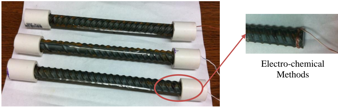
Figure 5.3 Steel rebars' preparation for corrosion tests
