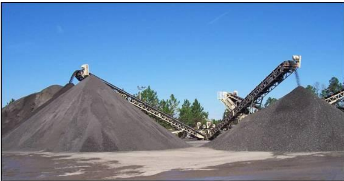
Figure 4.3 RAP Fractionation into Coarse FRAP (right) and Fine FRAP (left)
