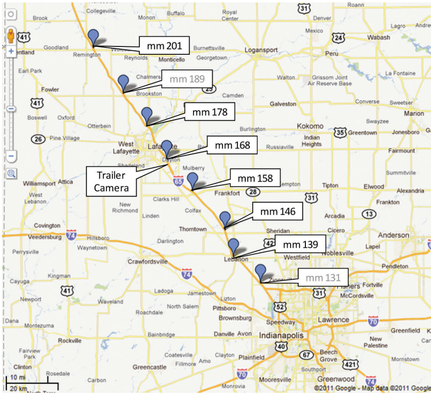
Figure 4.1 Location of portable Bluetooth data collection points on I-65 in Indiana.
