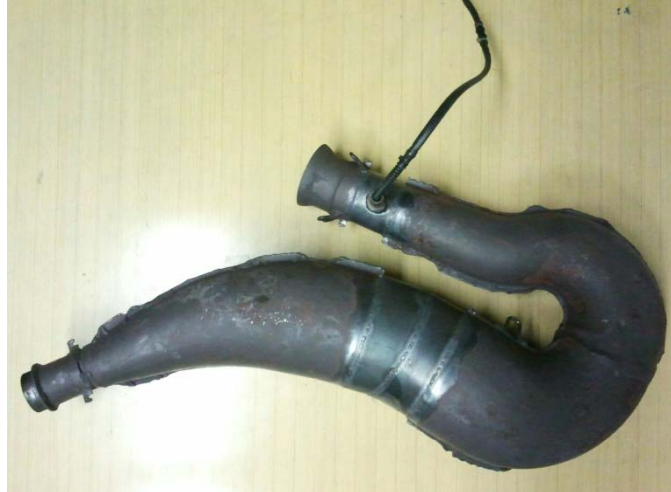
Figure 4: Completed tuned pipe used in the 2012 CSC competition
