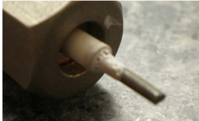
Figure 12: Ceramic adhesive paint used to seal the electrical lead at the top of the CPT.
