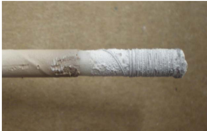
Figure 10: Boron Nitride coating after electrical heating of platinum wire.
