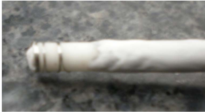
Figure 11: Ceramic core and platinum wire with alumina ceramic paint covering the right side of the core.
