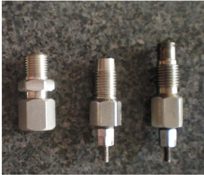
Figure 9: Comparison of feed-throughs. Left to right: MPG-125, in-house feed-through, and original design.
