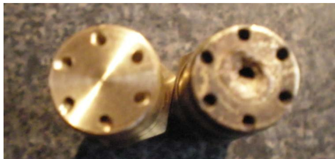
Figure 7: Newly machined prechamber body is on the left, and the original disassembled prechamber body is on the right.
