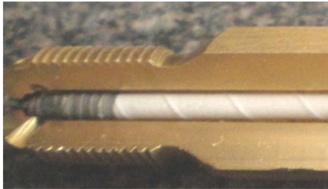
Figure 4: Ground wire on bottom of ceramic core.
