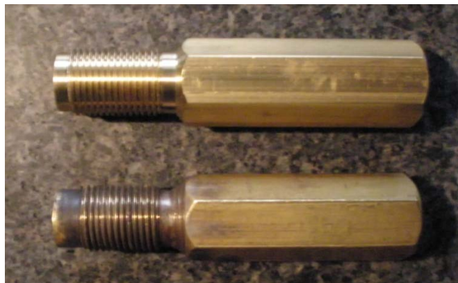
Figure 5: New designed prechamber shown on top, with an original prechamber pictured below.
