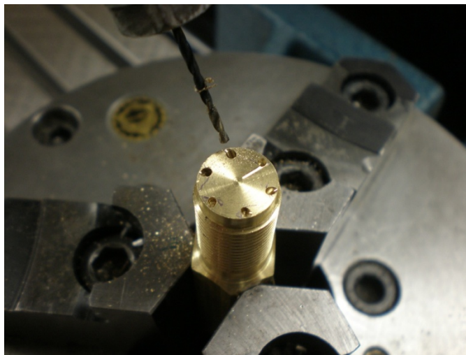
Figure 6: Mounting fixture for drilling angled holes in the tip of the prechamber.
