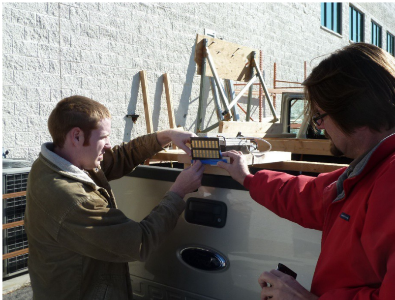
Figure 4. X-band radar mounted on tailgate of truck. Antenna is looking down at approximately 45 degrees.
