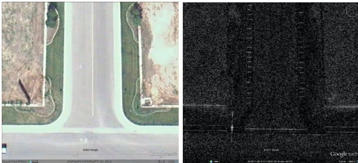
Figure 11. Google Earth image (left) and Ku-band SAR image (right) of roads and sidewalks in front of ImSAR. Cracks running left/right (the same direction as the flight direction) are readily seen.
