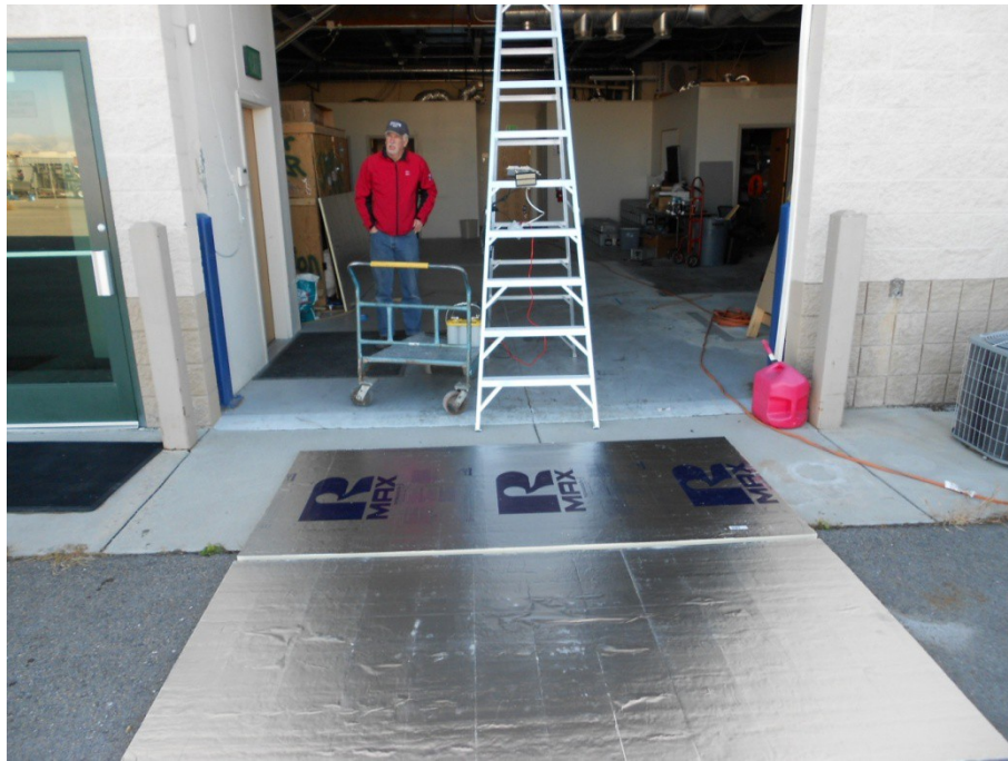
Figure 2. Configuration of preliminary experiments in which metallized foam sheets were illuminated by ladder-mounted X-band radar.
