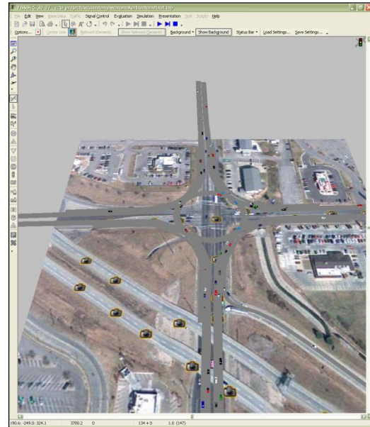
FIGURE 4.13b Still of VISSIM Simulation— Roundabout
