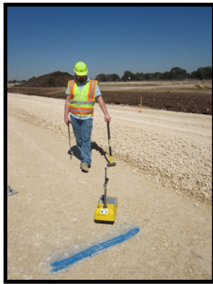
Figure 2.13. Collecting Nuclear Density Readings on US 183.
