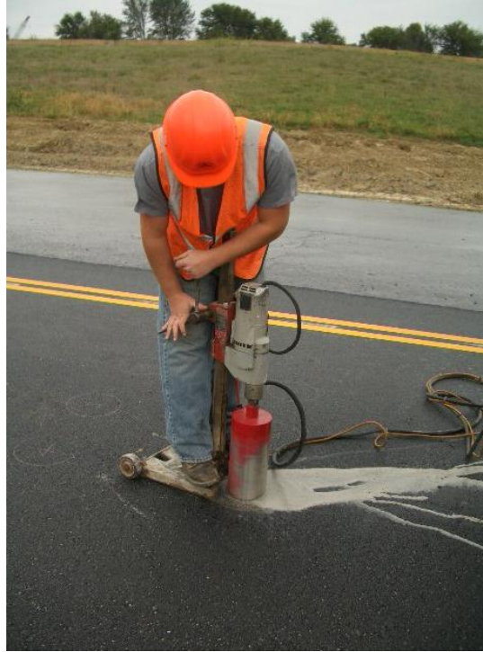
Figure 3.4 Taking Cores for PQI Calibration
