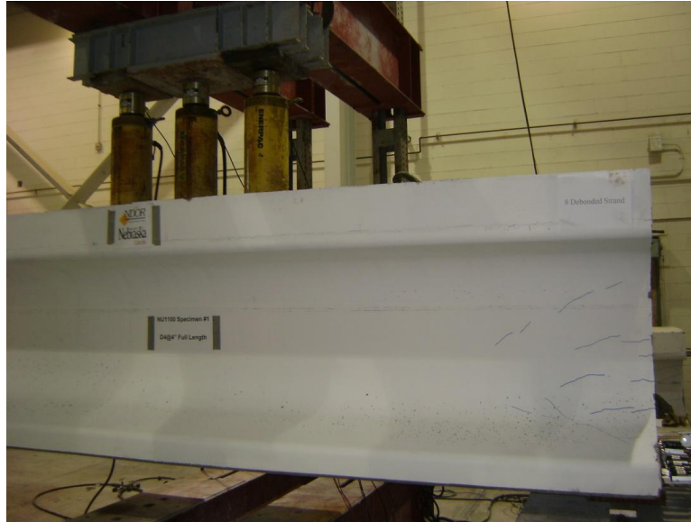
Figure 49 NU1100 Vertical Shear Test Setup
