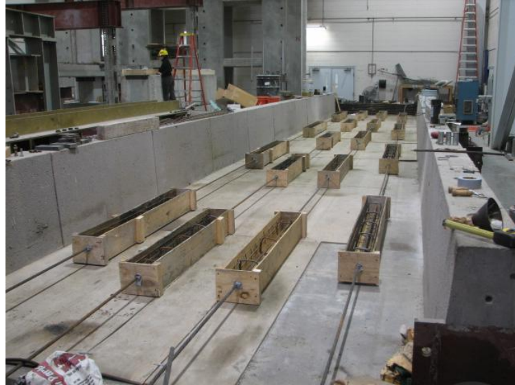
Figure 19 Forms of the Pullout Specimens
