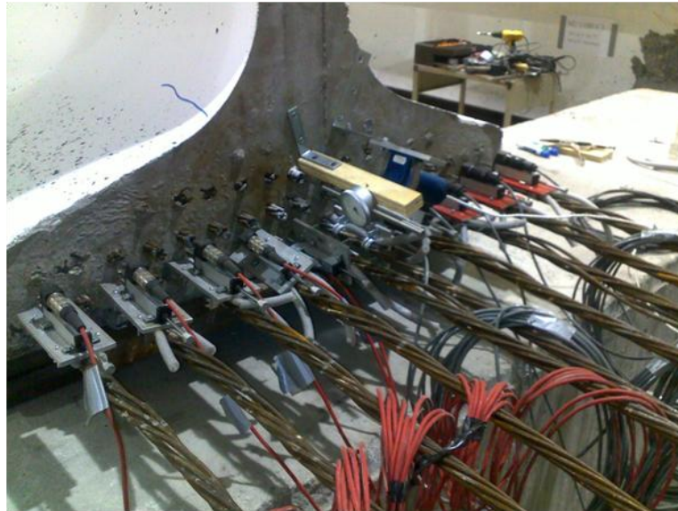
Figure 32 Development Length Test Strand Instrumentation
