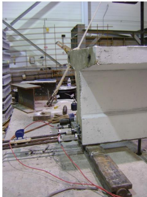
Figure 44 Shear Test Strand Instrumentation
