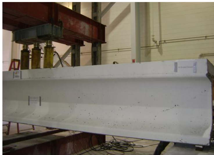
Figure 31 NU1100 Development Length Test Setup
