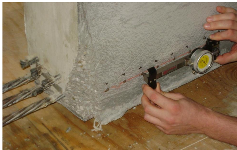
Figure 11 Measuring Strain in Concrete for Transfer Length Estimation
