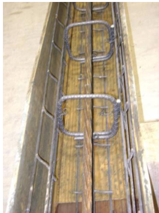
Figure 20 Specimen Strand Confinement
