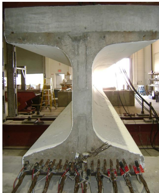
Figure 4.17 Shear test strand instrumentation
