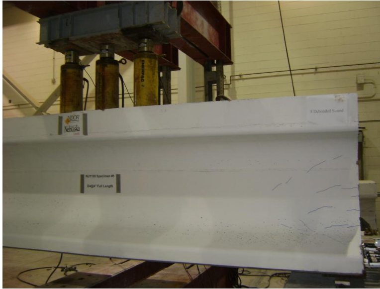
Figure 4.16 NU1100 vertical shear test setup
