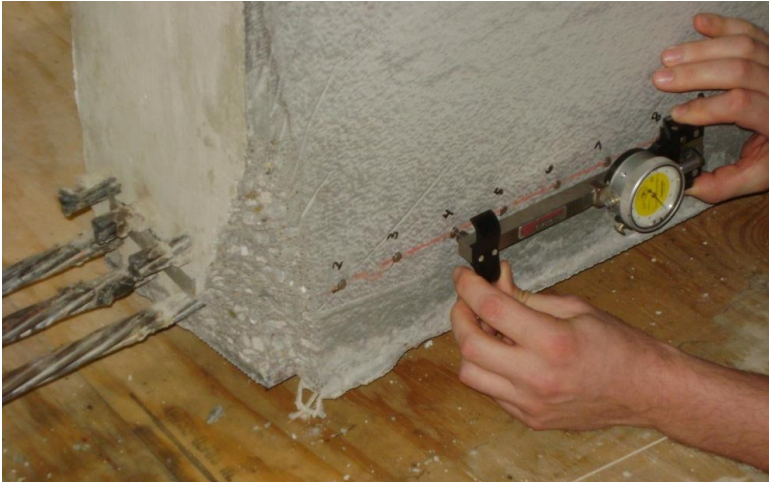
Figure 2.7 Measuring strain in concrete for transfer length estimation
