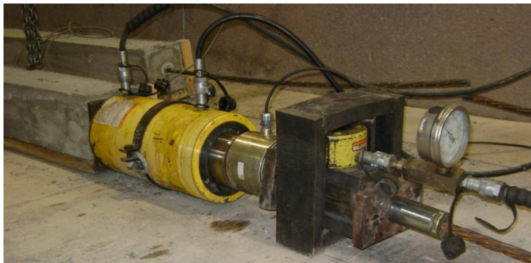
Figure 3.8 Pull-out testing setup
