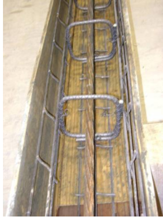
Figure 3.7 Specimen strand confinement
