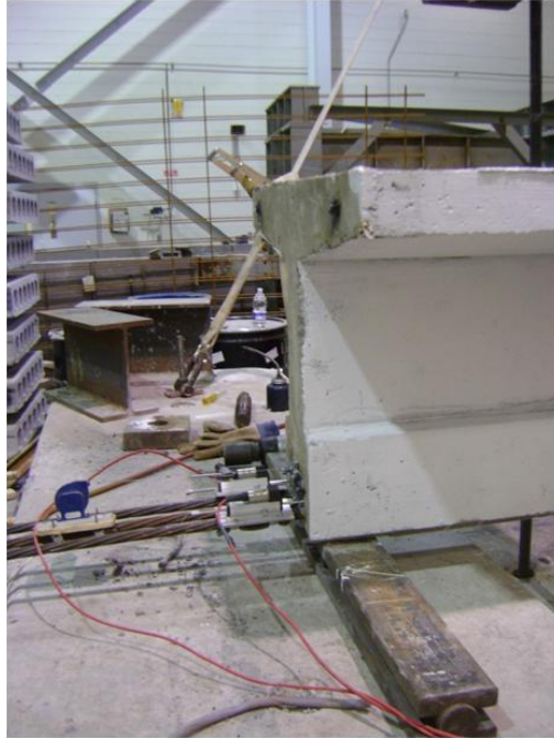
Figure 4.11 Shear test strand instrumentation
