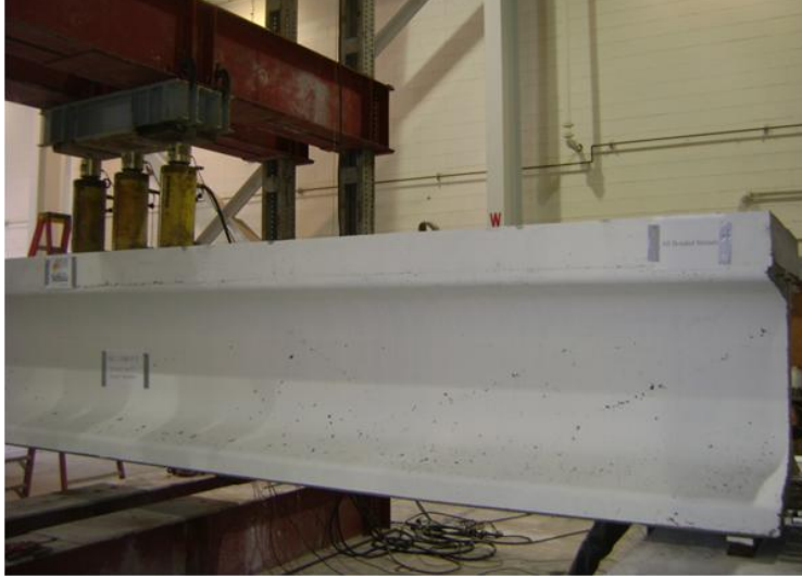
Figure 3.18 NU1100 development length test setup
