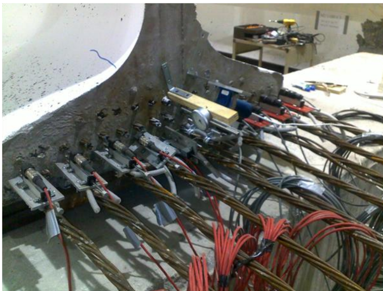
Figure 3.19 Development length test strand instrumentation
