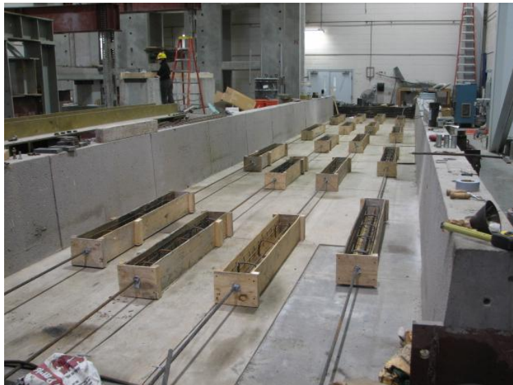
Figure 3.6 Forms of the pullout specimens
