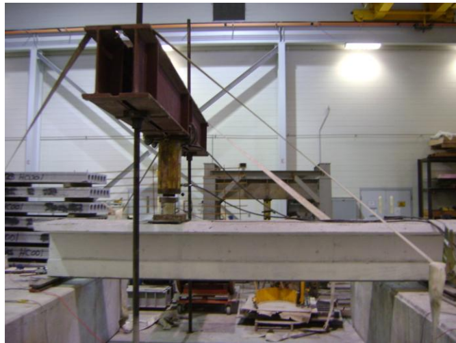
Figure 4.10 Vertical shear test setup
